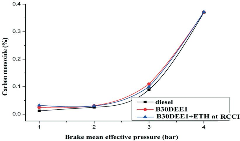
Fig. 5. Carbon monoxide emission versus BMEP
