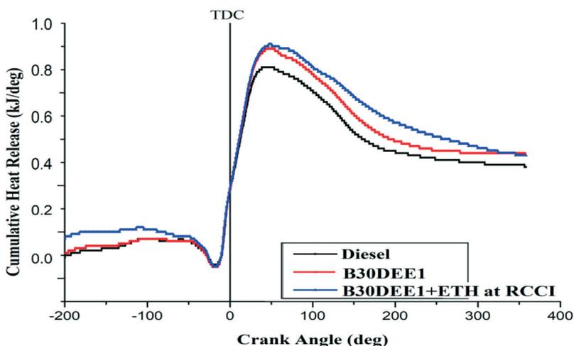
Fig. 12. Cumulative heat release versus crank angle
