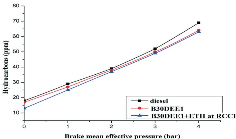
Fig. 6. Hydrocarbon emission versus BMEP
