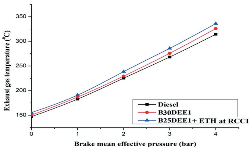
Fig. 4. Exhaust gas temperature with BMEP
