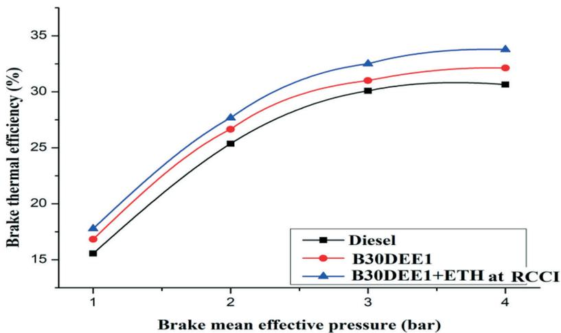
Fig. 3. Variance in brake thermal efficiency along BMEP
