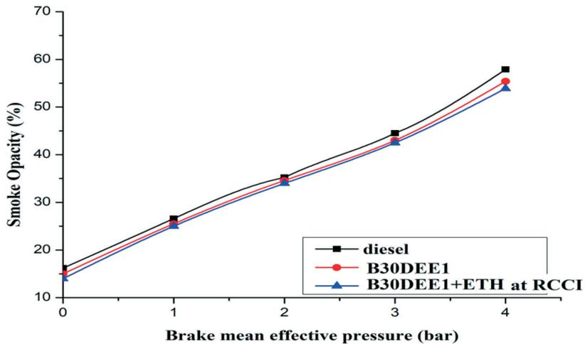
Fig. 8. Smoke Opacity versus BMEP
