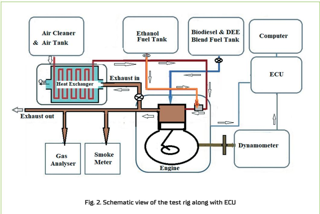
Fig. 2. Schematic view of the test rig along with ECU
