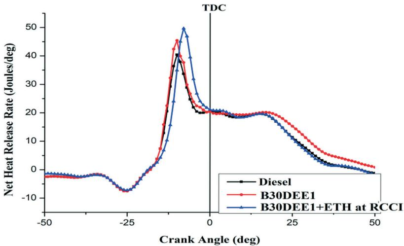
Fig. 10. Net heat release rate versus crank angle
