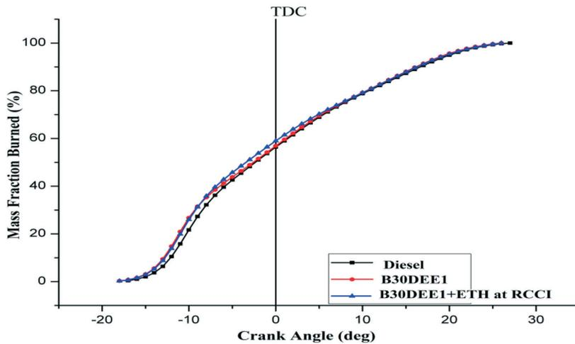
Fig. 11. Mass fraction of the fuel burned versus crank angle
