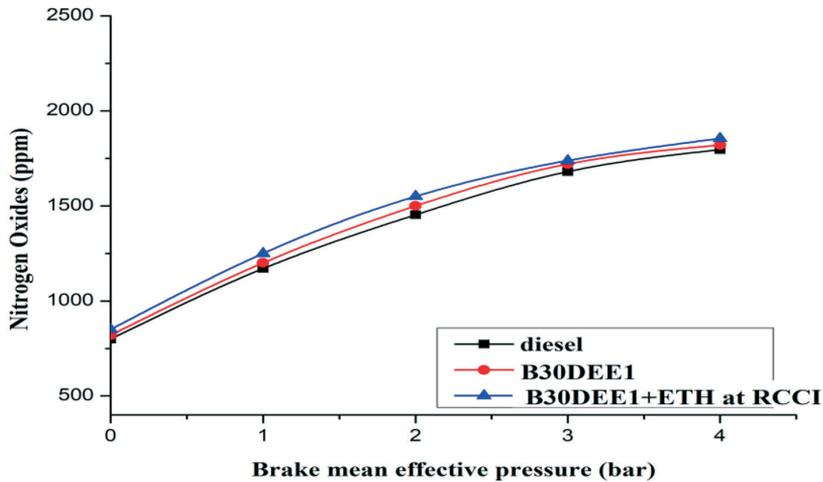
Fig. 7. Nitrogen oxide emission versus BMEP
