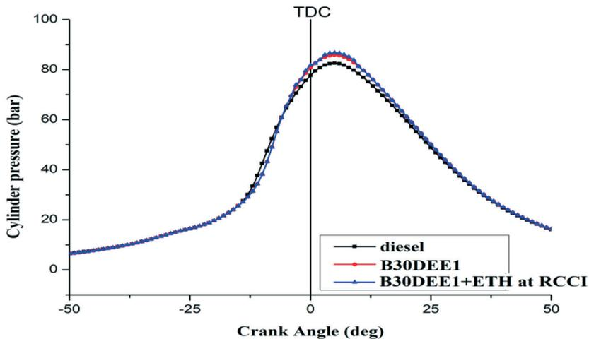
Fig. 9. Cylinder pressure versus crank angle
