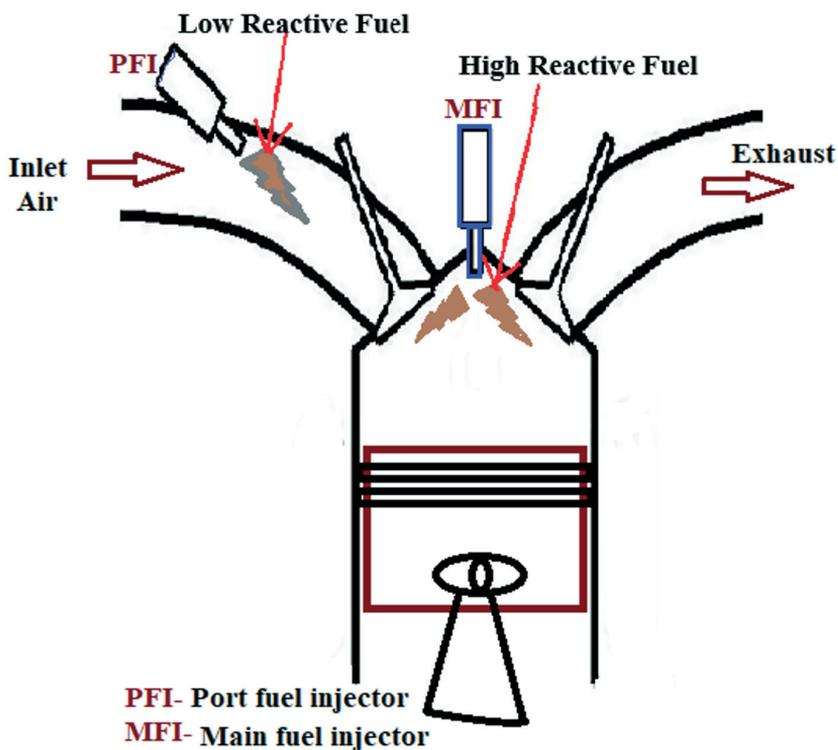
Fig. 1. Schematic diagram for RCCI enabled engine
