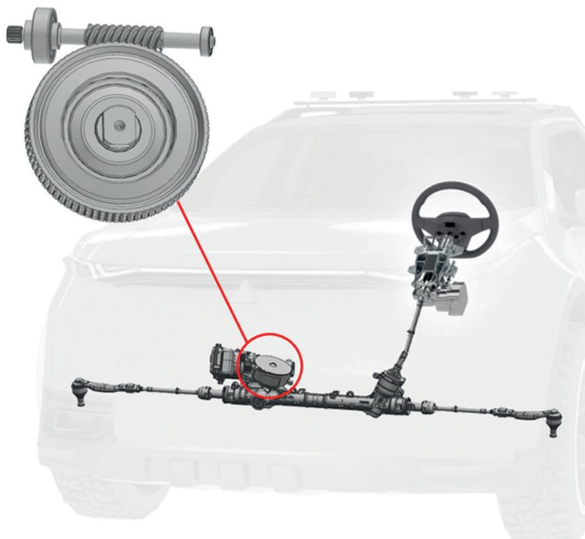
**Fig. 1. View of worm gearing in the EPS system**
