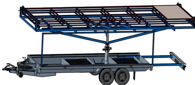
Fig. 2. CAD model of the mobile hybrid renewable energy system showing trailer platform, dual-axis tracking frame, and integrated wind turbines
