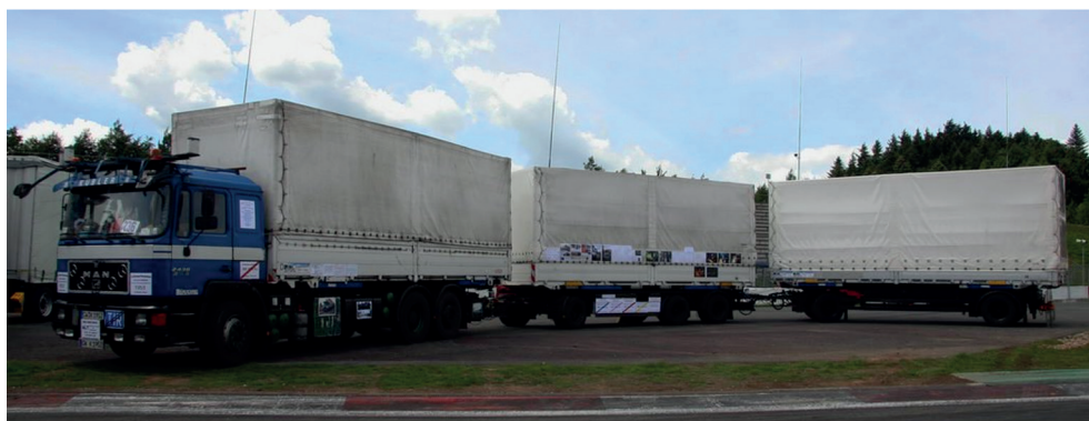
Fig. 1. Three-link road train
