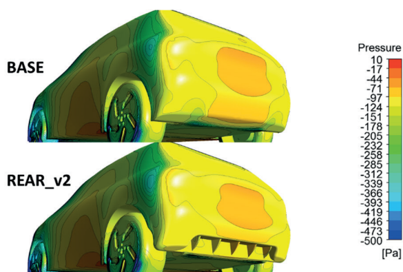
Fig. 24. Pressure colour map comparison for BASE geometry and REAR_v2 modification [Created by the authors]
