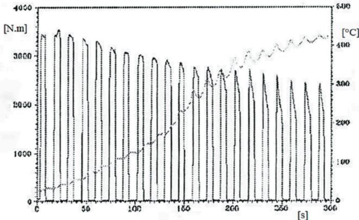
**Fig. 8 Interrupted braking to constant speed (time dependence of braking moment and temperature of lining)**
