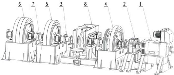
Fig.3. Flywheel braking test stand (1 – electromotor, 2 – gear box, 3 – clutch, 4, 5, 6 – flywheels, 7 – frame, 8 – exchange module for different types of brakes)
