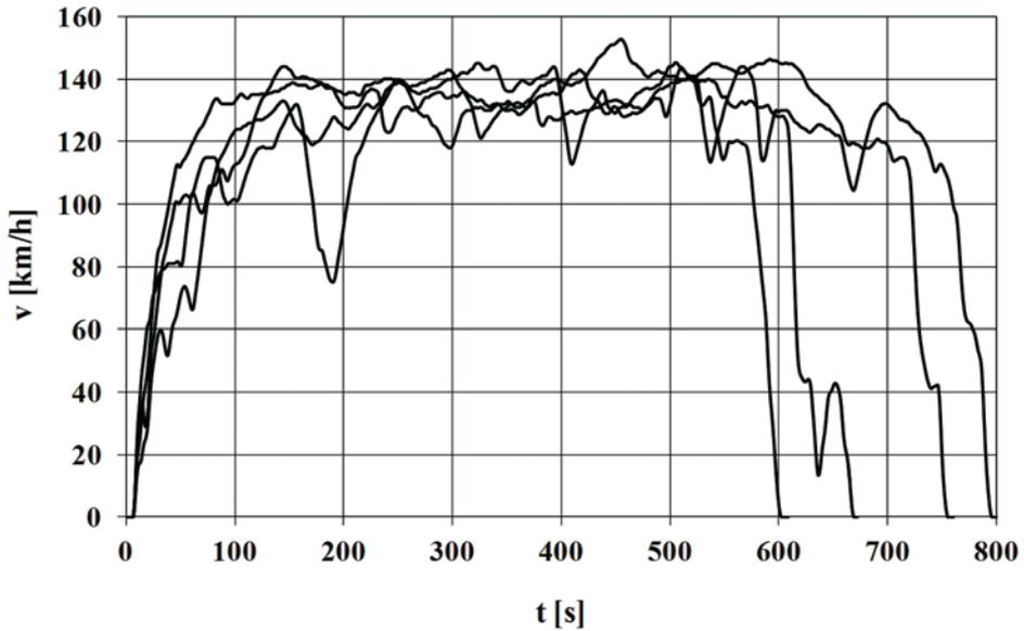
Fig. 17. Selected time histories of the vehicle speed for drives in high-speed traffic
