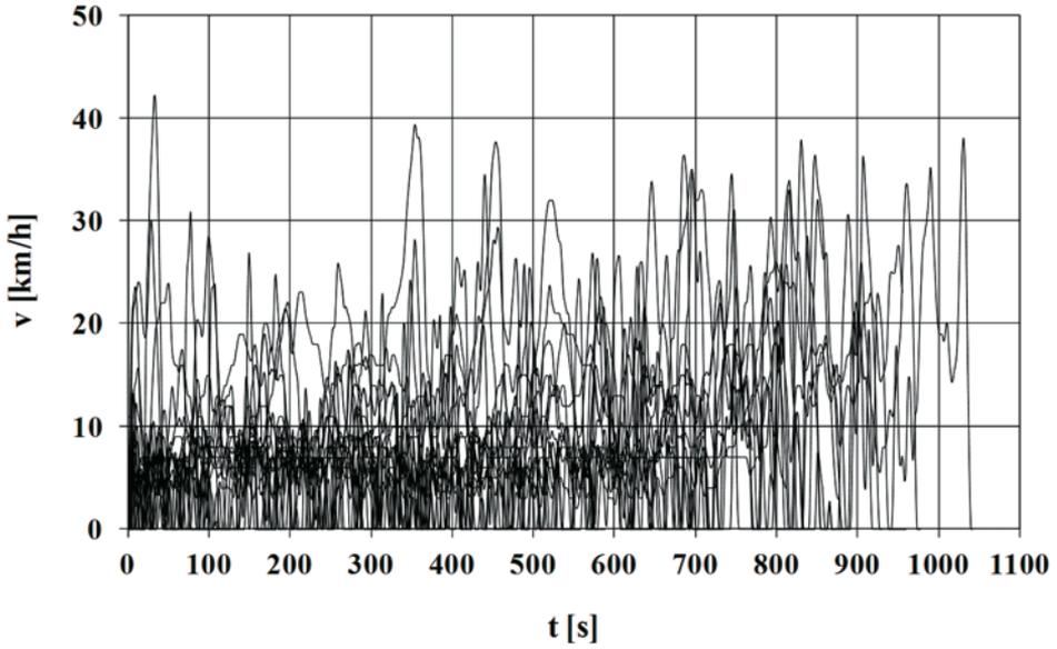
Fig. 2. Time histories of the vehicle speed recorded during test drives in urban traffic congestions
