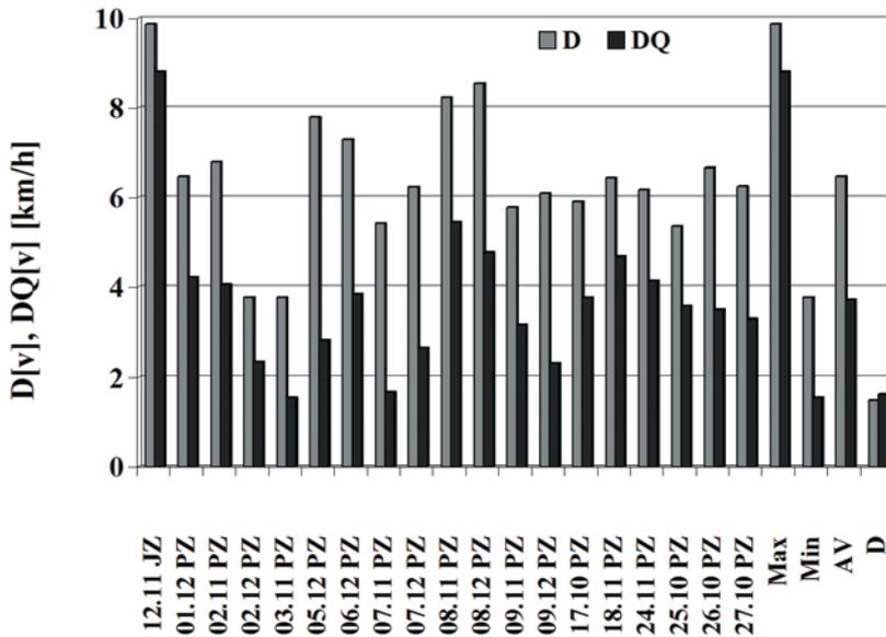
Fig. 10. Standard deviation and quartile deviation of the vehicle speed recorded during test drives in urban traffic congestions
