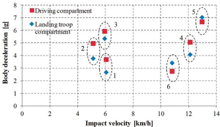
Fig. 4. The distribution of maximum body deceleration
