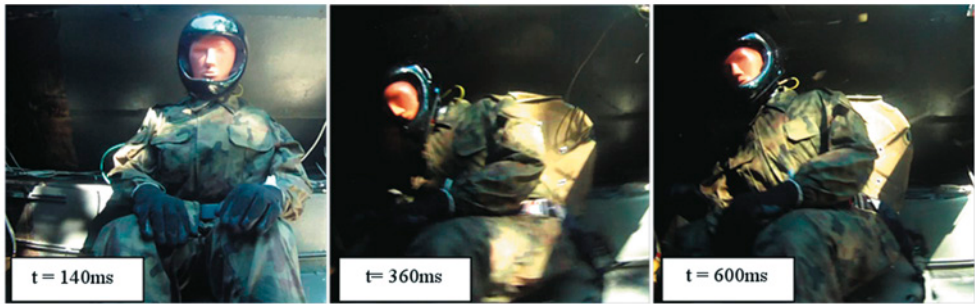
Fig. 8. Phases of motion of the dummy located in the landing troop compartment (trial no. 5)
