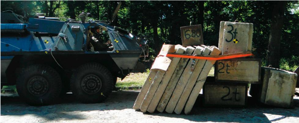
**Fig. 5. The concrete obstacle after collision ( $v = 12,10$  km/h)**
