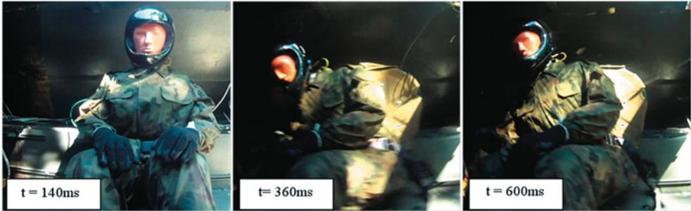
**Fig. 8. Phases of motion of the dummy located in the landing troop compartment (trial no. 5)**
