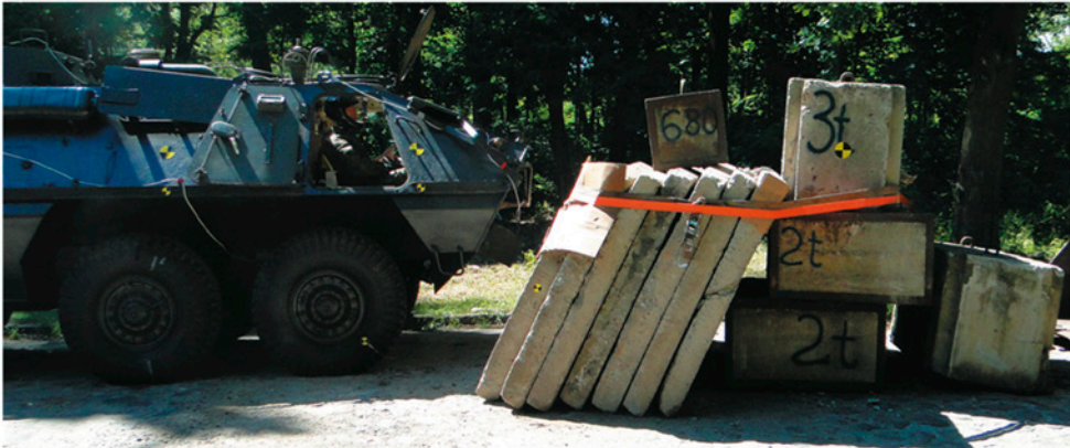
Fig. 5. The concrete obstacle after collision ( v = 12,10 km/h)
