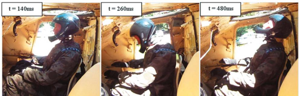
Fig. 7. Phases of motion of the dummy located in the driver's compartment (trial no. 5)
