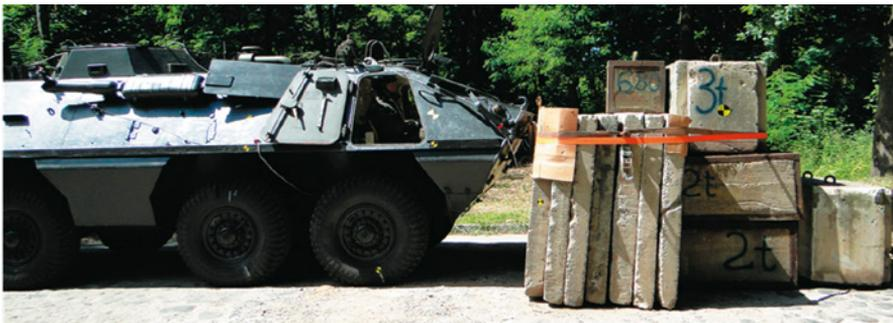
Fig. 1. APC SKOT and concrete obstacle before test
