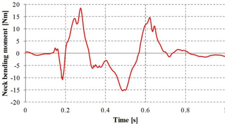
**Fig. 9. The course of the neck bending moment for a dummy located in the driver's compartment (trial no. 5)**
