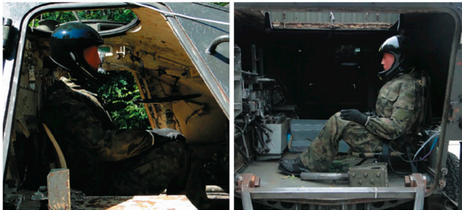
Fig. 2. A dummy located in the driver compartment (left) and in the landing troop compartment (right)
