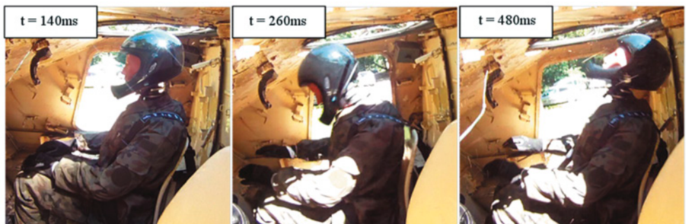
Fig. 7. Phases of motion of the dummy located in the driver's compartment (trial no. 5)
