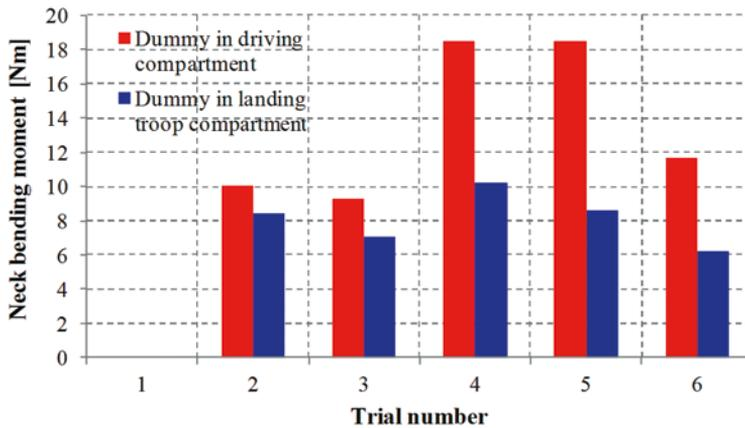
Fig. 10. The maximum values of neck bending moment
