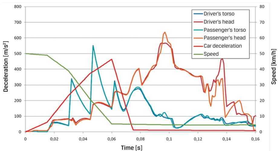
Fig. 4. Deceleration vs. time curves for the driver, passenger, and vehicle (computer model), for a speed of 50 km/h (typically adopted at type-approval tests), according to data obtained from sensors located as specified in the graph
