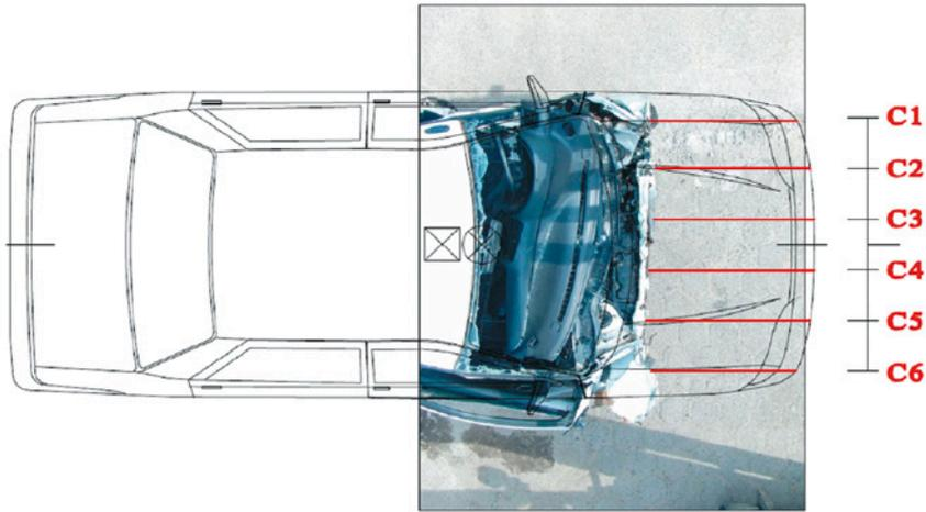
Fig. 3. The places where deformations of the front part of the Suzuki Swift car were measured
