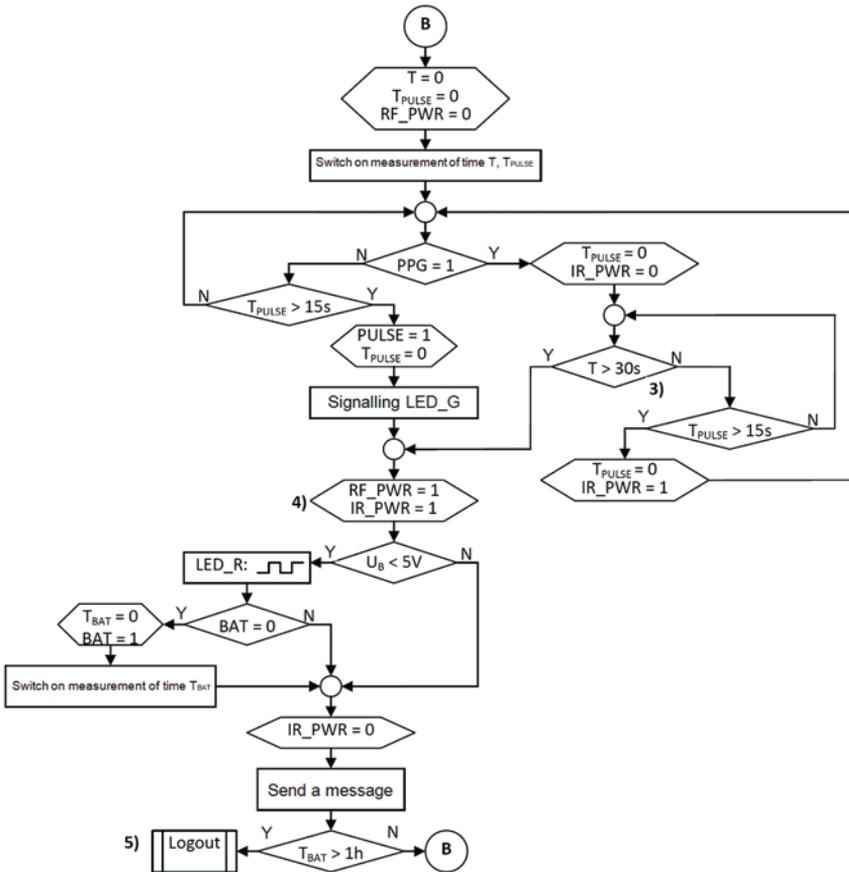
Fig. 6. Algorithm of operation of the pulse sensor [9.4]
