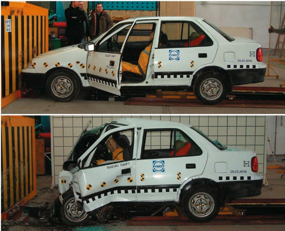
**Fig. 2. The Suzuki Swift car before and after the crash test; the impact speed was about 87 km/h**
