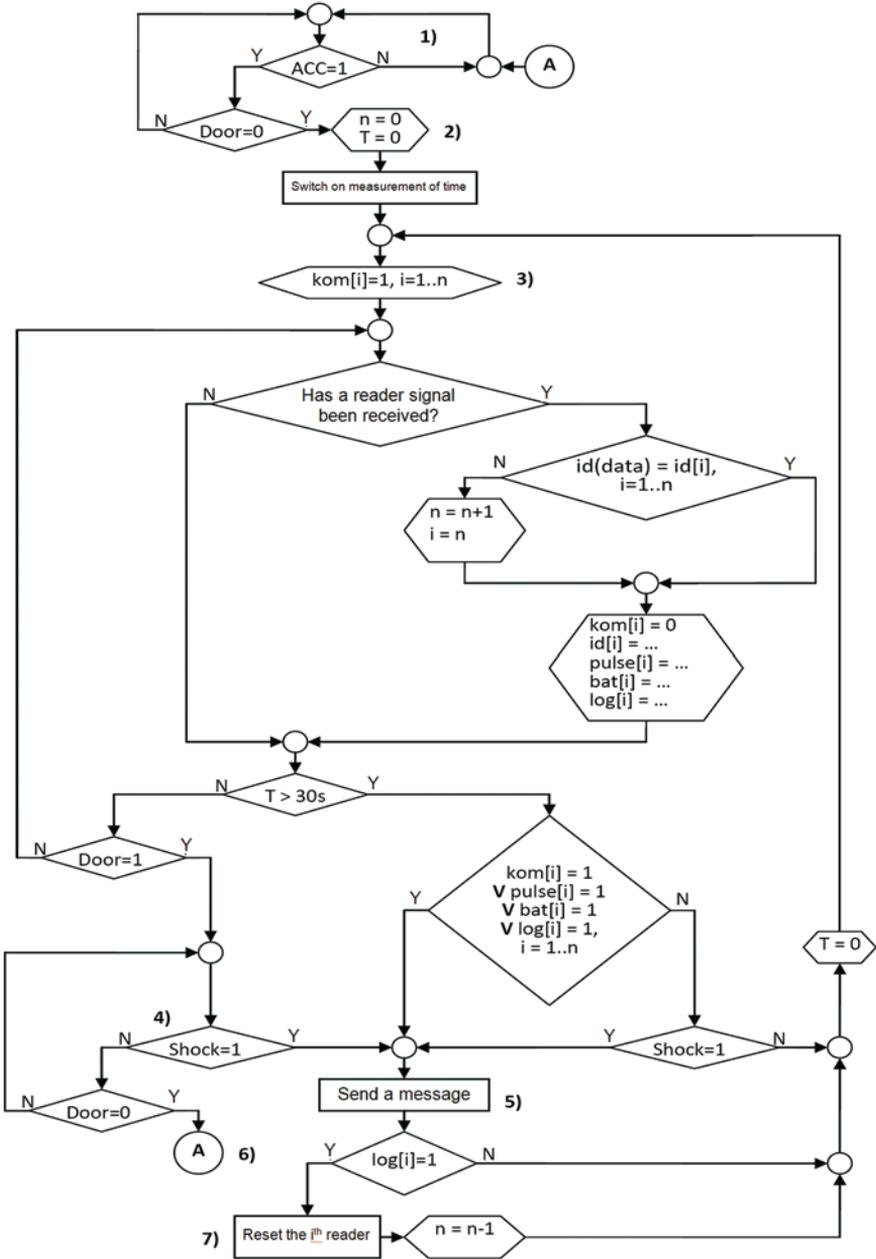
Fig. 7. Algorithm of operation of one of versions of the receiving unit that cooperates with the pulse sensor [9.4]
