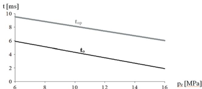
**Fig. 6.** Linearly approximated influence of the oil supply pressure on the valve motion delay and valve opening time:  $t_{op}$  – valve motion delay in relation to the current control signal;  $t_o$  – valve opening time
