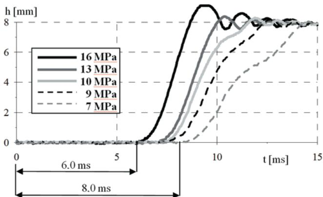
**Fig. 4. Influence of the oil supply pressure on the valve motion delay ( $C = 1\,000\ \mu\text{F}$ )**
