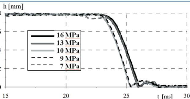
**Fig. 7.** Influence of the oil supply pressure on the valve opening process ( $C = 1\ 000\ \mu\text{F}$ )
