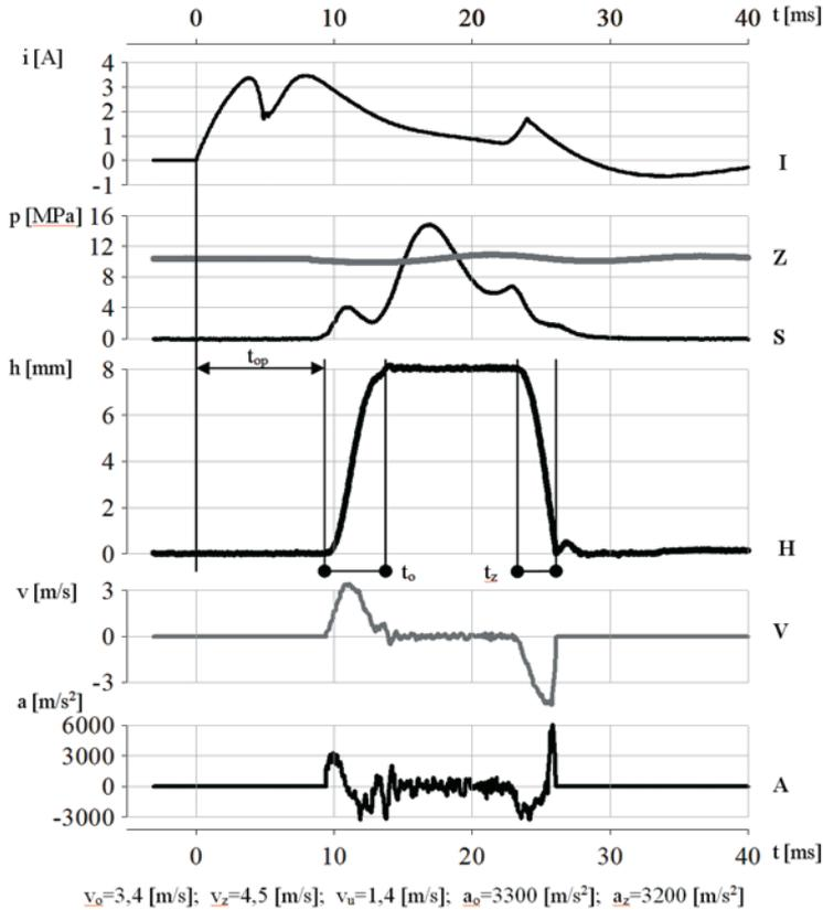
**Fig. 3. Example time histories of current control signal, parameters describing the valve kinematics, and oil pressures recorded during the bench tests**
