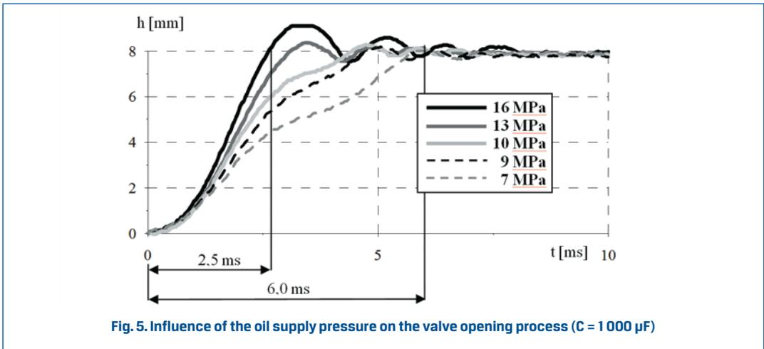
**Fig. 5. Influence of the oil supply pressure on the valve opening process ( $C = 1000 \mu\text{F}$ )**
