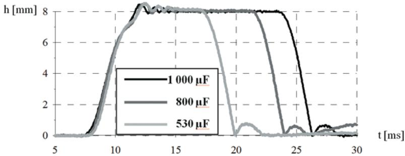
**Fig. 8. Influence of the control signal on the valve displacement vs. time curves ( $p_0 = 10 \text{ MPa}$ )**
