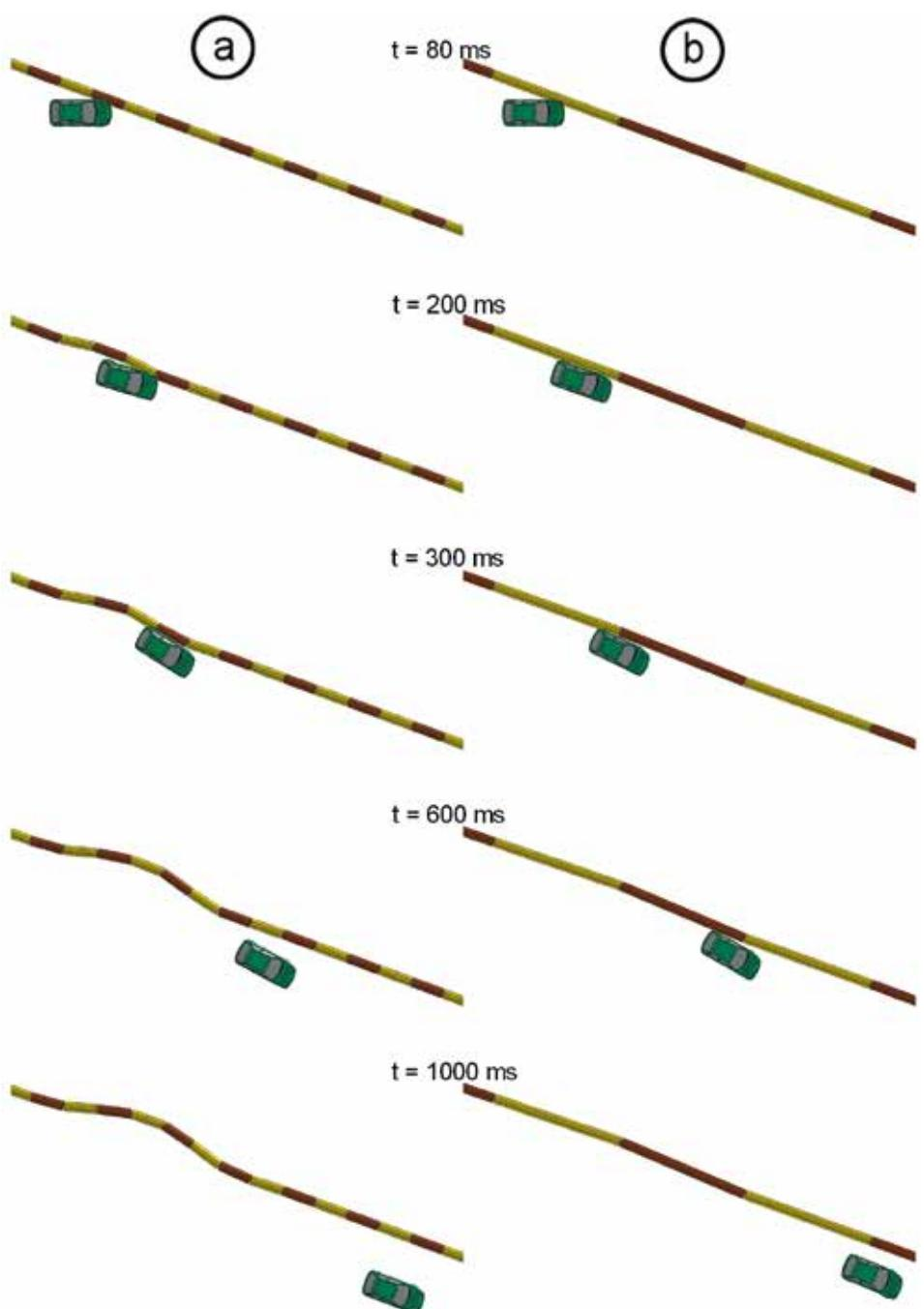
Fig. 8. The course of impact phases (impact point PZB), for  $t = 80, 200, 300, 600$  and  $1000$  ms, for a Suzuki Swift car with a concrete safety barrier composed of segments of various length: a) – 2m segment, b) – 8m segment
