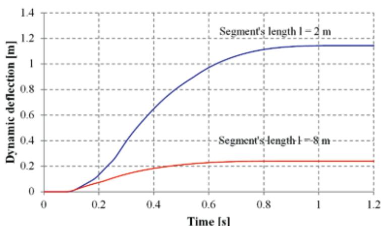
**Fig. 7. Dynamic deflection of the concrete safety barrier for two segment lengths**
