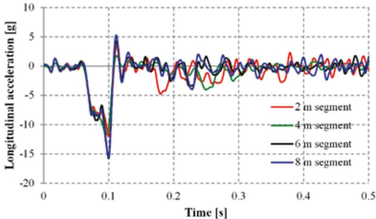
Fig. 3. A course of longitudinal accelerations of the centre of mass of the car in the time function for a concrete barrier composed of 4 m segments with marked out time zones
