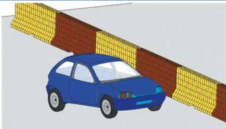
**Fig. 2. Suzuki Swift car model with a concrete barrier [4]**
