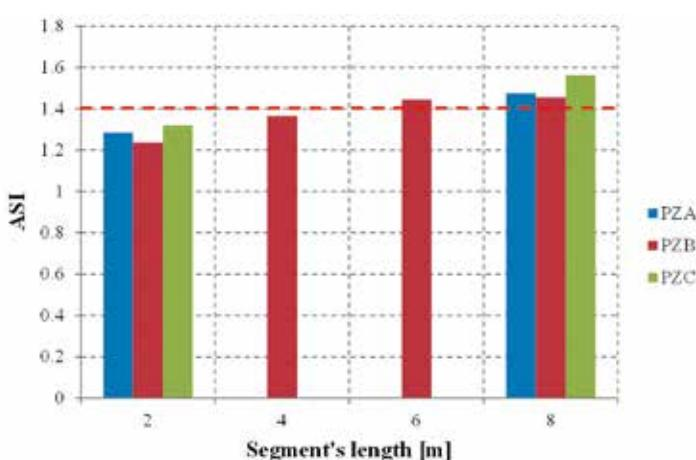
**Fig. 5. The histogram of the ASI index for the barriers composed of segments of various lengths and selected points of impact (PZ)**
