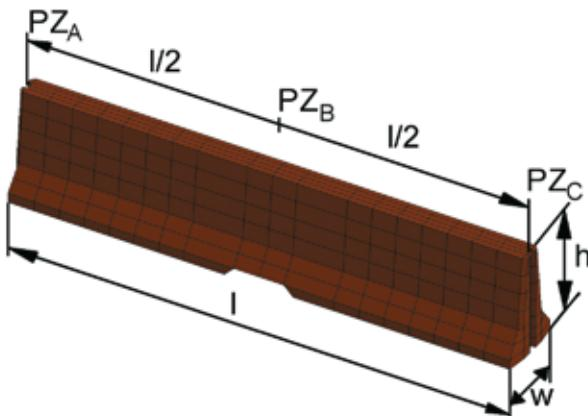
**Fig. 1. Segment of the concrete safety barrier: PZA, B, C – impact point, the beginning, the middle, the end of the segment; l (l/2) – segment length (segment half); h= 810 mm – segment height; w= 550 mm – segment width**
