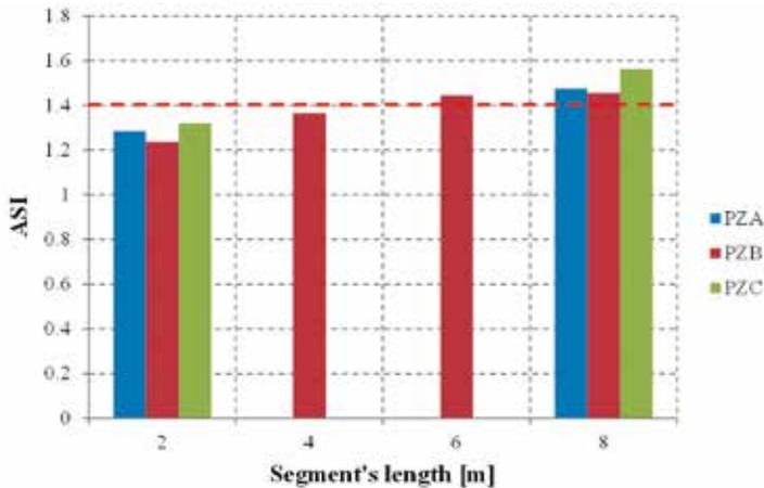
Fig. 5. The histogram of the ASI index for the barriers composed of segments of various lengths and selected points of impact (PZ)
