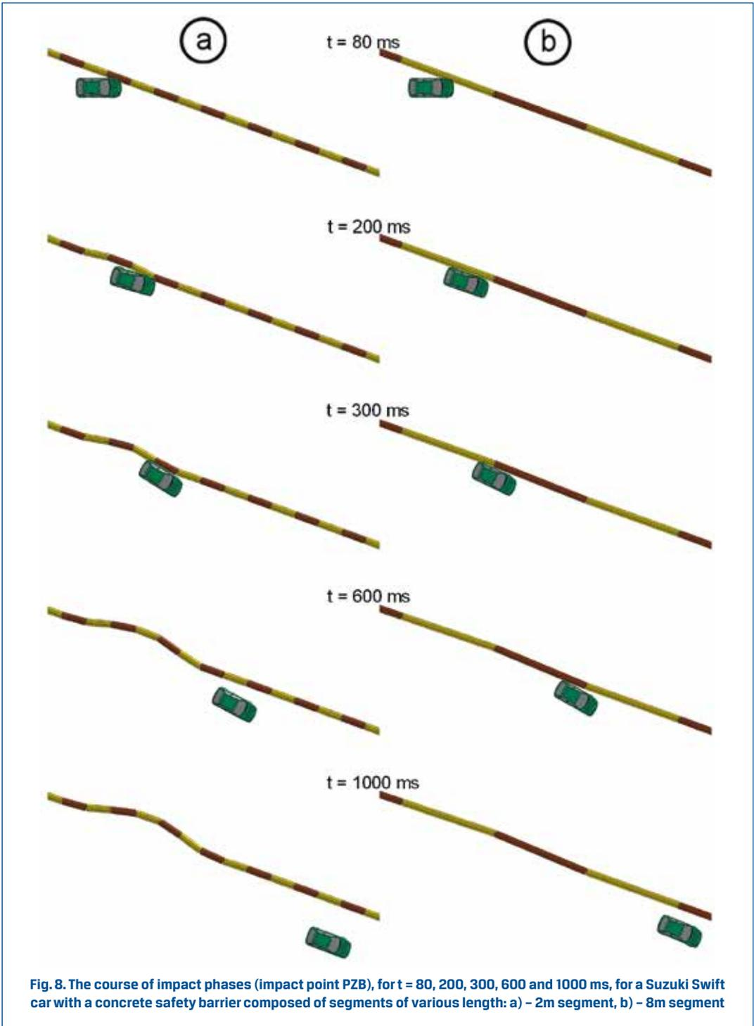
Fig. 8. The course of impact phases (impact point PZB), for  $t = 80, 200, 300, 600$  and  $1000$  ms, for a Suzuki Swift car with a concrete safety barrier composed of segments of various length: a) - 2m segment, b) - 8m segment
