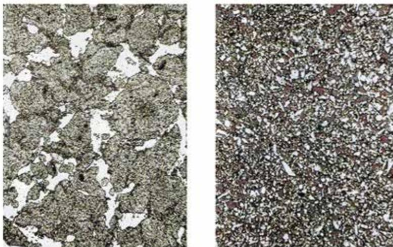
**Fig. 9. Dust of the sample taken from the disc brakes; magnitude  $\times 76$  (right) and  $\times 910$  (left)**
