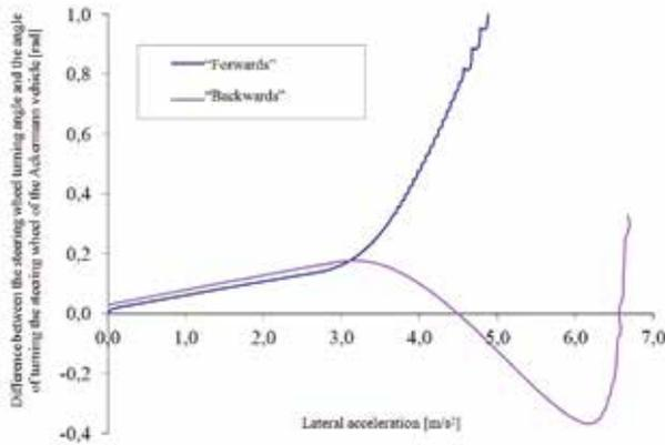
Fig. 11. Steerability curves for the vehicle moving on dry asphalt concrete with a velocity of 40 km/h
