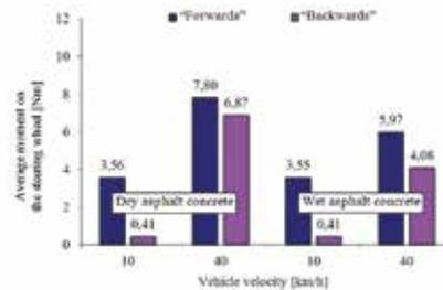
**Fig. 10. Average value of the modulus of the moment of forces on the steering wheel vs. vehicle velocity and road surface type**
