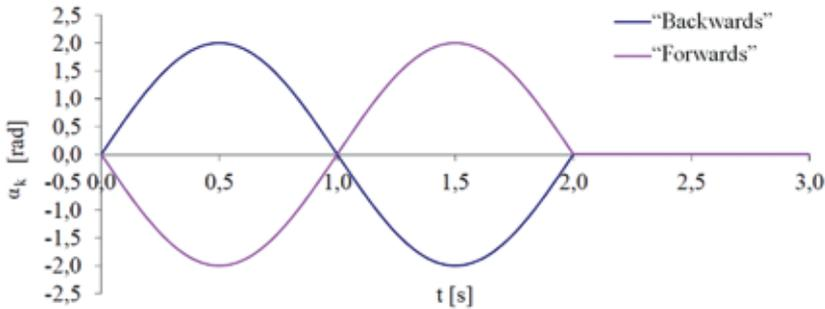
Fig. 5. Input applied to the steering wheel during a single lane-change manoeuvre
