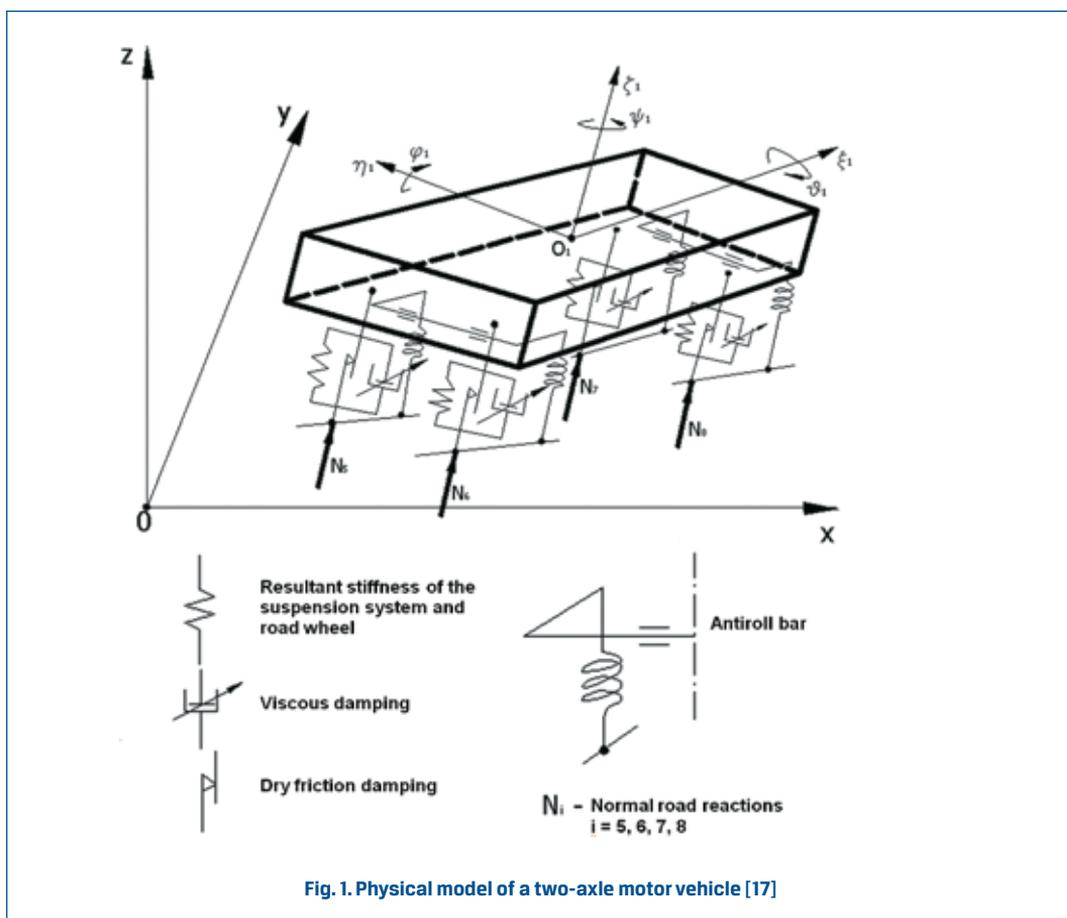
Fig. 1. Physical model of a two-axle motor vehicle [17]
