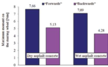
Fig. 19. Maximum moment of forces on the steering wheel during the manoeuvre
