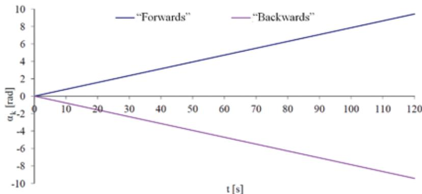
Fig. 3. Time history of the input (turning angle) applied to the steering wheel
