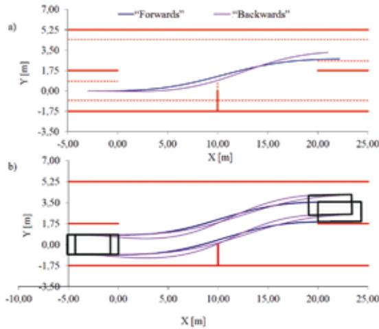
**Fig. 14. Trajectories of characteristic points of the vehicle driven on dry asphalt concrete, with the initial vehicle position for the movement "backwards" having been adjusted: a) centre of vehicle mass; b) vertices of the vehicle contour**
