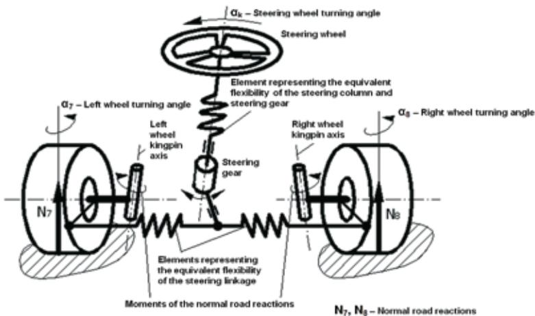
Fig. 2. Model of a motor vehicle steering system with a parallel structure [17, 18]
