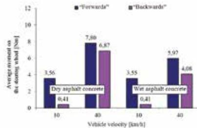
**Fig. 10. Average value of the modulus of the moment of forces on the steering wheel vs. vehicle velocity and road surface type**
