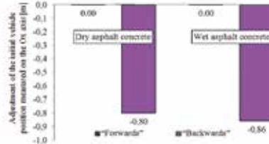
Fig. 16. Adjustment of the initial position of the vehicle centre of mass in the Ox direction, necessary for the manoeuvre to be successful
