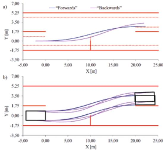
**Fig. 13. Trajectories of characteristic points of the vehicle driven on dry asphalt concrete: a) centre of vehicle mass; b) vertices of the vehicle contour**
