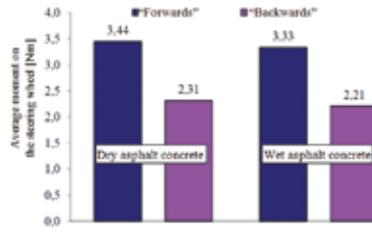
Fig. 20. Average moment of forces on the steering wheel during the manoeuvre
