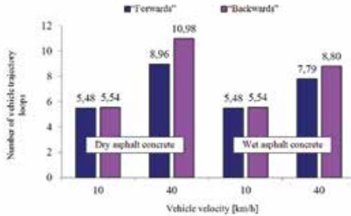
**Fig. 8. Number of vehicle trajectory loops vs. vehicle velocity and road surface type**
