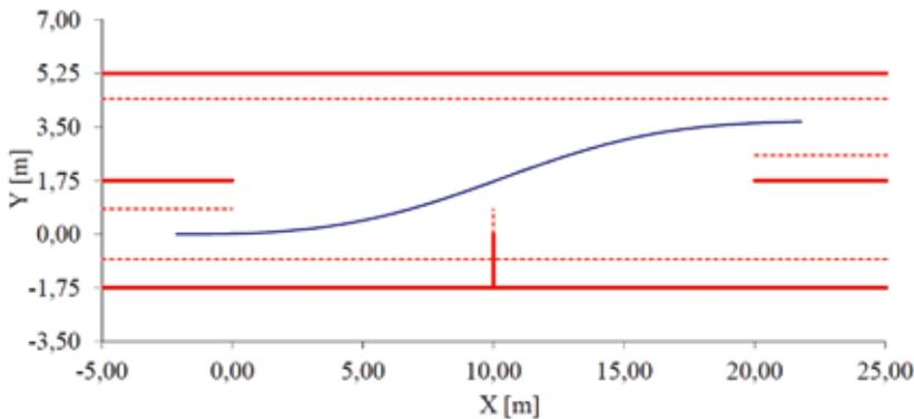
**Fig. 4. The prescribed "corridor" of vehicle motion during a single lane-change manoeuvre, with an example trajectory of the centre of vehicle mass  $O_1$**
