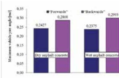
Fig. 17. Maximum vehicle body yaw angle during the manoeuvre
