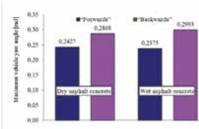
Fig. 17. Maximum vehicle body yaw angle during the manoeuvre
