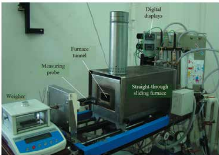
Fig. 2.1. General view of the test stand for gravimetric investigations of the PM oxidation kinetics [16]
