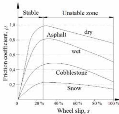
Fig.6. Wheel slip – friction characteristic on different road pavement
