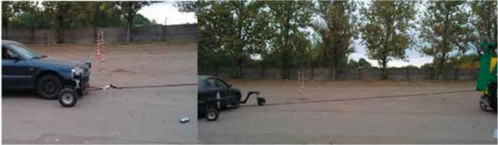
**Fig. 4. Pull experiment for evaluation of longitudinal and lateral friction**
