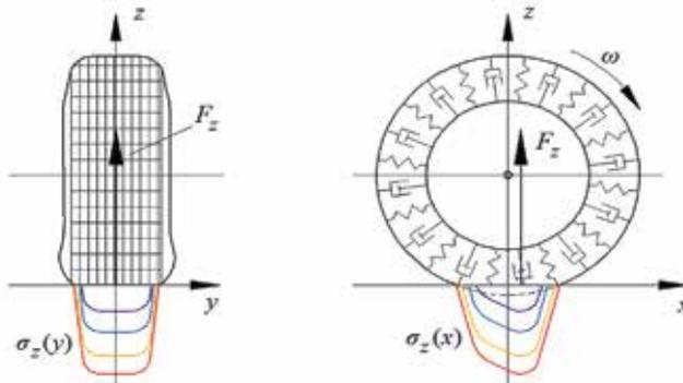
Fig. 3. Normal stress distribution in rolling tire contact area in different vertical load modes
