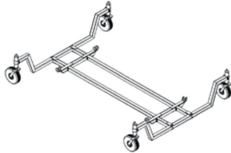
**Fig. 2. Construction of skidcar system**
