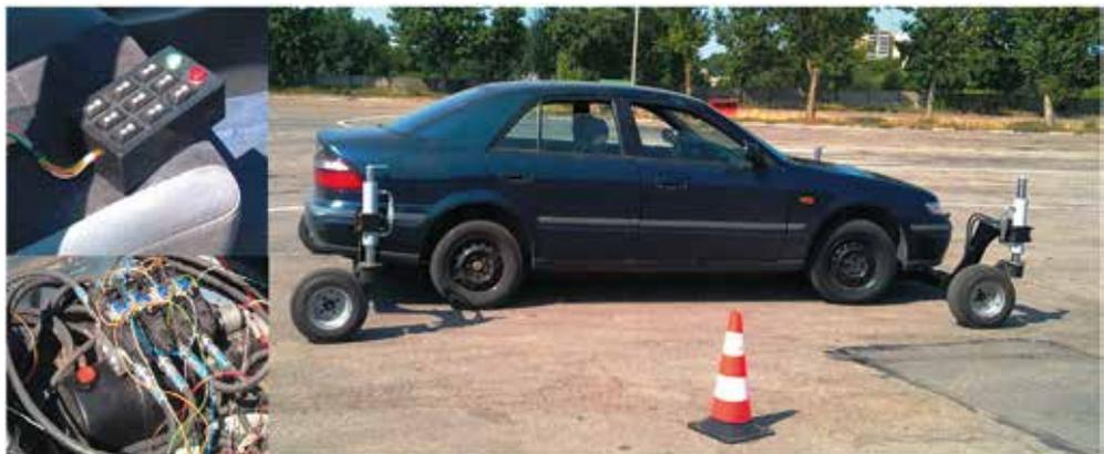
**Fig. 1. Vehicle equipped with skidcar system and system control panel with 12V hydraulic power pack**
