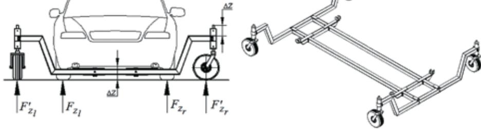
**Fig. 2. Construction of skidcar system**
