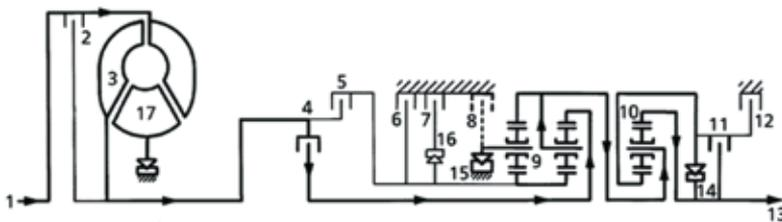
**Fig. 7. Schematic diagram of power flow for the transmission operating in gear "1". Drive mode selector lever set to D/1 [17, 20]**
