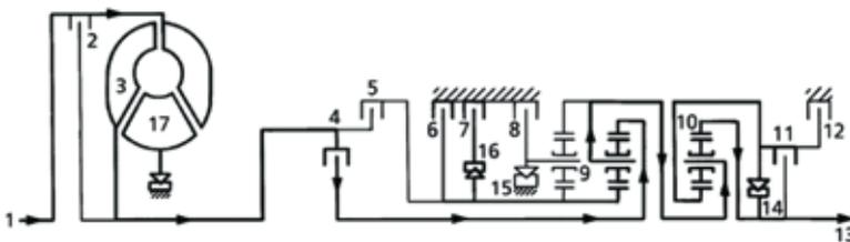
**Fig. 8. Schematic diagram of power flow for the transmission operating in gear "2". Drive mode selector lever set to D/2 [17, 20]**
