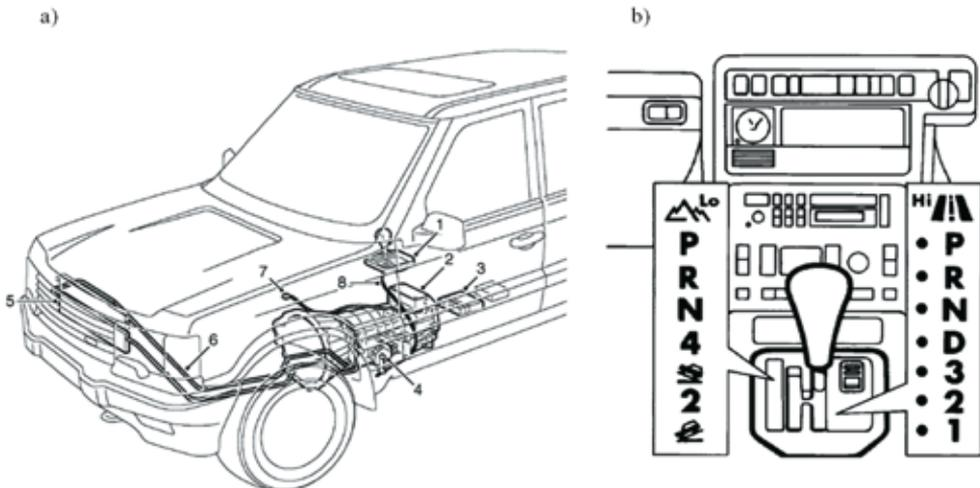
**Fig. 1. The ZF-4HP24 automatic transmission system: a) automatic transmission component layout; b) drive mode selector lever assembly with an "H gate" mechanism [17];**
