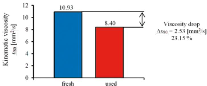
**Fig. 13. Kinematic viscosity  $v_{D80}$  of ATF DEXRON IID/III samples taken from the transmission of a vehicle that had travelled  $S_p = 148\,345$  km in total ("used" fluid) and of fresh ATF ("fresh" fluid)**
