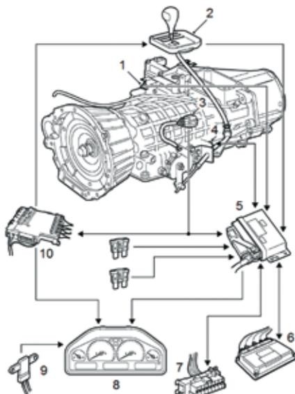
**Fig. 3. Schematic diagram of the electronic system of the ZF-4HP24 automatic transmission:**
