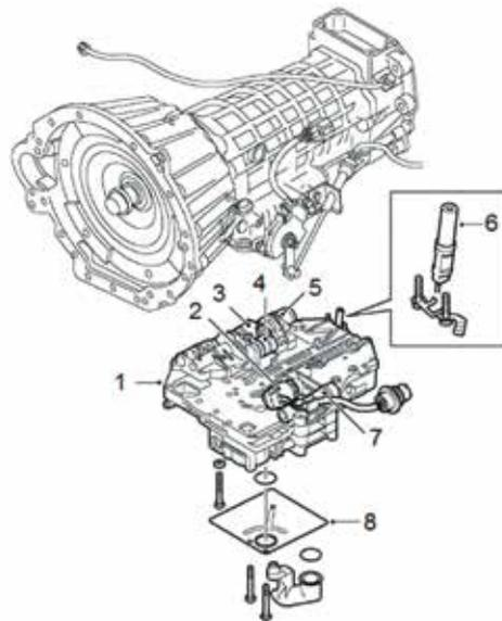
**Fig. 4. Electrohydraulic controller: 1 – valve block; 2 – pressure-regulating solenoid valve (MV 4); 3, 4 – gear-shift control solenoid valves (MV 2 and MV 1, respectively); 5 – lock-up clutch control solenoid valve (MV 3); 6 – output shaft speed sensor; 7 – manual control valve; 8 – suction filter of the hydraulic system [17]**
