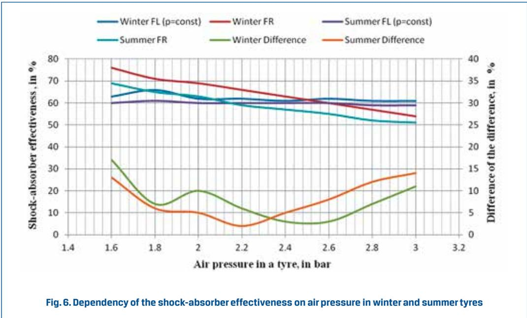
Fig. 6. Dependency of the shock-absorber effectiveness on air pressure in winter and summer tyres
