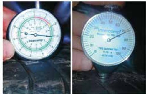
**Fig. 4. Summer tyre tread depth and rubber hardness**
