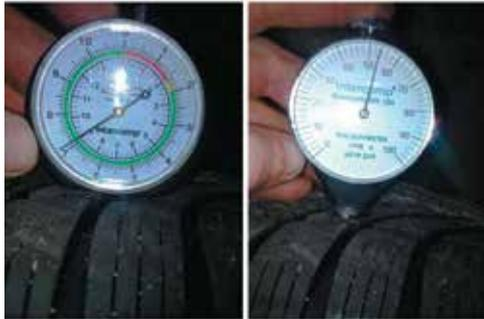
**Fig. 3. Winter tyre tread depth and rubber hardness**
