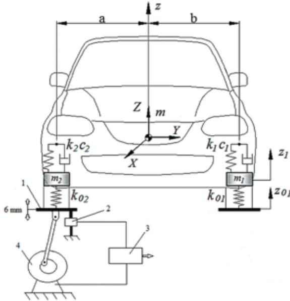
**Fig. 1. A half-car model for dynamic analysis and principal mode of EUSAMA method (on the left side):**
