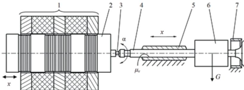
**Fig. 3. The model of the assembly consisted of movable coil the drive and valve bearing in its guide and loaded by additional weight; 1 - immovable part of the drive, 2 - movable coil, 3 - spherical joint, 4 - valve, 5 - guide, 6 - additional weight, 7 - seat insert**
