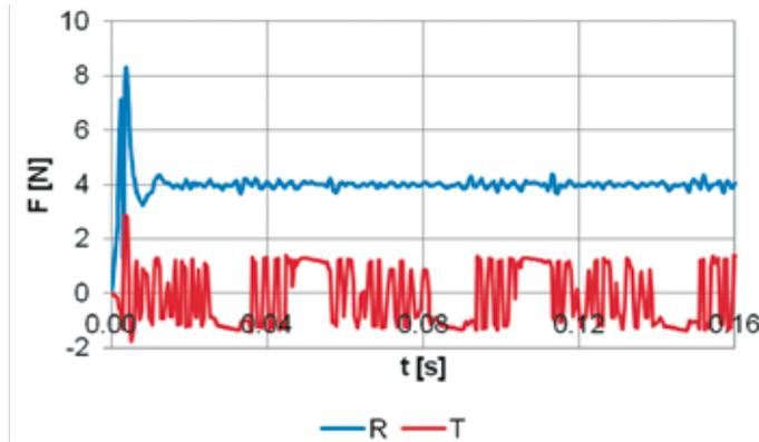
**Fig. 10.** Values of friction force  $T$  and of normal force  $R$  against time  $t$ , obtained during simulations; loading frequency  $f = 16$  Hz, valve stroke  $h_{max} = 5$  mm
