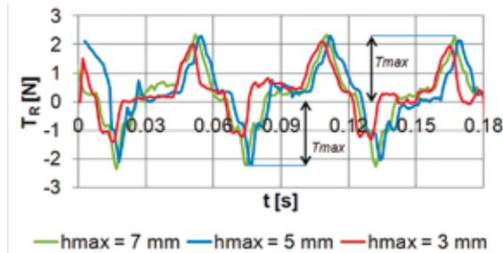
**Fig. 7. Measured values of the friction force  $T_R$  between valve and its guide against time  $t$ ; loading frequency  $f = 16$  Hz, valve stroke  $h_{max} = 7$  mm,  $h_{max} = 5$  mm and  $h_{max} = 3$  mm, respectively,  $T_{max}$  - maximum friction force during valve displacement against its guide**
