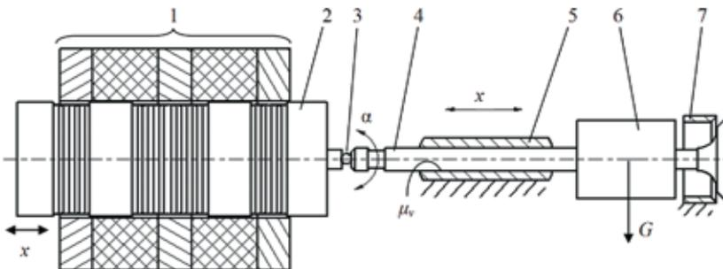
**Fig. 3. The model of the assembly consisting of movable coil the drive and valve bearing in its guide and loaded by additional weight; 1 - immovable part of the drive, 2 - movable coil, 3 - spherical joint, 4 - valve, 5 - guide, 6 - additional weight, 7 - seat insert**
