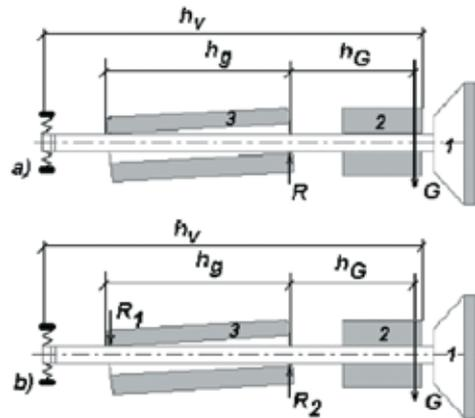
**Fig. 2. The scheme of loading for the valve - added mass - guide assembly; 1 - valve, 2 - added mass, 3 - guide; a) loading case, when reaction R between valve stem and its guide has existed in only one place, b) loading case, when reactions R1 and R2 between valve stem and its guide have existed in two places**
