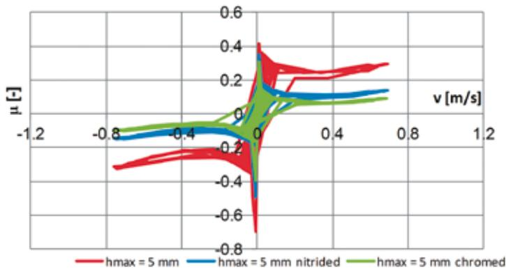
**Fig. 12. Values of friction coefficient  $\mu$  against sliding velocity  $v$ ; loading frequency  $f = 16$  Hz, valve stroke  $h_{max} = 5$  mm, without protective layer, nitrided and chromed**
