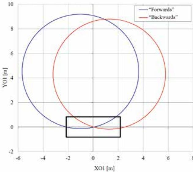
**Fig. 2. Trajectory of the centre of vehicle mass at a constant value of the steering wheel turning angle**
