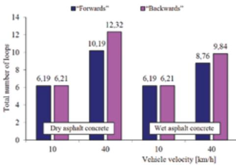
**Fig. 11. Total number of vehicle trajectory loops vs. vehicle velocity and road surface type**
