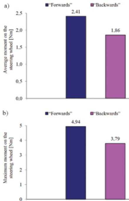
Fig. 21. Average (a) and maximum (b) moment applied to the steering wheel during the parking manoeuvre
