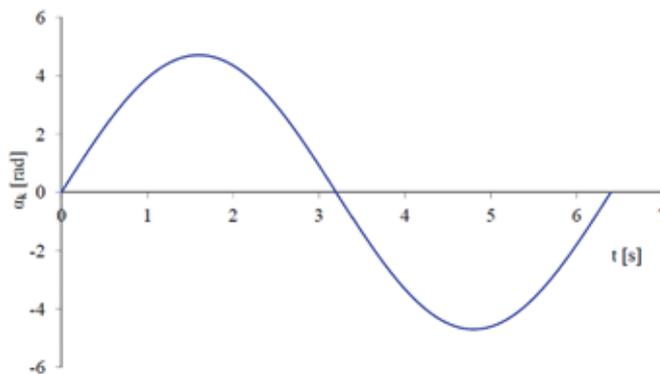
**Fig. 18. Manoeuvre 3. Time history of the steering wheel input during the "forward" movement, with the parameters (period and amplitude) of this input having been modified**
