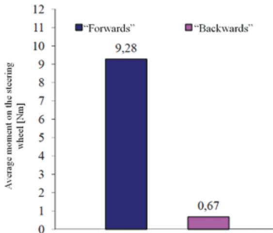
Fig. 4. Average absolute values of the moments on the steering wheel of the vehicle driven along a path with a constant curvature radius
