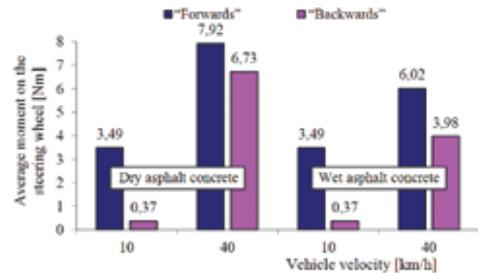
**Fig. 14. Average absolute values of the moment on the steering wheel vs. vehicle velocity and road surface type**
