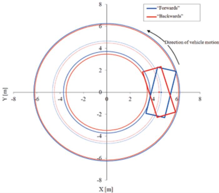
Fig. 3. Trajectory of the centre of vehicle mass at a constant value of the steering wheel turning angle, after changes in the initial vehicle position
