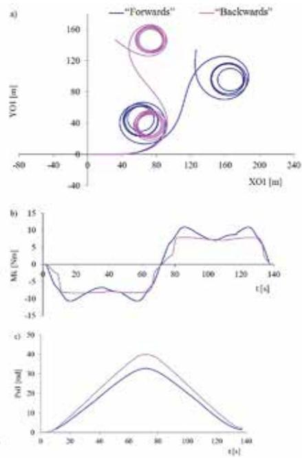
**Fig. 8. Vehicle driven with a speed of 40 km/h on dry asphalt concrete:**
