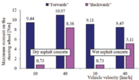
**Fig. 13. Maximum absolute values of the moment on the steering wheel vs. vehicle velocity and road surface type**
