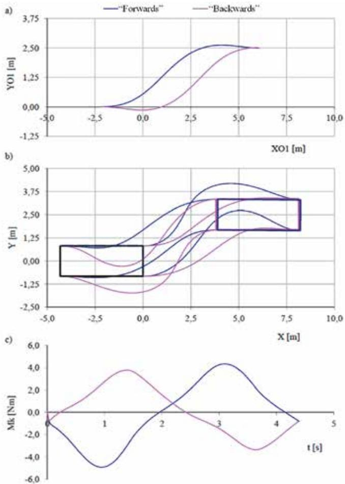
Fig. 16. Trajectory of the centre of vehicle mass (a), trajectory of the vehicle contour (b), and time history of the moment on the steering wheel (c)
