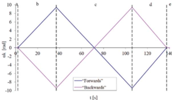
Fig. 6. Time history of the "saw-tooth" steering wheel input; individual stages of the manoeuvre have been shown
