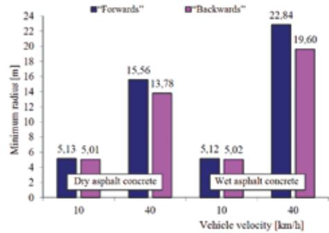
**Fig. 12. Radius of the smallest vehicle trajectory loop vs. vehicle velocity and road surface type**
