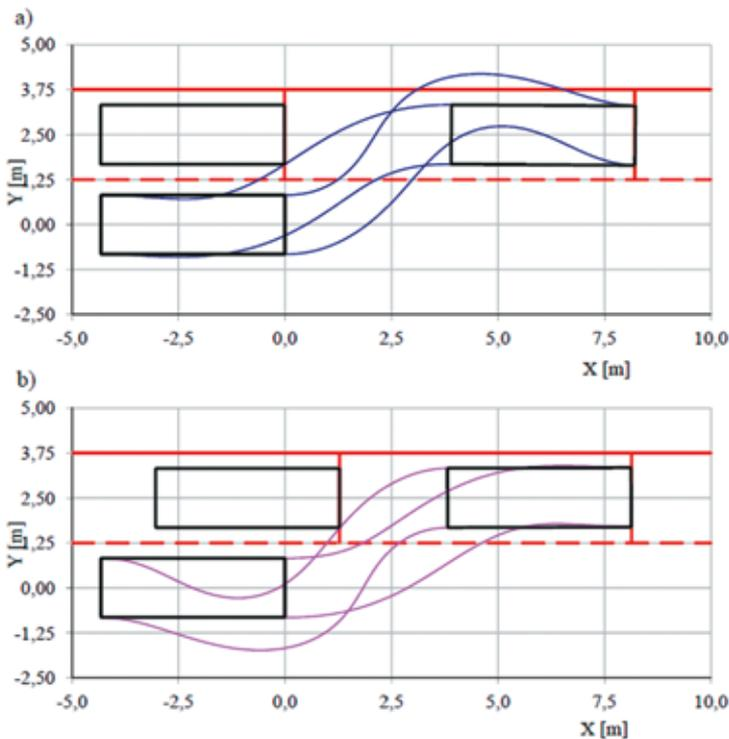
**Fig. 17. Trajectory of the vehicle contour: a) for the vehicle moving "forwards"; b) for the vehicle moving "backwards"**
