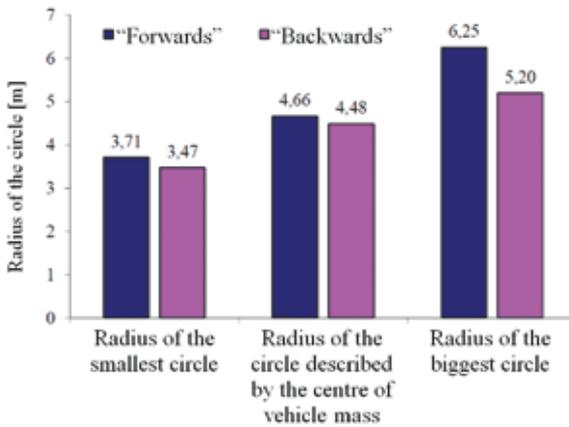
Fig. 5. Radii of the circles described by the vehicle driven "forwards" and "backwards"
