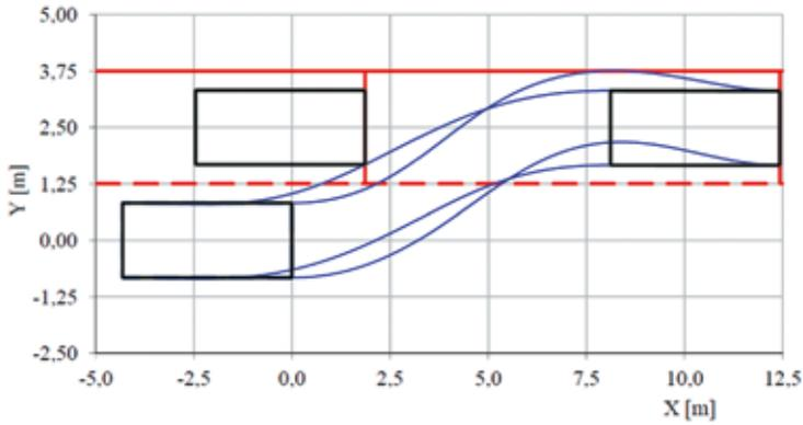
Fig. 19. Trajectory of the vehicle contour for the vehicle moving "forwards" after modification of the steering wheel input
