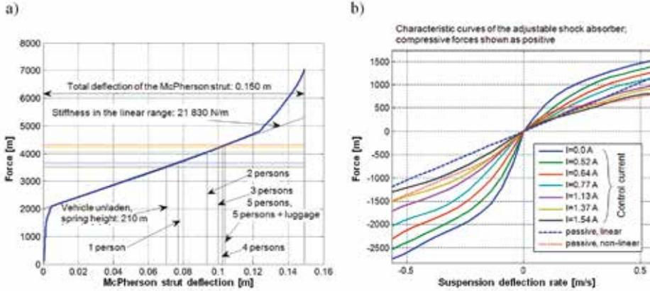
**Fig. 7. Characteristic curves of components of the model of the passive quarter-car suspension system: a) spring, with loads specified; b) semi-active and passive shock absorber**
