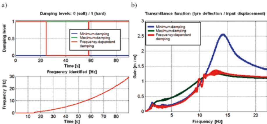
**Fig. 8. Effect of switching-over the damping level according to the input frequency; comparison with the suspension performance curves plotted for the suspension system with the damping having been set to the minimum and maximum levels of the shock absorber performance range: a) changes in the damping level; b) tyre deflection gain curves**
