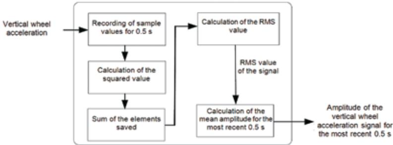
**Fig. 5. Schematic diagram of the algorithm of real-time amplitude detection**
