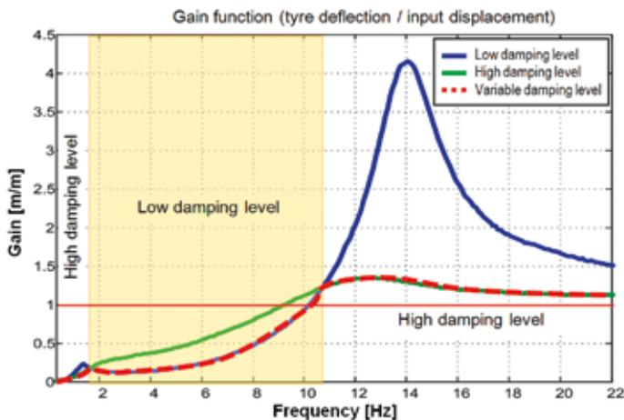
Fig. 2. The idea of changing the damping level according to the input frequency
