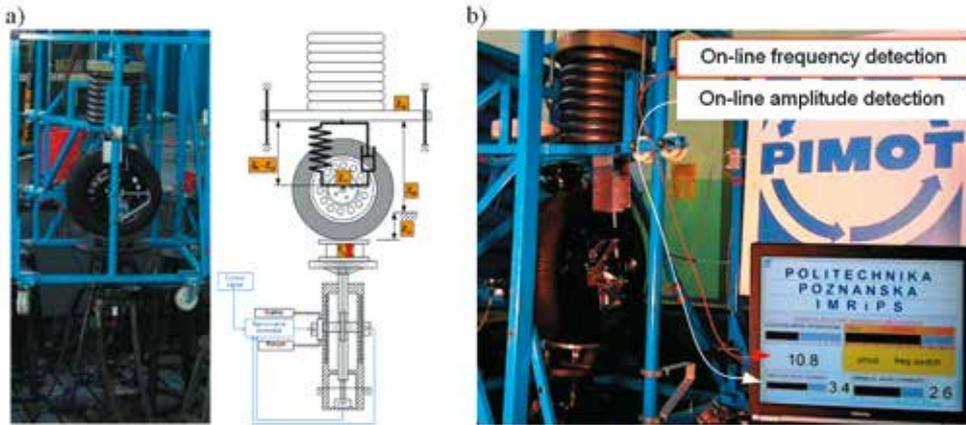
Fig. 10. Test rig for the testing of a physical quarter-car suspension model coupled with an electrohydraulic vibrator (a) and an instrument with a real-time result of the signal frequency identification algorithm being displayed on the instrument screen by the program used (b)
