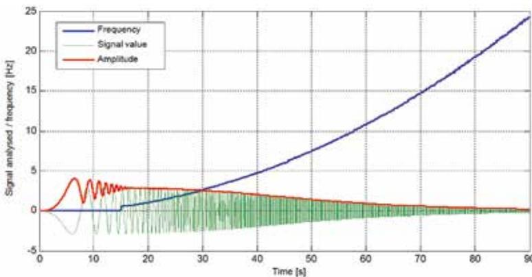
**Fig. 6. Result of the identification of signal frequency and amplitude**
