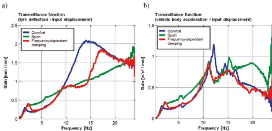
Fig. 11. Effect of smooth adjusting of the damping level to the input frequency; comparison with the suspension performance curves plotted for the suspension system with the damping having been set to the minimum (comfort) and maximum (sport) levels of the shock absorber performance range: a) tyre deflection gain curves; b) vehicle body acceleration gain curves
