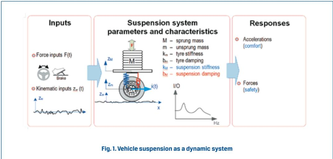
The force inputs come from inertia forces, which are generated in result of changes in the longitudinal and lateral vehicle dynamics, caused by vehicle manoeuvres performed by the driver with the use of vehicle controls. Nevertheless, the inputs that most frequently occur are kinematic inputs caused by vehicle drives on uneven road surfaces with different speeds.
