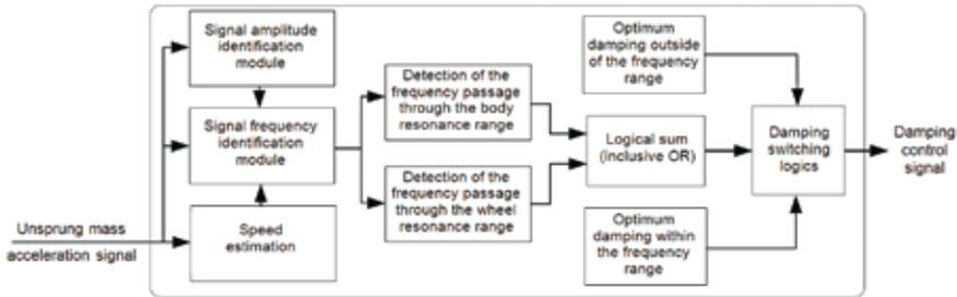
Fig. 3. Structure of the algorithm of adaptive damping control according to input frequency
