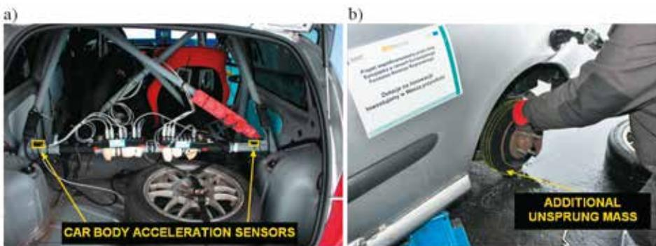
**Fig. 3. The test car Renault Clio II: a) Locations of the rear vehicle body part acceleration sensors; b) Location of the weight (non-revolving) that represented the extra unsprung mass**
