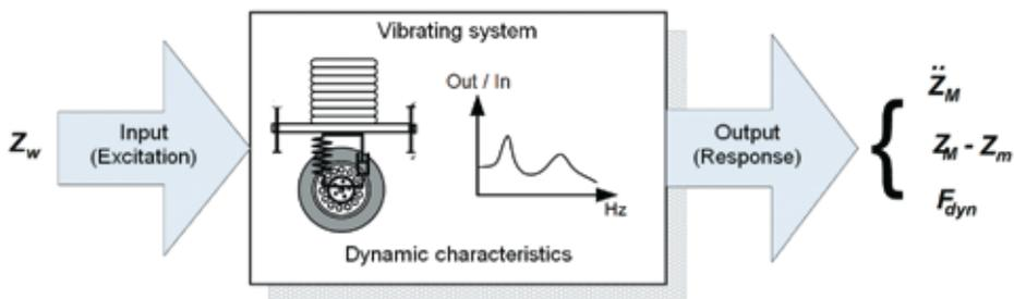
Fig. 7. Quarter-car suspension system as a dynamic system
