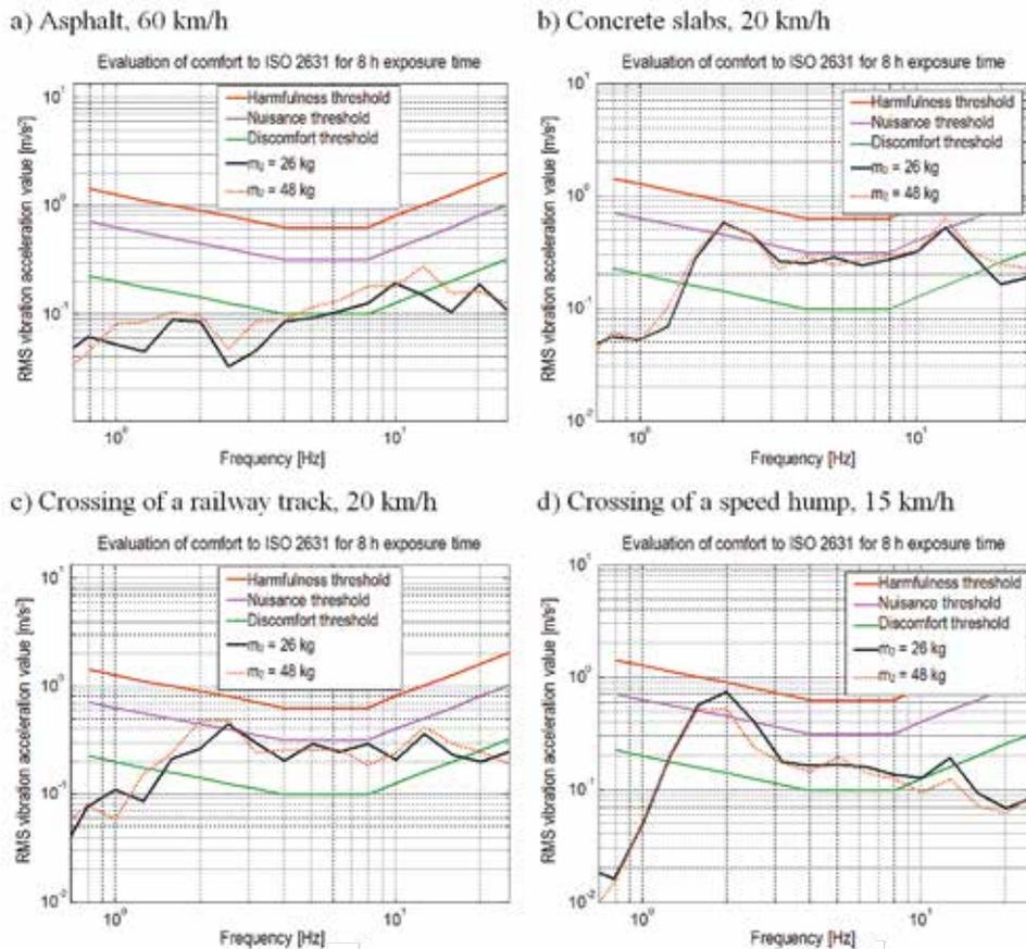
**Fig. 4. RMS acceleration values of vertical car body vibrations above the rear axle in 1/3 octave frequency bands from 0.63 Hz to 25 Hz for selected vehicle operation conditions, against the standard limit values according to ISO 2631 for 8 hour time of exposure to vibrations**
