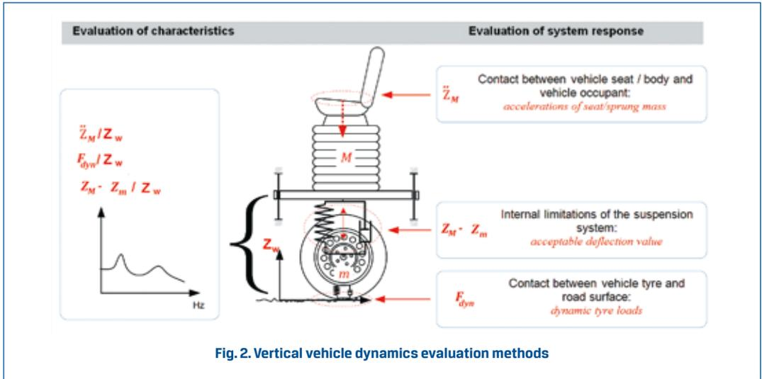
Fig. 2. Vertical vehicle dynamics evaluation methods
