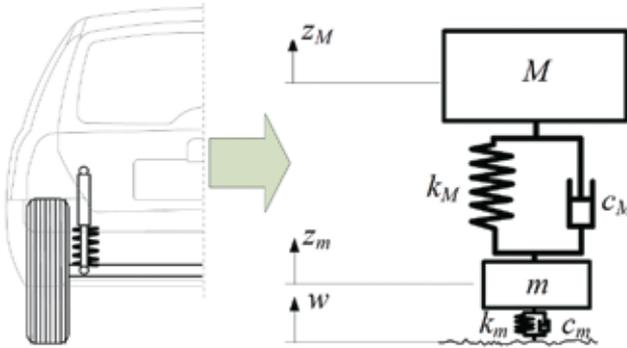
**Fig. 5. Sketch showing the simplification of a quarter of the car by reducing it to a model with two degrees of freedom**
