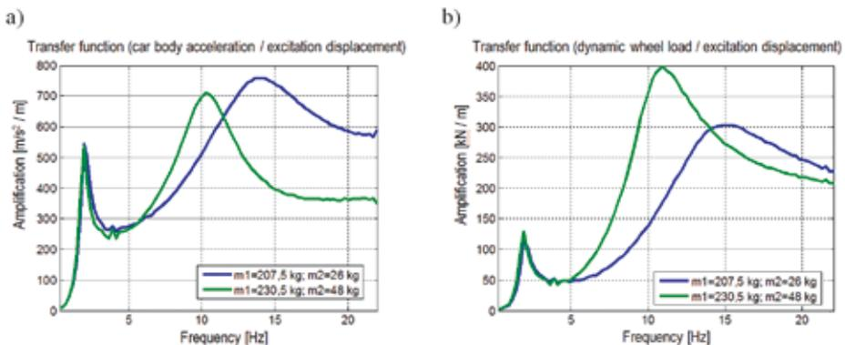
**Fig. 8. Selected dynamic characteristics of the suspension system: a) function of amplification of the excitation to accelerations  $\ddot{z}_M/w$ ; b) function of amplification of the excitation to the dynamic wheel load  $F_{dyn}$  proportional to tyre deflection  $(\dot{w} - \dot{z}_m) / w$**
