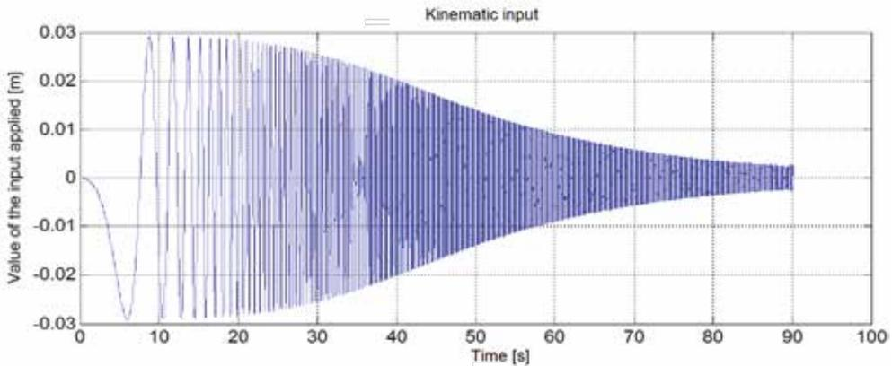
Fig. 6. Kinematic input function used to examine dynamic system characteristics
