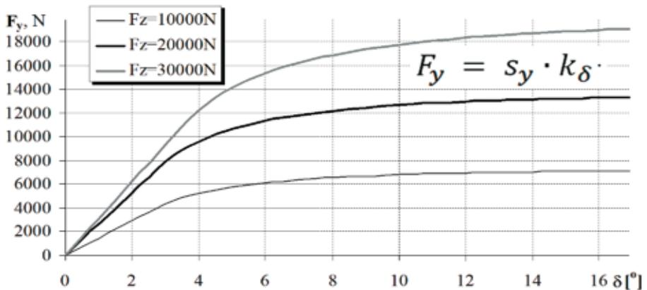
**Fig. 1 a) Changes in the lateral tyre slip  $s_y$  and coefficient of tyre resistance to sideslip  $k_\delta$  as functions of the tyre sideslip angle  $\delta$ ; b) Characteristics of the pneumatic tyre resistance to sideslip, determined for different values of normal wheel load  $F_z$ .**
