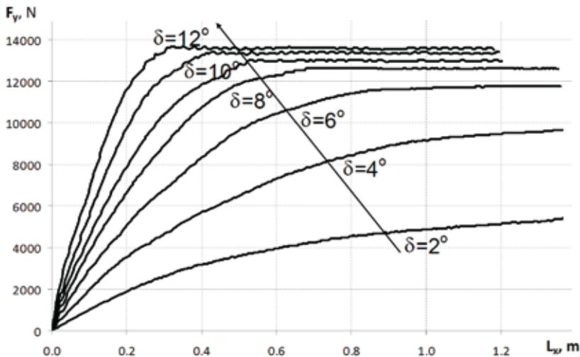
**Fig. 2. Tyre relaxation characteristics determined in quasi-static wheel motion conditions (for tyres of a medium-capacity motor truck, at normal wheel load of  $F_z = 20\,000$  N)**
