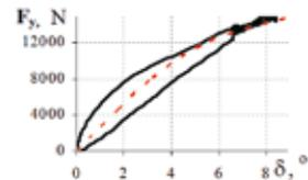
Fig. 4. Tyre relaxation in the conditions of oscillatory changes in the tyre sideslip angle: a) oscillations in the tyre sideslip angle  $\delta$  around its zero value, with different amplitudes ( $f = 2 \text{ Hz}$ ); b) oscillations in the tyre sideslip angle  $\delta$  around a preset initial constant value  $\delta_{y0}$  of this angle ( $f = 2 \text{ Hz}$ ,  $A = 1^\circ$ ,  $v_x = 60 \text{ km/h}$ )
