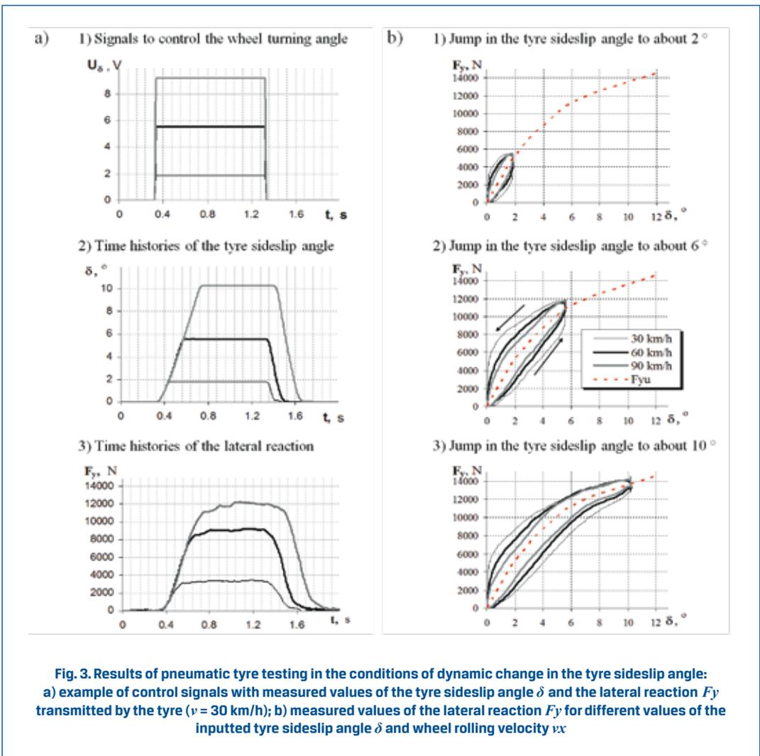
**Fig. 3. Results of pneumatic tyre testing in the conditions of dynamic change in the tyre sideslip angle: a) example of control signals with measured values of the tyre sideslip angle  $\delta$  and the lateral reaction  $F_y$  transmitted by the tyre ( $v = 30$  km/h); b) measured values of the lateral reaction  $F_y$  for different values of the inputted tyre sideslip angle  $\delta$  and wheel rolling velocity  $v_x$**
