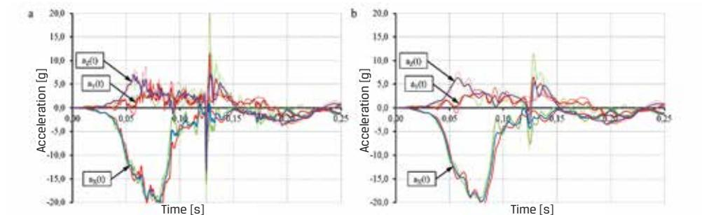
**Fig. 7. Scatter of the results of measurements of torso acceleration components in the local coordinate system, observed when repeating variant 2 of the experiment: a – CFC180 filtration; b – CFC60 filtration**
