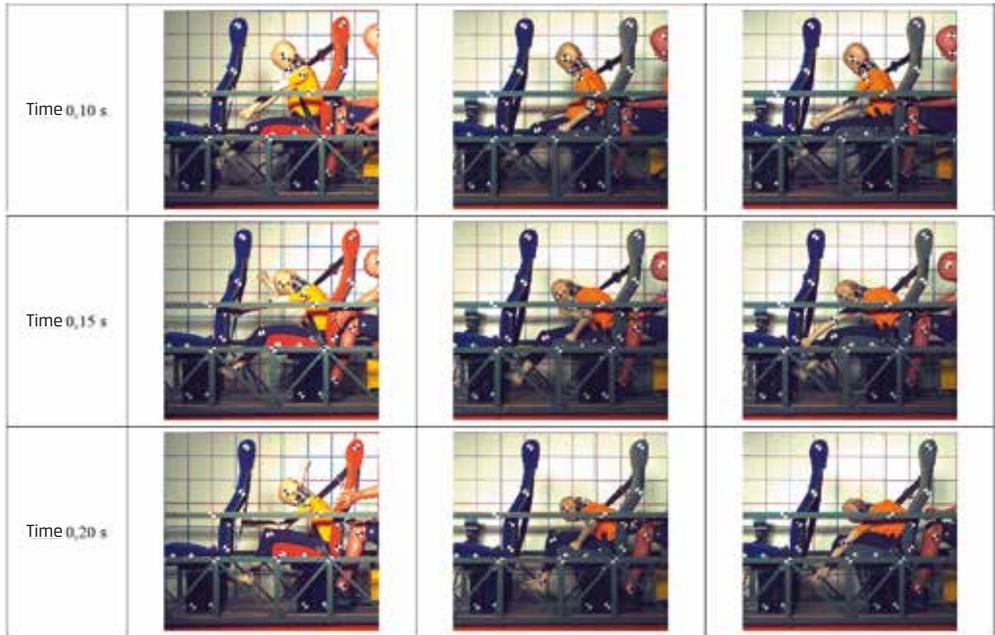
Based on a frame-by-frame analysis of the video records, successive positions (in 0.01 s intervals) of markers stuck on the dummy were identified. The head and torso trajectories thus determined (Figs. 4 and 5) made a basis for a general assessment of the influence of the seat belt strap position on dummy's movement and on the resulting hazards. A few important details about this movement have been presented in subsequent parts of this paper.
