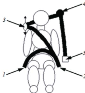
**Fig. 1. Example of a system to adjust the position of the shoulder portion of a three-point seat belt:
