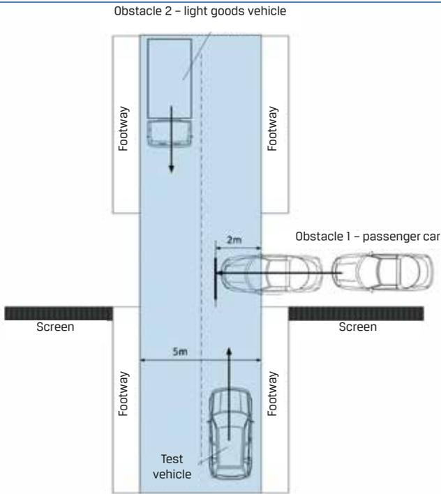
**Fig. 2. Schematic diagram of scenario 1 of the tests**
