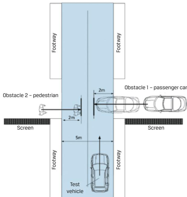
Fig. 4. Schematic diagram of scenario 5 of the tests
