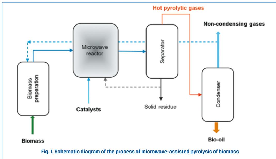
Fig. 1. Schematic diagram of the process of microwave-assisted pyrolysis of biomass
