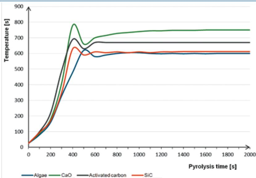
Fig. 2. The course of the microwave pyrolysis process depending on the absorber used
