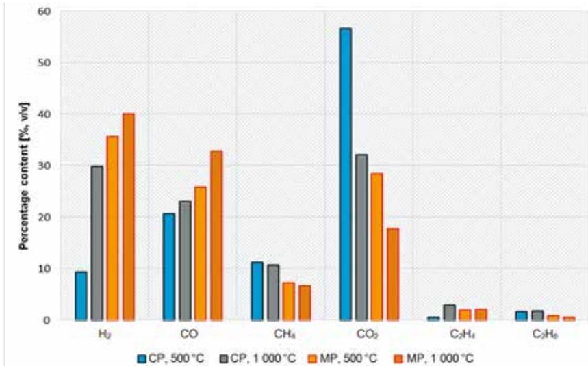
**Fig. 3. Comparison between the volumes of gases yielded by the pyrolysis processes of both types at temperatures of 500°C and 1 000°C:**
