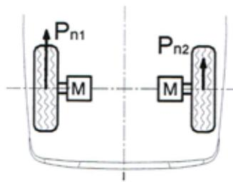
**Fig. 12. Implementation of the active differential functions by using separate motors to drive the road wheels of the vehicle**
