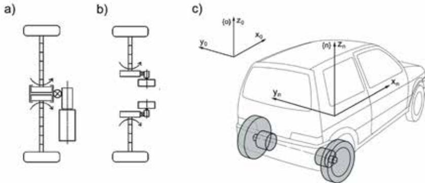
**Fig. 6. Model simulation testing of an urban vehicle with two different rear wheel driving methods:**
