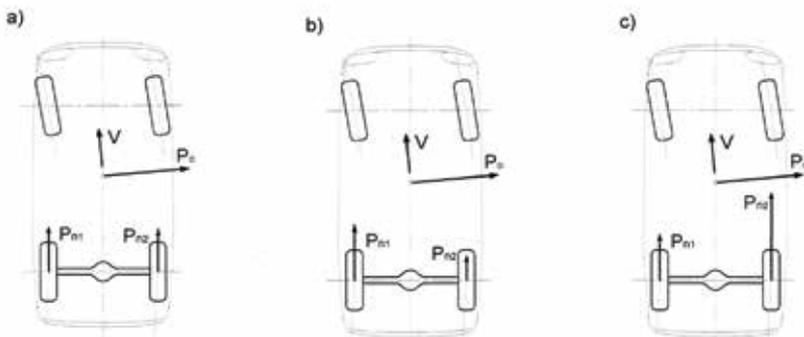
**Fig. 1. Distribution of driving forces between wheels in a turning vehicle, in the case of various differential gears: a) simple (open) differential; b) limited slip differential; c) active differential gear performing the "torque vectoring" function**
