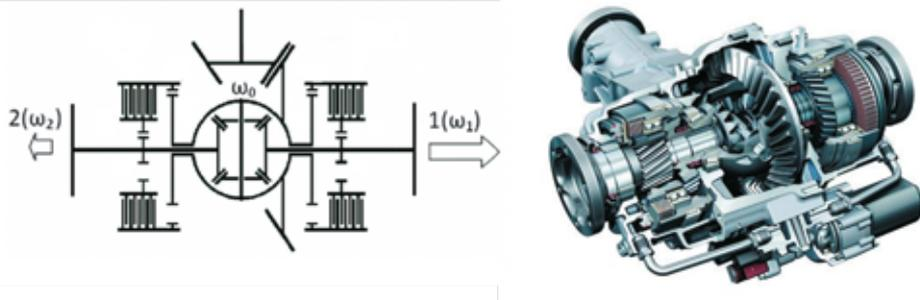
**Fig. 14. Schematic diagram and view of the active differential gear developed by Audi**
