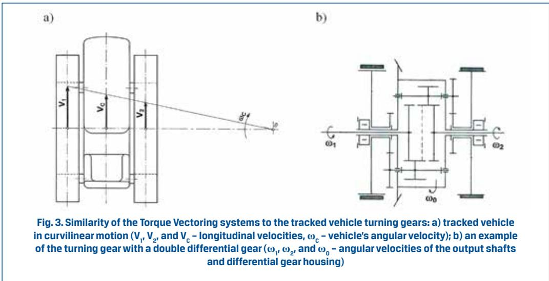
A similar process can be observed in motor vehicles. By imposing different driving forces on the road wheels of a single drive axle or by diversifying the angular velocities of the wheels, a vehicle yaw torque  $M_z$  is generated. Then, if such an input is consistent with the sign of the steering wheel turning angle, the tyre sideslip angle is changed and the vehicle turning effect is enhanced.
