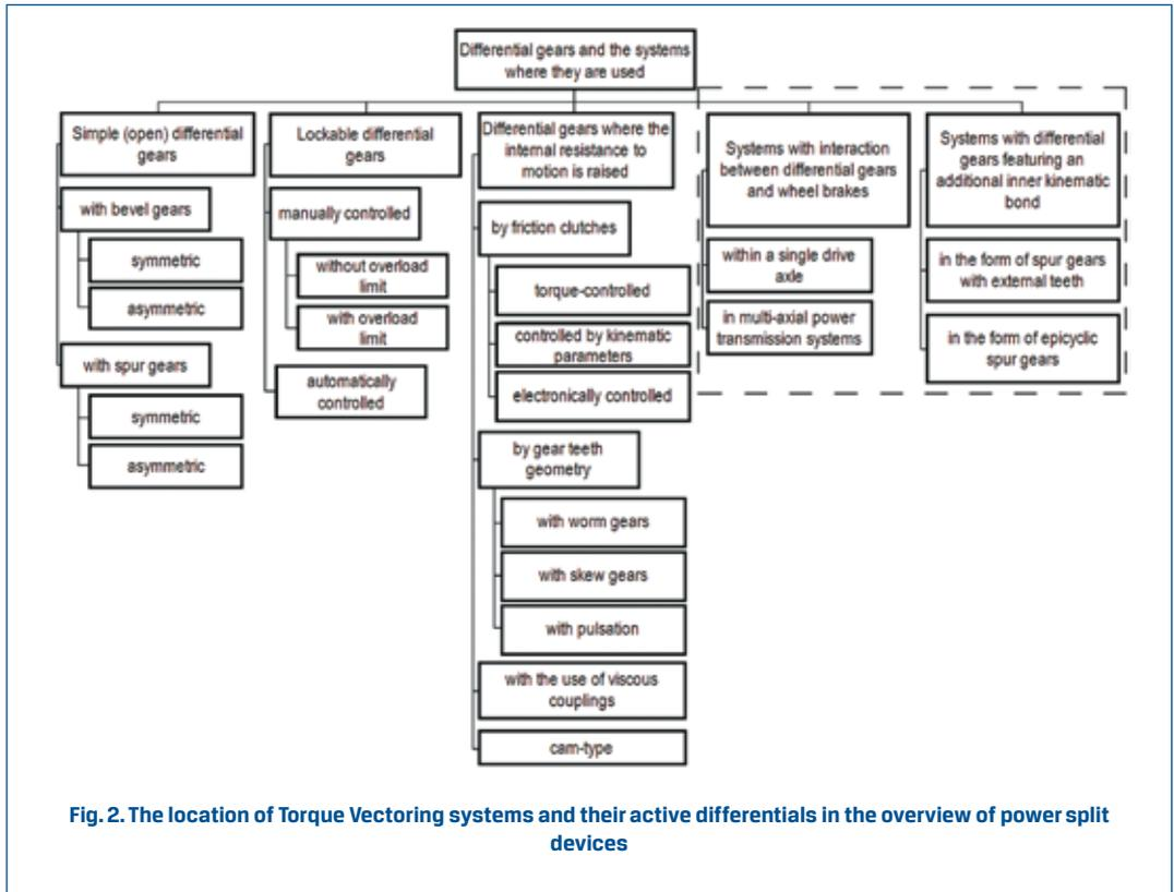
**Fig. 2. The location of Torque Vectoring systems and their active differentials in the overview of power split devices**
