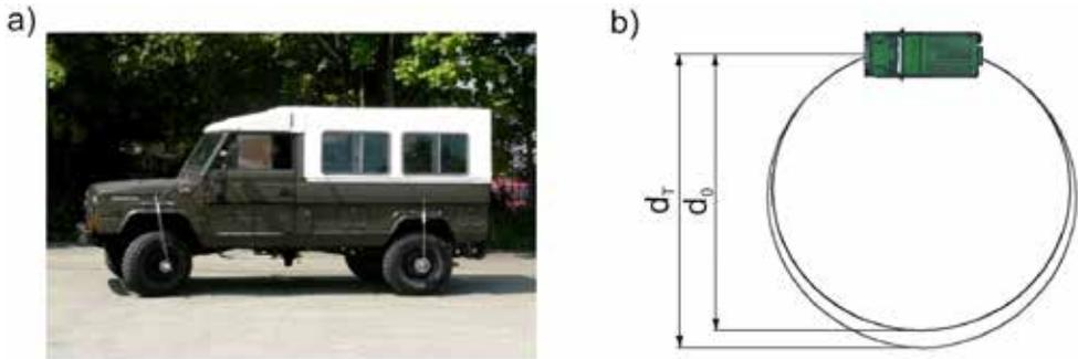
**Fig. 4. The testing of a Honker 4x4 vehicle having a rear drive axle differential with variable inner friction torque  $M_T$ : vehicle path diameter  $d_0 = 10.25$  m for  $M_T = 0$  and  $d_1 = 11.40$  m for  $M_T = 800$  Nm**
