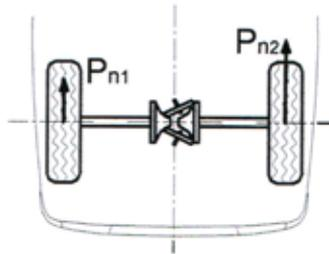
**Fig. 9. Implementation of the function of an active differential by the application of a variable-ratio toroidal friction gear**
