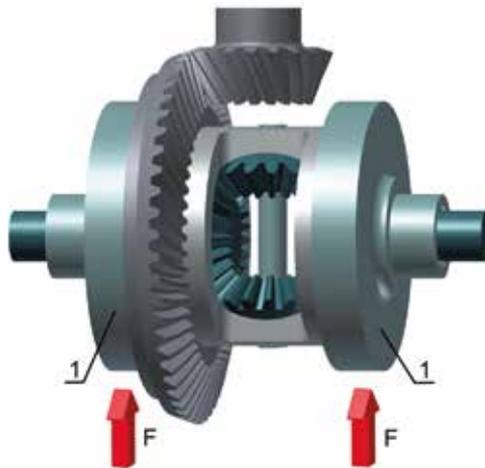
**Fig. 15. General concept of an active differential gear of a new type: 1 – multiplying transmissions of a new type; F – radial forces to control the transmission ratios**
