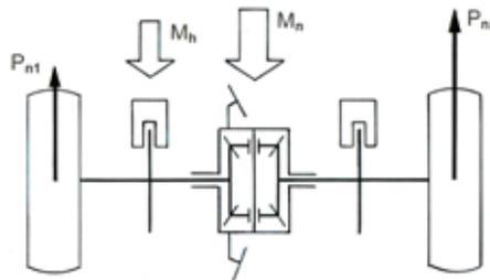
**Fig. 11. Differentiation of wheel driving forces by means of a simple differential gear and separately controlled wheel brakes**
