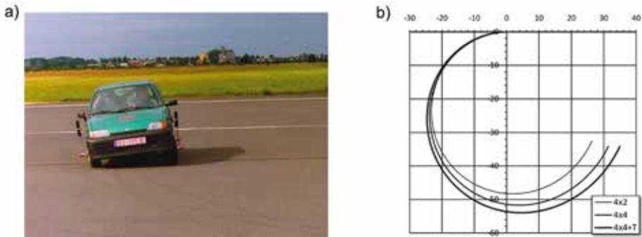
**Fig. 5. A prototype Cinquecento 4x4 car during field tests (a) and the vehicle paths obtained for different modes of operation of the car's power transmission system, i.e. 4x2, 4x4, and 4x4+T (b)**
