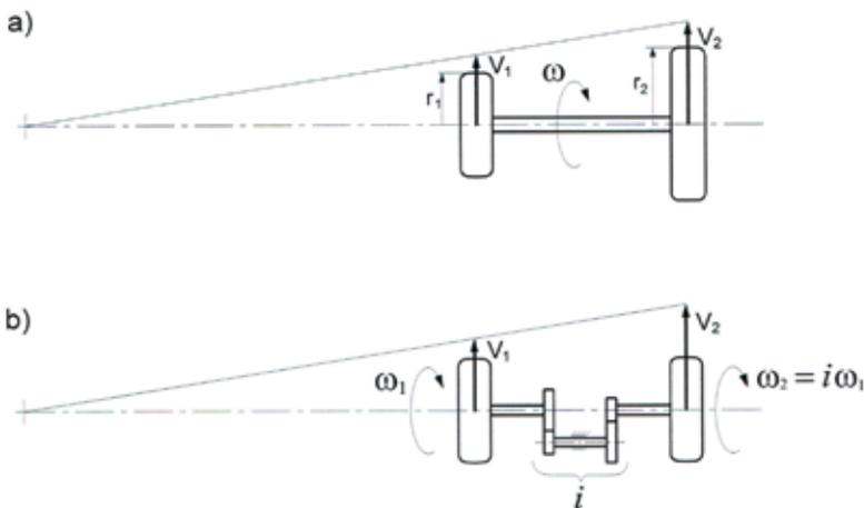
**Fig. 10. Idea of an additional kinematic bond in the active differential gears: a) wheels of different radii coupled by a rigid shaft; b) wheels of equal radii kinematically coupled by a gear train**
