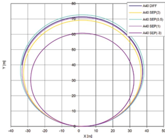
**Fig. 7. Results of model simulation tests of a Cinquecento 4x4 vehicle at 40 km/h speed and various outer to inner wheel torque ratios  $SEP = M_z / M_w$**
