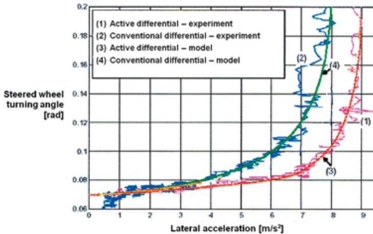
Fig. 8. Handling characteristics of a vehicle with an active differential gear fitted in its rear axle when driven on a circle with a radius of  $R_s = 40$  m on a surface with good grip, according to [1]
