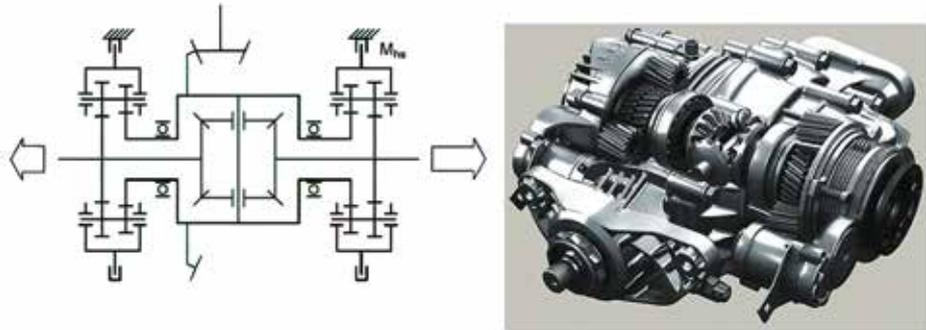
**Fig. 13. Schematic diagram and view of the active differential gear applied to the rear drive axle of the BMW X6 car**
