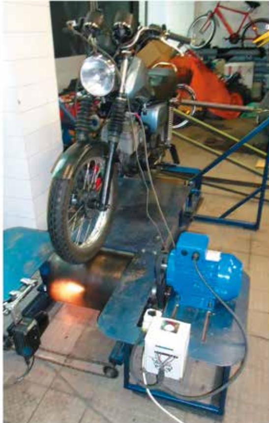
**Fig. 4. Motorcycle on the test stand**
