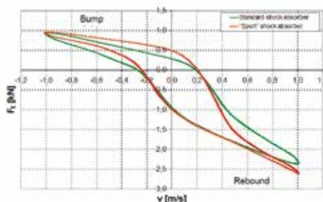
Fig. 3. Force-displacement  $P_t = f(s)$  and force-velocity  $P_t = f(v)$  (damping) characteristics of the standard and "sport" shock absorbers of the front wheel suspension system of the VW Passat test vehicle (green and red curves, respectively)
