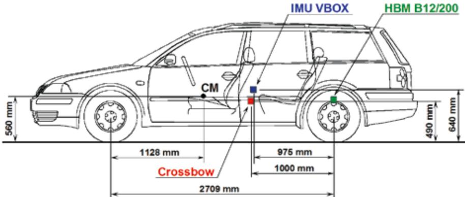
**Fig. 5. Approximate locations of the Crossbow and VBOX inertial blocks and the HBM sensor:**
