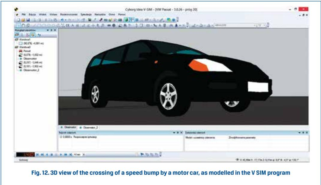
**Fig. 12. 3D view of the crossing of a speed bump by a motor car, as modelled in the V SIM program**
