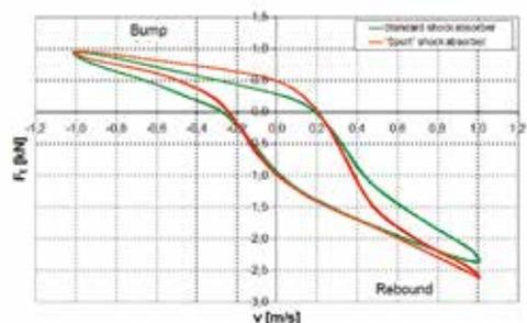
Fig. 3. Force-displacement  $P_t = f(s)$  and force-velocity  $P_t = f(v)$  (damping) characteristics of the standard and "sport" shock absorbers of the front wheel suspension system of the VW Passat test vehicle (green and red curves, respectively)
