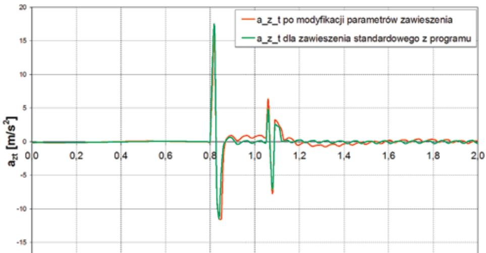
**Fig. 15.** Time histories of the vertical acceleration of a car body point over the rear wheel axle, calculated from a simulation in the V SIM program for the crossing of a single speed bump with a speed of about 40 km/h and for the standard suspension system parameters available from the program database (green curve) and for the parameters having been modified as described above (orange curve)
