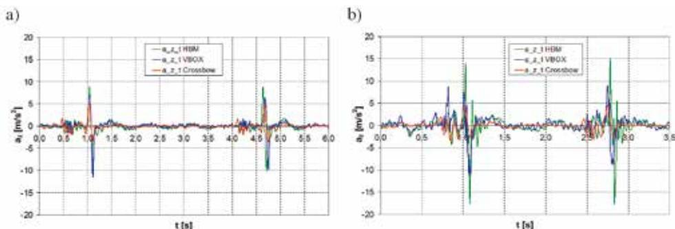
**Fig. 11. Time histories of the vertical acceleration of a car body point over the rear wheel axle, calculated (red and blue curves) and measured (green curve), for the car with the "sport" shock absorbers crossing the speed bump with speeds of 20 km/h (graph "a") and 40 km/h (graph "b"),**
