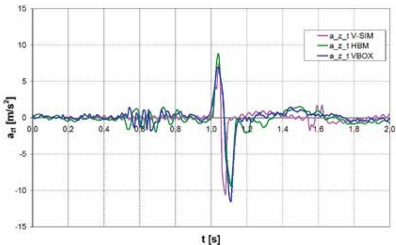
Fig. 13. Time histories of the vertical acceleration of a car body point over the rear wheel axle, obtained by calculation from the V SIM program (pink curve) and from the VBOX data (blue curve) and measured with an HBM B12/200 acceleration sensor (green curve), for the car with the "sport" shock absorbers crossing the speed bump with a speed of 20 km/h
