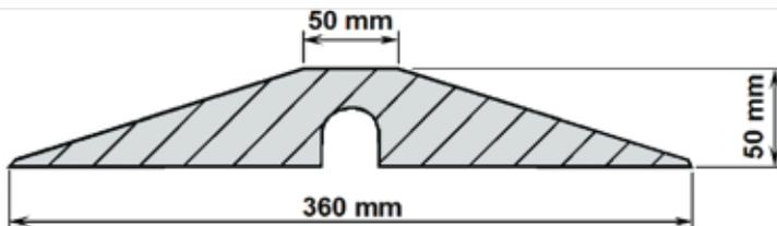
**Fig. 6. Profile of the speed bump used at the road tests of the VW Passat car**
