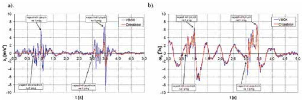
Fig. 9. Time histories of the vertical acceleration  $a_z$  and pitch rate  $\omega_y$  measured with the use of the Crossbow and VBOX instruments for the vehicle crossing the speed bumps with a speed of 40 km/h
