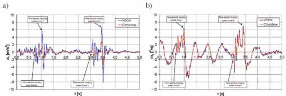
Fig. 8. Time histories of the vertical acceleration  $a_z$  and pitch rate  $\omega_y$  measured with the use of the Crossbow and VBOX instruments for the vehicle crossing the speed bumps with a speed of 30 km/h
