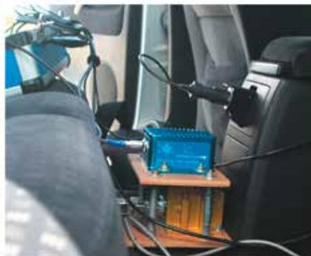
Fig. 2. A view of the VBOX and Crossbow measuring equipment installed in the vehicle interior
