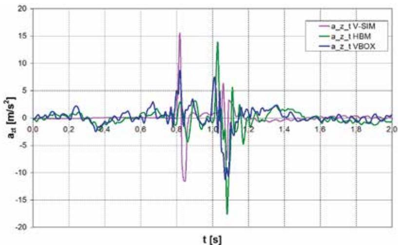
Fig. 14. Time histories of the vertical acceleration of a car body point over the rear wheel axle, obtained by calculation from the V SIM program (pink curve) and from the VBOX data (blue curve) and measured with an HBM B12/200 acceleration sensor (green curve), for the car with the "sport" shock absorbers crossing the speed bump with a speed of 40 km/h
