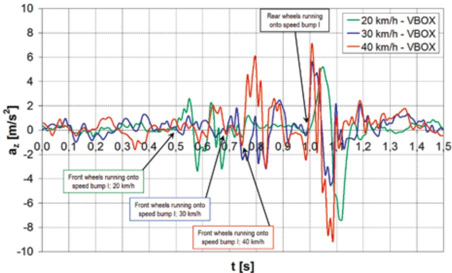
**Fig. 10. Comparison of time histories of vertical vehicle acceleration  $a_z$  recorded when the car with the "sport" shock absorbers crossed a speed bump with speeds of 20 km/h, 30 km/h, and 40 km/h**
