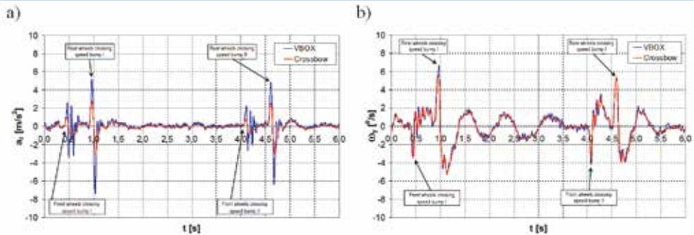
Fig. 7. Time histories of the vertical acceleration  $a_z$  and pitch rate  $\omega_y$  measured with the use of the Crossbow and VBOX instruments for the vehicle crossing the speed bumps with a speed of 20 km/h
