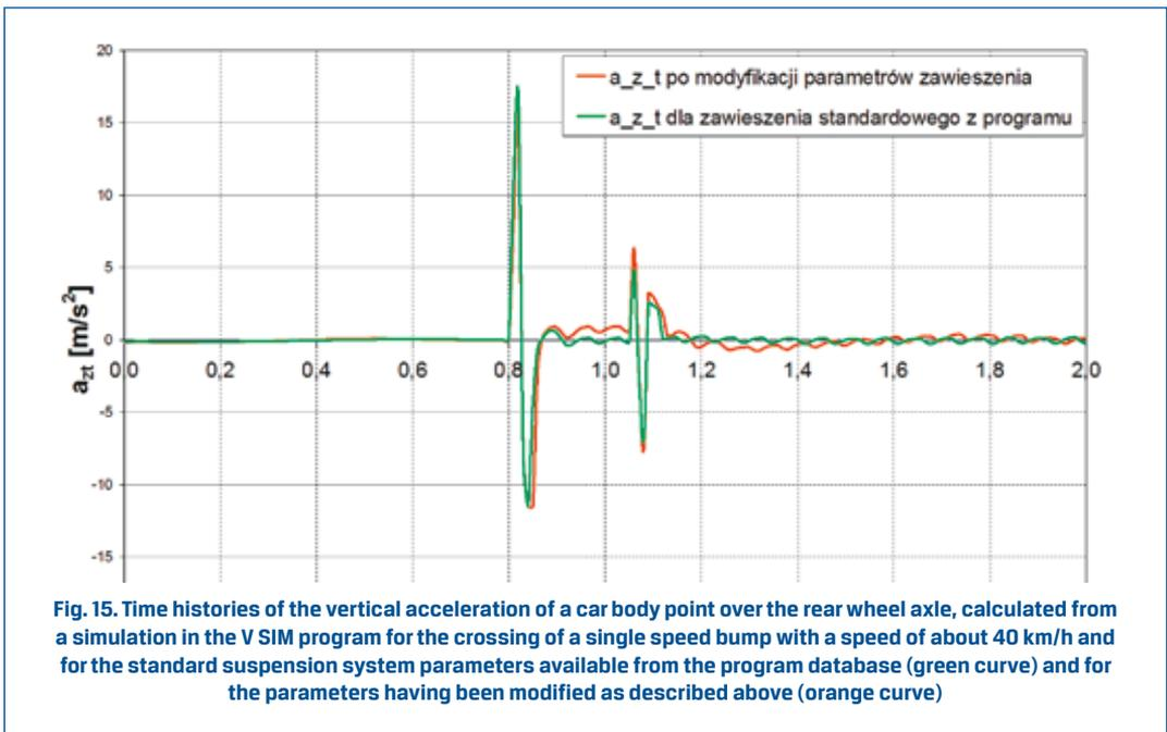
**Fig. 15. Time histories of the vertical acceleration of a car body point over the rear wheel axle, calculated from a simulation in the V SIM program for the crossing of a single speed bump with a speed of about 40 km/h and for the standard suspension system parameters available from the program database (green curve) and for the parameters having been modified as described above (orange curve)**
