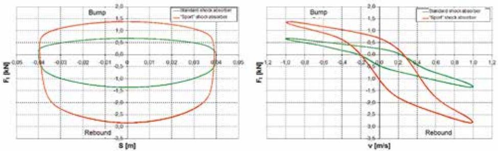
**Fig. 4. Force-displacement  $P_1 = f(s)$  and force-velocity  $P_1 = f(v)$  (damping) characteristics of the standard and "sport" shock absorbers of the rear wheel suspension system of the VW Passat test vehicle (green and red curves, respectively)**
