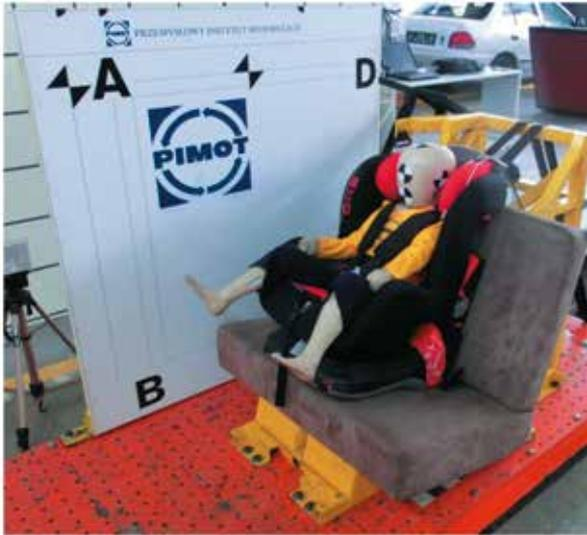
**Fig. 7. General view of the child dummy placed in a child safety seat, which was secured to a vehicle seat rigidly mounted on the measuring trolley**
