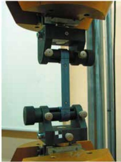
Fig. 4. Method of gripping seat belt strap specimens on the measuring stand built on an Instron 8802 tensile-testing machine
