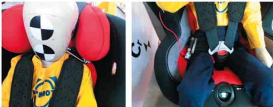
**Fig. 9. View of the load cells used to measure the forces developing in the shoulder and hip portions of the safety harness securing the test dummy in the child safety seat**
