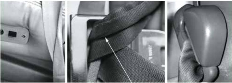
**Fig. 2. Examples of folded seat belt straps [2]**
