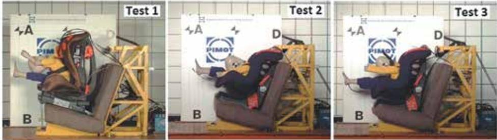
**Fig. 8. Maximum dummy's displacements during the tests (video record frames): test 1 – safety seat 1; tests 2 and 3 – safety seat 2**
