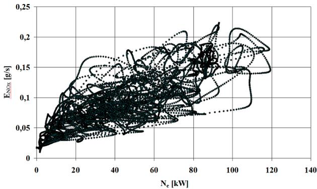
**Fig. 12. Correlation relationship between nitrogen oxides emission rate ( $E_{NOx}$ ) and effective power ( $N_e$ ) of the engine in the NRTC test**
