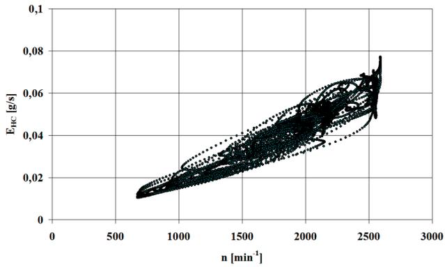
Fig. 5. Correlation relationship between hydrocarbons emission rate ( $E_{HC}$ ) and engine speed ( $n$ ) in the NRTC test
