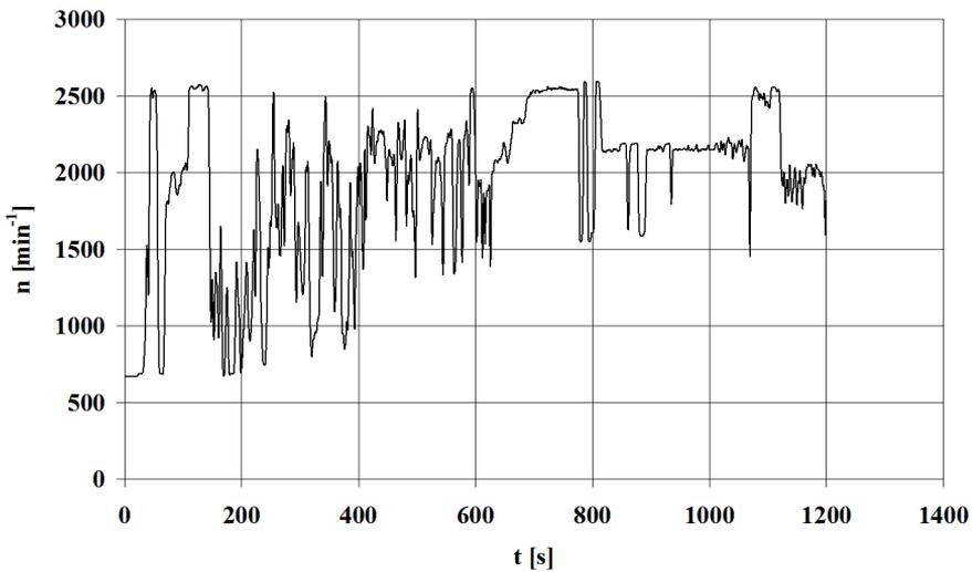
**Fig. 1. Engine speed ( $n$ ) vs. time ( $t$ ) curve, recorded during the NRTC test**
