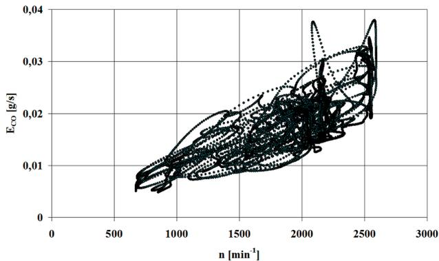
**Fig. 4.** Correlation relationship between carbon monoxide emission rate ( $E_{CO}$ ) and engine speed ( $n$ ) in the NRTC test
