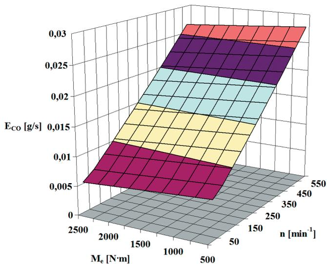
Fig. 13. Graph representing the second-degree polynomial function that approximates the dependence of carbon monoxide emission rate ( $E_{CO}$ ) on engine speed ( $n$ ) and torque ( $M_e$ )
