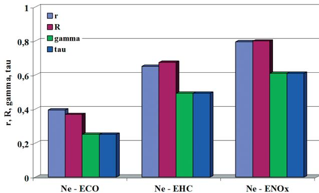
**Fig. 21. Coefficients of Pearson's linear correlation ( $r$ ), Spearman's rank correlation ( $R$ ), Kruskal's gamma correlation ( $\gamma$ ), and Kendall's tau correlation ( $\tau$ ) of carbon monoxide emission rate (ECO), hydrocarbons emission rate (EHC), and nitrogen oxides emission rate (ENOx) with effective power ( $Ne$ ) of the engine under test**
