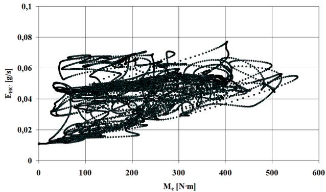
Fig. 8. Correlation relationship between hydrocarbons emission rate ( $E_{HC}$ ) and engine torque ( $M_e$ ) in the NRTC test
