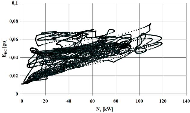
**Fig. 11. Correlation relationship between hydrocarbons emission rate ( $E_{HC}$ ) and effective power ( $N_e$ ) of the engine in the NRTC test**
