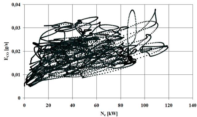
Fig. 10. Correlation relationship between carbon monoxide emission rate ( $E_{CO}$ ) and effective power ( $N_e$ ) of the engine in the NRTC test
