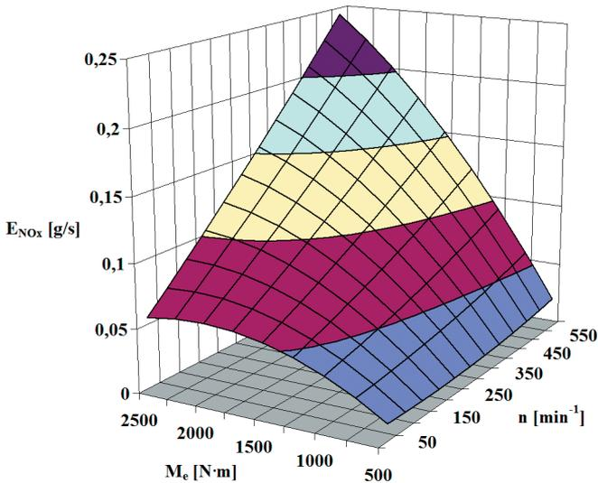
**Fig. 15. Graph representing the second-degree polynomial function that approximates the dependence of nitrogen oxides emission rate ( $E_{NO_x}$ ) on engine speed ( $n$ ) and torque ( $M_e$ )**
