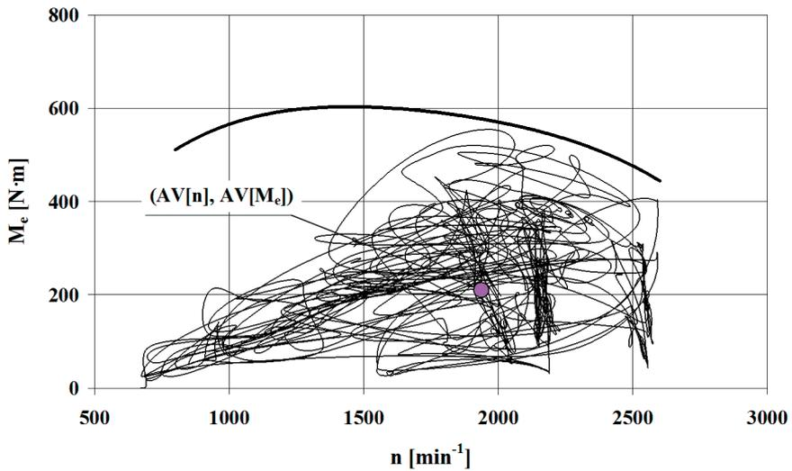
**Fig. 3.** The set of the IC engine operation states during the NRTC test against the background of the full-load torque vs. speed curve:  $n$  – engine speed;  $AV[n]$  – average value of the engine speed;  $AV[M_e]$  – average value of the engine torque
