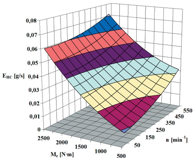
Fig. 14. Graph representing the second-degree polynomial function that approximates the dependence of hydrocarbons emission rate ( $E_{HC}$ ) on engine speed ( $n$ ) and torque ( $M_e$ )
