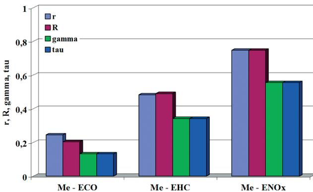
**Fig. 20.** Coefficients of Pearson's linear correlation ( $r$ ), Spearman's rank correlation ( $R$ ), Kruskal's gamma correlation ( $\gamma$ ), and Kendall's tau correlation ( $\tau$ ) of carbon monoxide emission rate (ECO), hydrocarbons emission rate (EHC), and nitrogen oxides emission rate (ENOX) with engine torque ( $Me$ )
