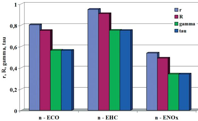
**Fig. 19.** Coefficients of Pearson's linear correlation ( $r$ ), Spearman's rank correlation ( $R$ ), Kruskal's gamma correlation ( $\gamma$ ), and Kendall's tau correlation ( $\tau$ ) of carbon monoxide emission rate (ECO), hydrocarbons emission rate (EHC), and nitrogen oxides emission rate (ENOX) with engine speed ( $n$ )
