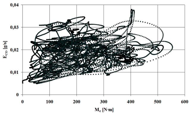
Fig. 7. Correlation relationship between carbon monoxide emission rate ( $E_{CO}$ ) and engine torque ( $M_e$ ) in the NRTC test
