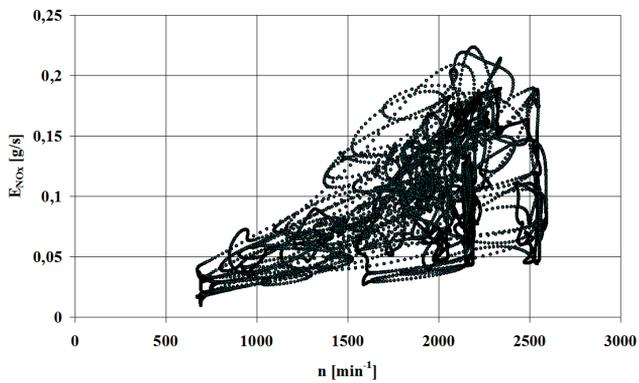
Fig. 6. Correlation relationship between nitrogen oxides emission rate ( $E_{NOx}$ ) and engine speed ( $n$ ) in the NRTC test
