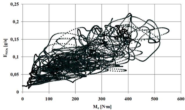
Fig. 9. Correlation relationship between nitrogen oxides emission rate ( $E_{NOx}$ ) and engine torque ( $M_e$ ) in the NRTC test
