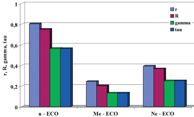
Fig. 16. Coefficients of Pearson's linear correlation (r), Spearman's rank correlation (R), Kruskal's gamma correlation (gamma), and Kendall's tau correlation (tau) between carbon monoxide emission rate (ECO) and speed (n), torque (Me), and effective power (Ne) of the engine under test
