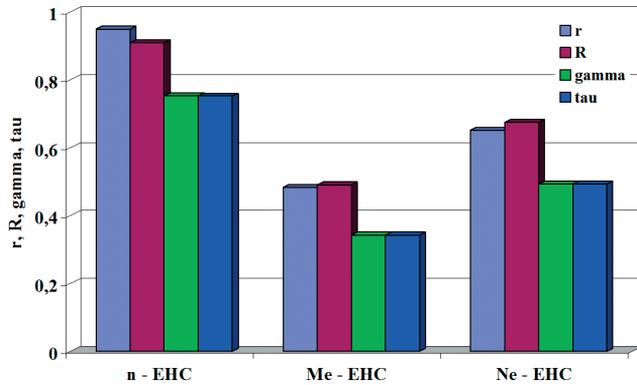
Fig. 17. Coefficients of Pearson's linear correlation (r), Spearman's rank correlation (R), Kruskal's gamma correlation (gamma), and Kendall's tau correlation (tau) between hydrocarbons emission rate (EHC) and speed (n), torque (Me), and effective power (Ne) of the engine under test
