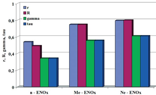
Fig. 18. Coefficients of Pearson's linear correlation (r), Spearman's rank correlation (R), Kruskal's gamma correlation (gamma), and Kendall's tau correlation (tau) between nitrogen oxides emission rate (ENOX) and speed (n), torque (Me), and effective power (Ne) of the engine under test
