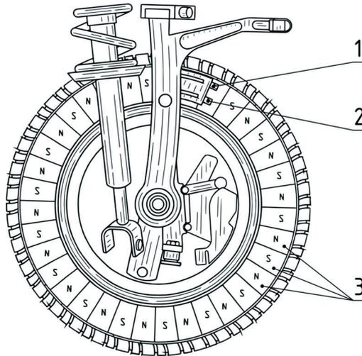
**Fig. 11. System with magnetic field sensors being used for measuring the tangential and lateral components of tyre deformation: 1, 2 – magnetic field sensors (magnetoresistors or Hall sensors); 3 – alternating magnetic poles fabricated in a ferromagnetic band incorporated into the inner surface of the tyre sidewall [12]**
