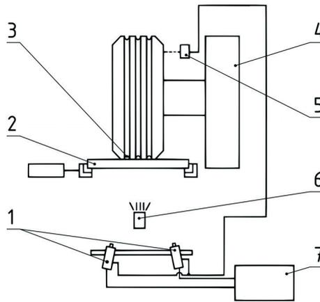
**Fig. 8. Laboratory test stand with a stereovision system for measuring the geometrical dimensions and deformation of tyre tread: 1 – cameras; 2 – transparent base plate; 3 – tread grooves deformed when being in contact with the base plate; 4 – wheel loading device; 5 – synchronized camera release system; 6 – illuminator (light source); 7 – computing unit [15]**
