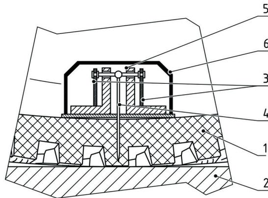
**Fig. 6. Cross-section of a set-up (transducer) for the measuring of tread lug deformations with the use of Surface Acoustic Wave (SAW) sensors: 1 – tyre; 2 – road surface; 3 – SAW sensor; 4 – pin (acting as lever); 5 – overload protection; 6 – transducer housing [23]**
