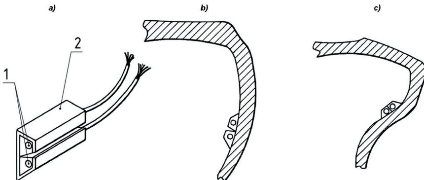
**Fig. 4. a) Variable capacitance sensor of the radial deformation of a tyre; b) Sensor fixed to the inner surface of the tyre sidewall, with the sidewall being in a relaxed position; c) Sensor fixed to the inner surface of the tyre sidewall, with the sidewall being deformed owing to the load applied: 1 - electrode; 2 - sensor's housing with a V-shaped groove [6]**
