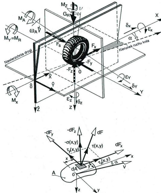
**Fig. 1. Illustration of a tyre deformation occurring and forces acting on the tyre during interaction between the tyre and the road surface [7]**
