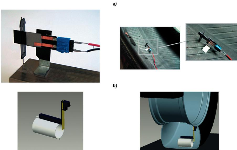
**Fig. 7. Examples of piezoelectric transducers for measuring the lateral component of tyre deformation, utilizing a flexible beam coated with PVDF film [10]**
