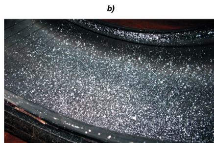
**Fig. 9. a) Camera adapted for being mounted on the wheel rim inside the tyre, intended for tyre deformation measurements; b) inner surface of the tyre, with a random speckle pattern applied to it [13]**
