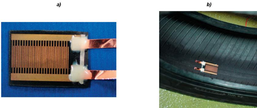
**Fig. 3. Variable capacitance tyre deformation sensor: a) interdigital capacitor having a pair of electrodes fabricated by photolithography in a 150 nm gold layer deposited on a rubber substrate; b) tyre adapted to deformation measurement, having the interdigital capacitor fixed on the inner tyre surface [18]**
