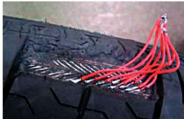
**Fig. 13. Tyre prepared for sensorless measurement of tyre belt circumferential strain; deformation measurement based on investigation of the relationship between tyre belt strain and capacitance of an interdigital capacitor composed of tyre belt wires (as electrodes) and rubber (as a dielectric material) [19]**
