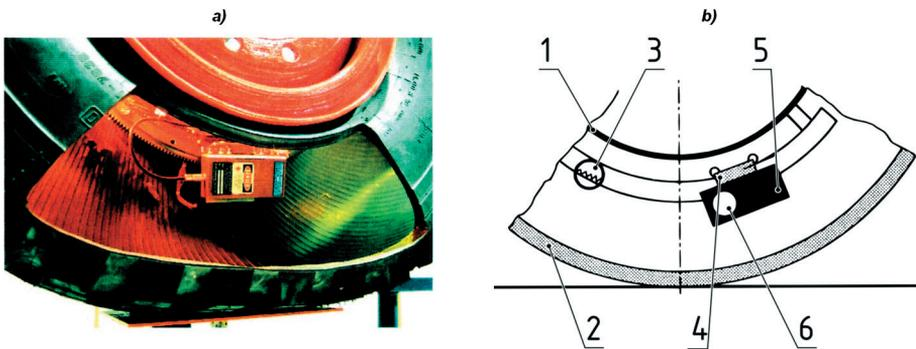
**Fig. 10. Laser head adapted for measuring the radial component of tyre deformation: a) laser head assembly installed inside a tyre; b) measuring setup schematic: 1 – rim; 2 – tyre; 3 – toothed guide; 4 – self-propelled laser head carriage; 5 – laser head; 6 – stepper motor [2]**
