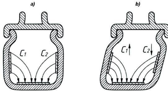
**Fig. 5. Three-electrode plate capacitor as a variable capacitance sensor of the lateral component of tyre deformation, with the electrodes having been mounted on the inner tyre surface: a) tyre undeformed,  $C_1 = C_2$ , b) tyre deformed owing to a lateral force applied,  $C_1 > C_2$  [14]**
