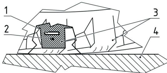
**Fig. 12. Integral magnetic sensor of tread lug deformation, based on on a matrix of Hall sensors; schematic diagram of the measuring system: 1 – integrated circuit with a matrix of Hall sensors; 2 – permanent magnet; 3 – tread lugs; 4 – road surface [27]**
