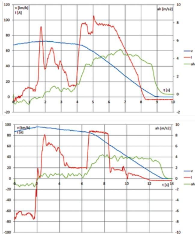
**Fig. 3. Regenerative charging current at braking with a deceleration of about  $4\text{--}4.5\text{ m/s}^2$  from an initial speed of 70 km/h (top) and 90 km/h (bottom)**
