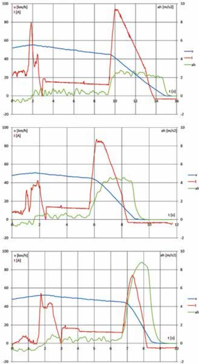
Fig. 2. Regenerative charging current at different braking deceleration values from an initial speed of 50 km/h
