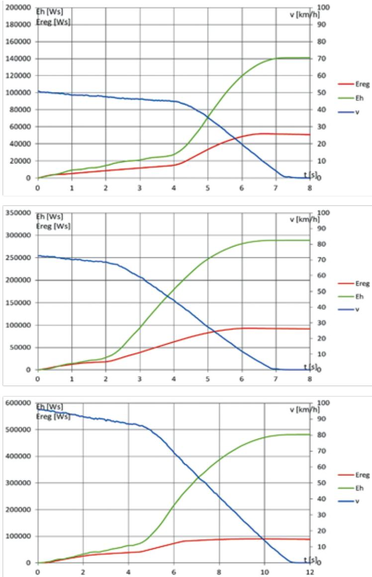
Fig. 5. Energy  $E_h$  taken away ("consumed") during the vehicle braking process and electric energy  $E_{reg}$  recovered ("regenerated") vs. the braking time, at a braking deceleration of 4–4.5 m/s<sup>2</sup>
