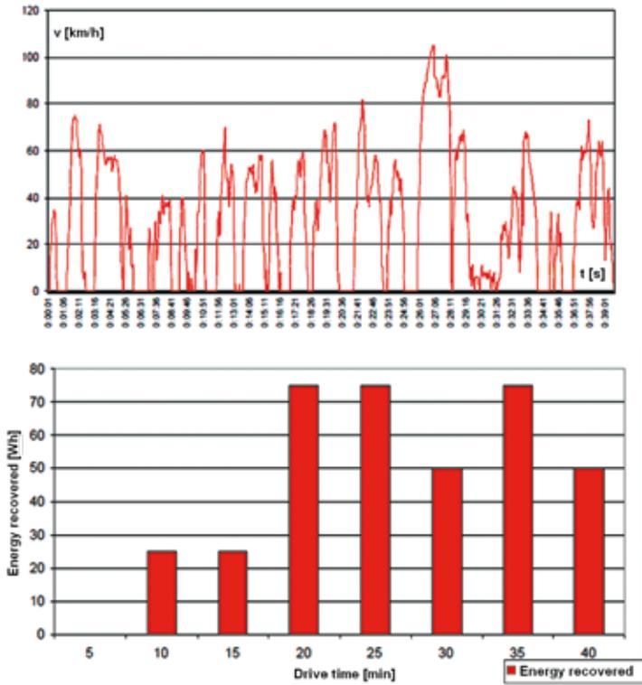
Fig. 4. Vehicle speed and energy recovered during the test drive performed in the urban driving cycle conditions [7]
