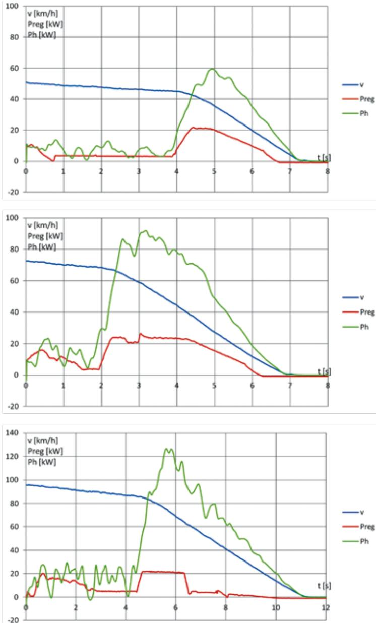
Fig. 6. Demand for braking power and regenerative braking power at various initial vehicle braking speeds
