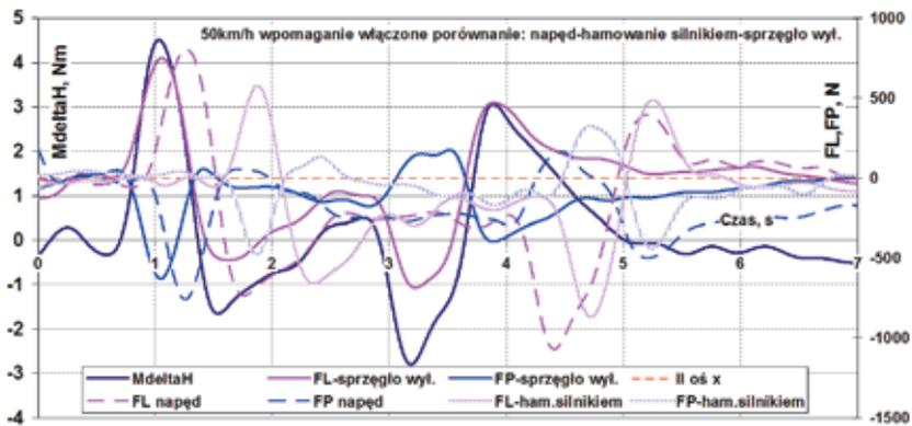
Fig. 5. Comparison of forces in the steering rods on the drive, engine braking and free-wheeling. Drive through the lowered ground roadside. Speed 50 km/h, Power steering on. Symbols: FL – force measured in the left steering rod, FP – force measured in the right steering rod, MdeltaH – rotation torque on the driving wheel
