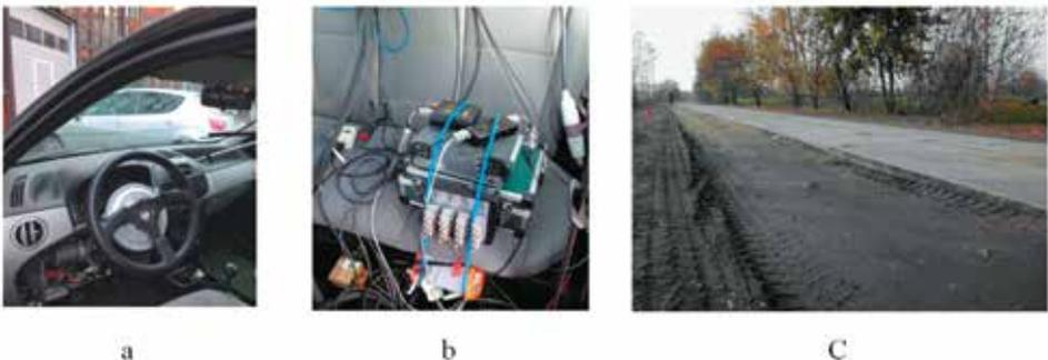
**Fig. 2. A set of instruments (a measuring steering wheel and AD32 processing and re-cording device) as well as a sample view of the test track (a concrete-surface road with the lowered ground roadside)**
