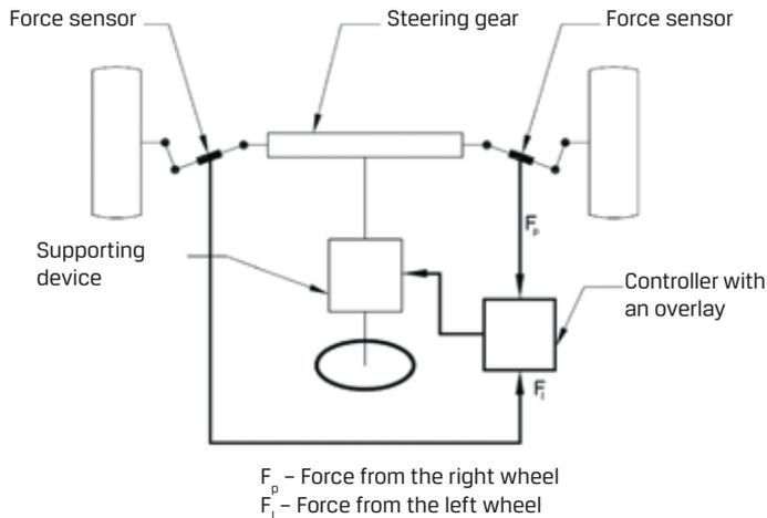
**Fig. 1 Schematic diagram of the proposed solutions to the control system.**
