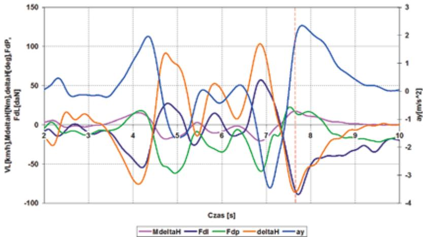
Fig. 4. Drive through the lowered roadside. Speed 40 km/h, Standard power steering on. Symbols as in figure 3
