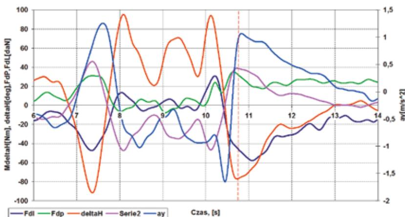
**Fig. 3. Drive through the lowered roadside. Speed 40km/h, Power steering off. Symbols: FL - force measured in the left steering rod, FP - force measured in the right steering rod, deltaH - driving wheel rotation angle, MdeltaH - rotation torque on the driving wheel, ay - transverse acceleration, t - time**
