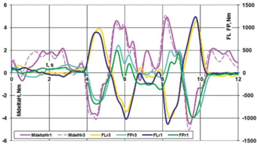
Fig. 6. Comparison of forces in the steering rods at two extreme values of the pivot point radius - standard (r1) and maximum (r3). The drive through the roadside at a speed of 50 km/h and the switched on supporting device. FLr1, FPr1 - forces in rods with Mdel-taHr1, MdeltaHr2 - rotation torque on the driving wheel with the maximum pivot point radius, FLr3, FPr3 - forces in rods with MdeltaHr3
