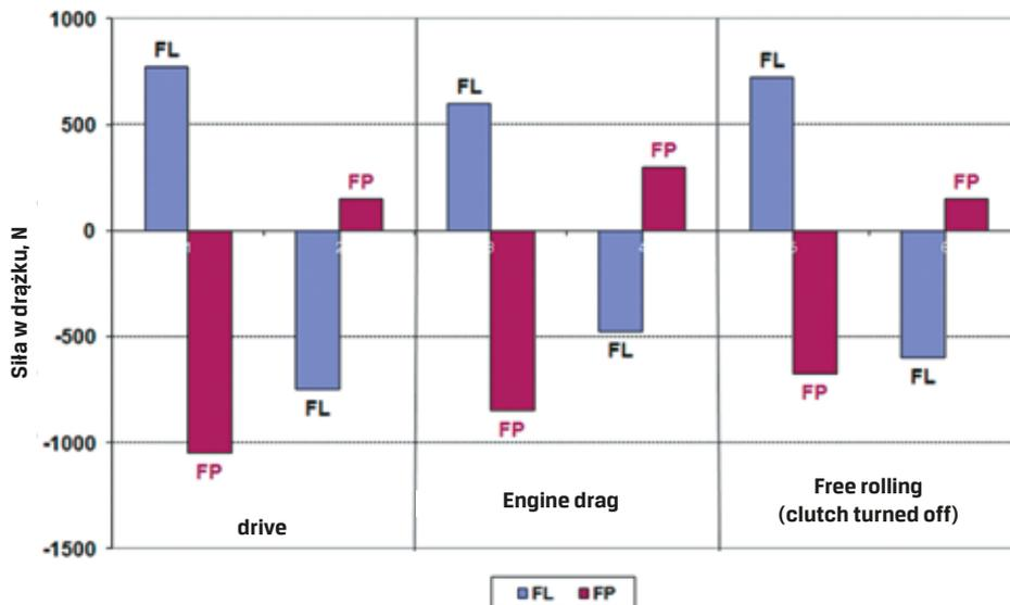
Fig. 7. Forces in the steering rods at various workloads of the tangential forces of front wheels of the car. FDL - force in the left rod, FDP - force in the right rod
