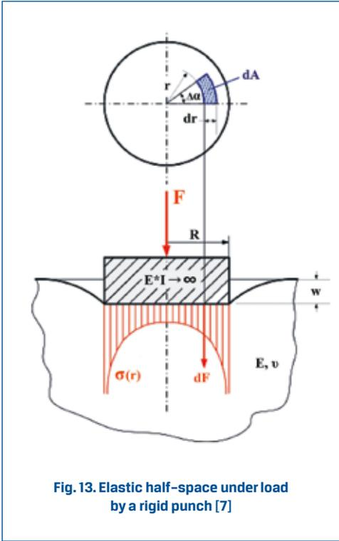
**Fig. 13. Elastic half-space under load by a rigid punch [7]**
