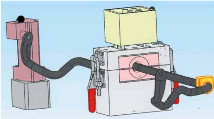
Fig. 6. Device for the vulcanization of flexible bearings (adhesive mounting, Figs. 3 and 4)
