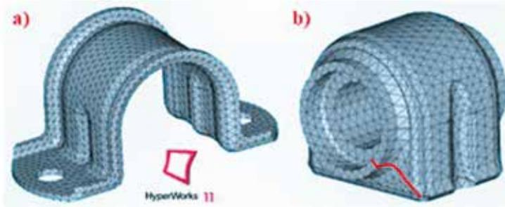
Fig. 10. Computational mesh FEM (HyperMesh) – clamps and flexible bearings of stabilizer bar L405VA
