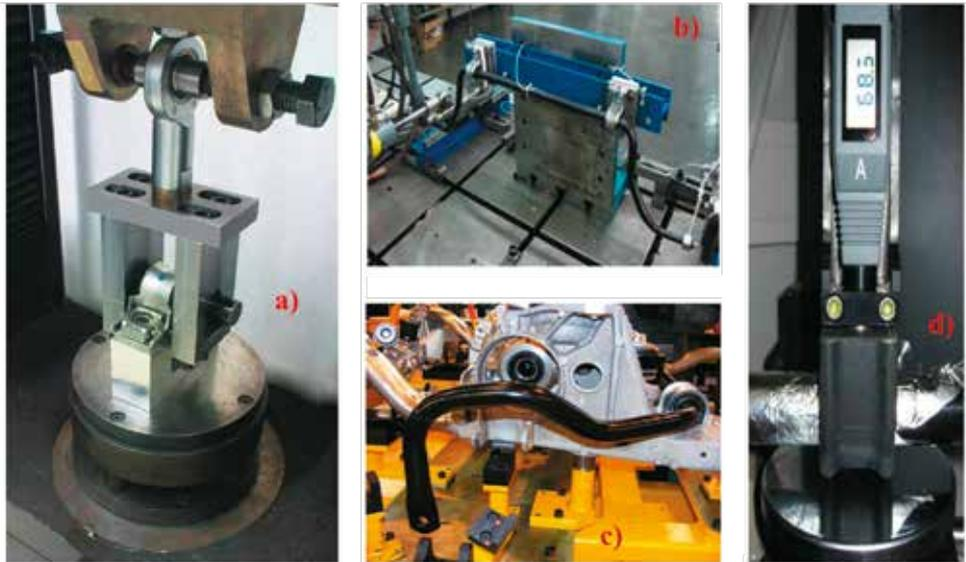
Fig. 14. a) Measuring station for bearing rigidity (source: TKF&S GmbH)
