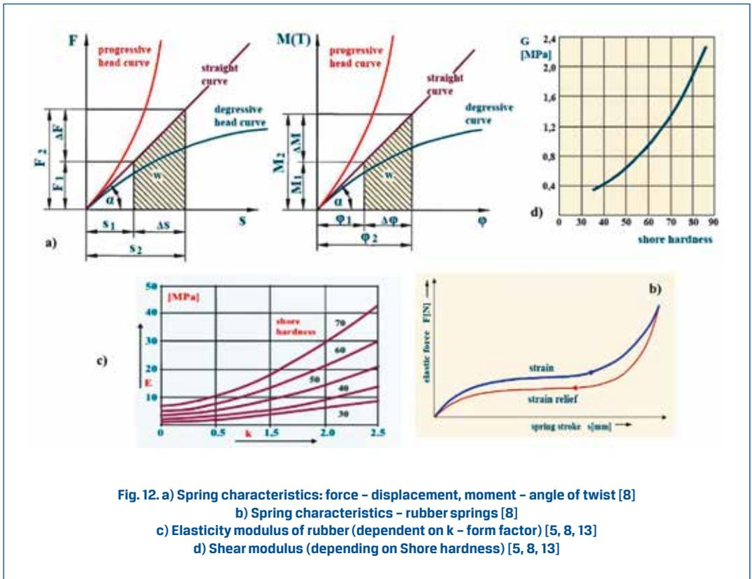
Fig. 12. a) Spring characteristics: force – displacement, moment – angle of twist [8]
