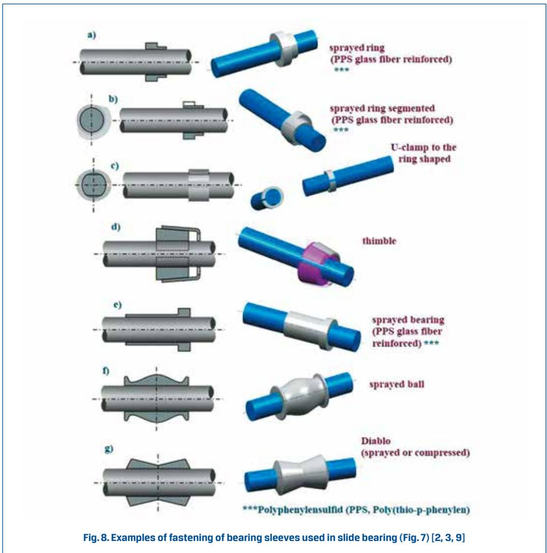
Fig. 8. Examples of fastening of bearing sleeves used in slide bearing (Fig. 7) [2, 3, 9]
