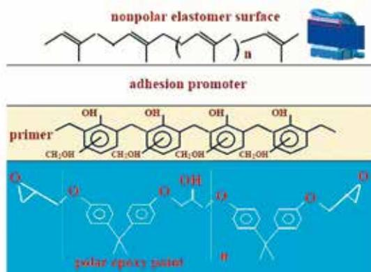
Fig. 3. Chemical process of bearing fastening (adhesive mounting) [9]
