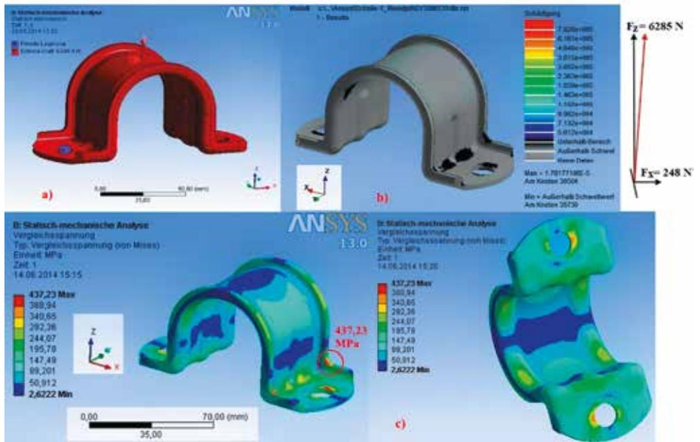
Fig. 11. Strength computations FEM of the clamp and flexible bearing of stabilizer bar L405VA
