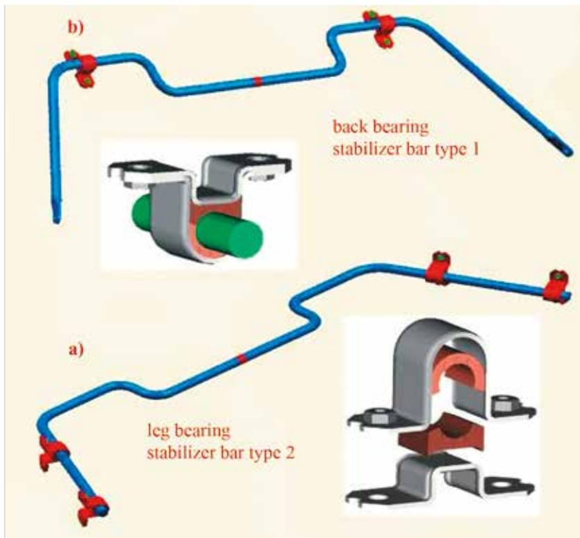
Fig. 1. Bearing arrangement of a stabilizer for a vehicle [2, 3, 9]
