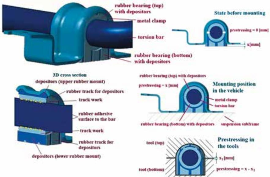
Fig. 5. Device for the vulcanization of flexible bearings (adhesive mounting, Figs. 3 and 4) [2, 3, 9]
