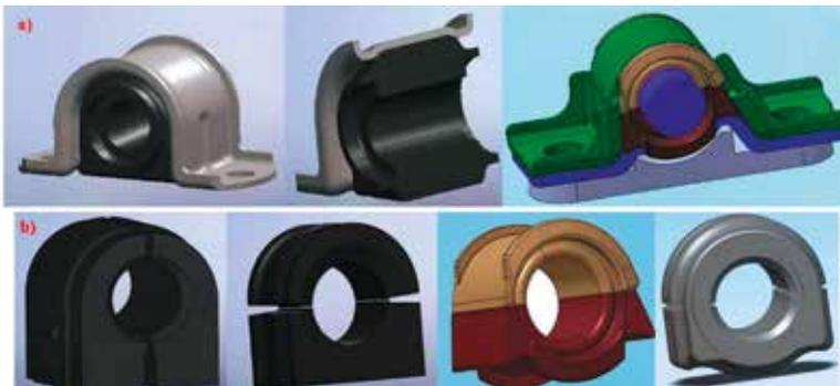
Fig. 4. a) Example of stabilizer bar mounting - adhesive mounting
