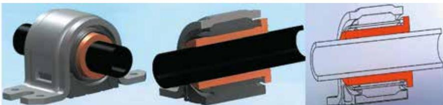
Fig. 7. Example of stabilizer bar mounting – slide bearing
