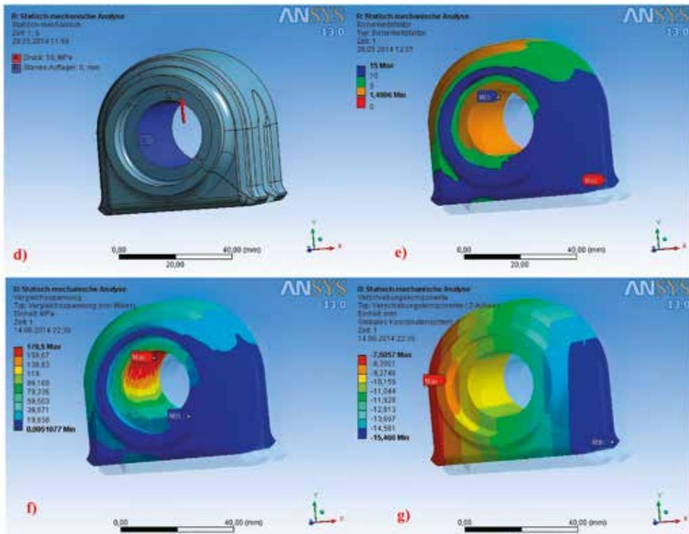
Fig. 11. Strength computations FEM of the clamp and flexible bearing of stabilizer bar L405VA, cont.
