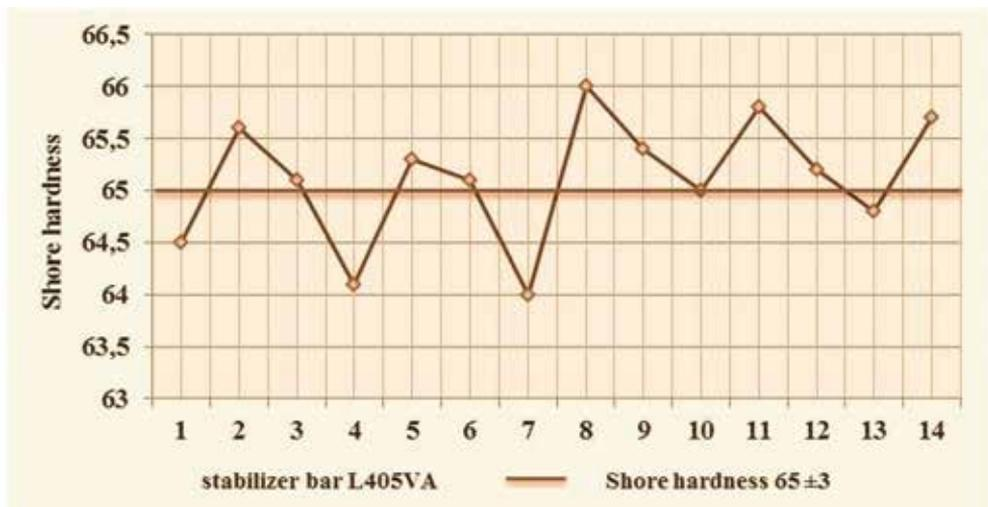
Rys. 15. Shore hardness measurement of flexible bearing of stabilizer bar L405VA on the stand shown in Fig. 14
