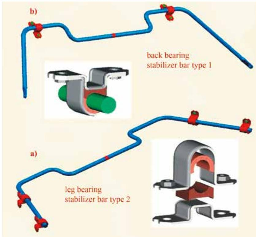
Fig. 1. Bearing arrangement of a stabilizer for a vehicle [2, 3, 9]
