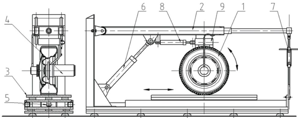
**Fig. 2. Test rig for the investigation of static and dynamic properties of tyres: 1 - wheel with the tyre under investigation; 2 - frame; 3 - plate simulating the test road surface, enabling the measurements of reaction components; 4 - hydraulic motor propelling the wheel (1); 5 - hydraulic cylinder propelling the plate (3); 6, 7 - hydraulic cylinder and turnbuckle screw for vertical loading and unloading the wheel (1); 8, 9 - hydraulic cylinder and module for steering the wheel (1)**
