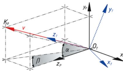
**Fig. 5. Representation of the orientation of vector  $v$  relative to the stationary coordinate system  $x_p, y_p, z_p$  (attached to the transducer base), with the use of angles  $\alpha$  and  $\beta$  between the projections of vector  $v$  on planes  $y_p, z_p$  and  $x_p, z_p$ , respectively, and axis  $z_p$ .**
