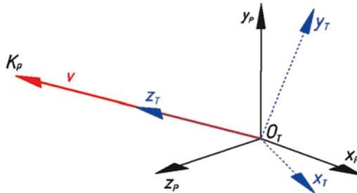
**Fig. 4. Mathematical model of the main linkage of the multiple-sensor 3D tyre deformation transducer:**
