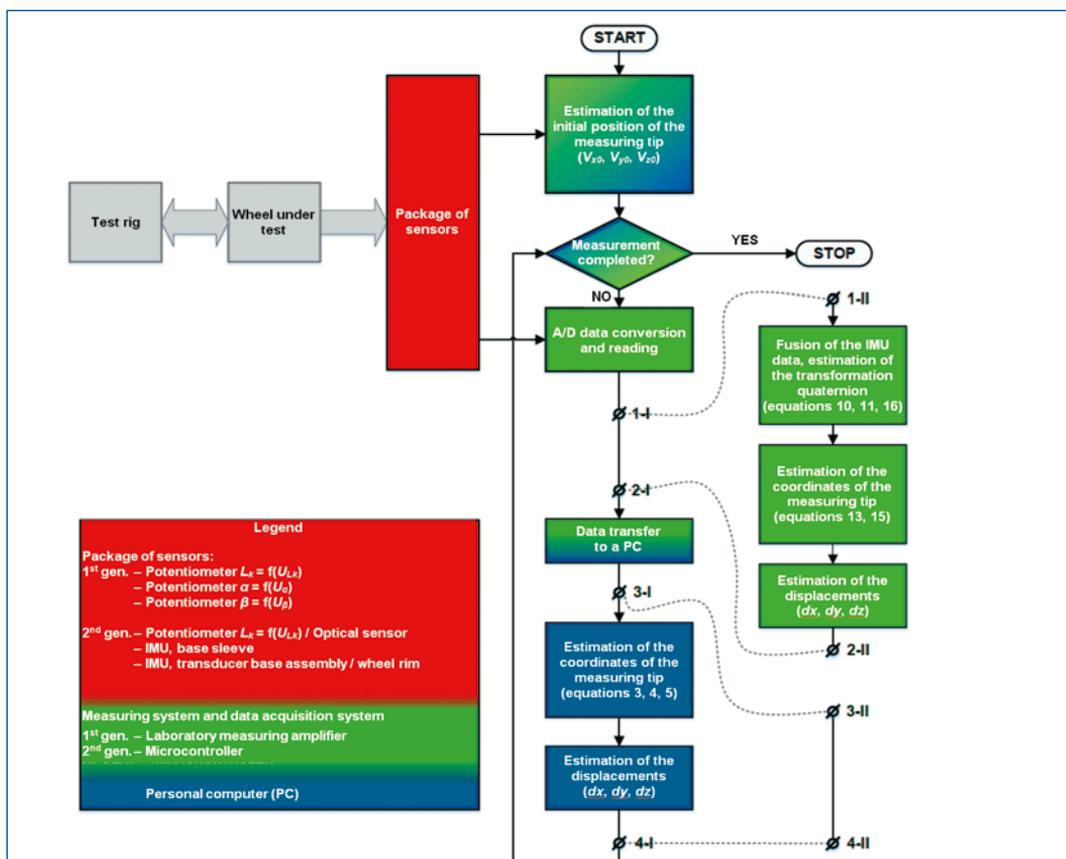
**Fig. 12. Generalized block diagram of the algorithm of operation of a multiple-sensor 3D tyre deformation transducer, showing the differences between the algorithms implemented by the transducers of the first and second generation:**
