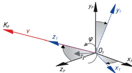
**Fig. 6. Representation of the orientation of vector  $\mathbf{v}$  relative to the  $x_P, y_P, z_P$  coordinate system, using unit quaternions:  $\varphi$  – value of the angle of rotation of the  $P$  reference frame around the unit vector  ${}^P r$ , needed for the corresponding axes of the  $P$  and  $T$  reference frames to coincide, after [15]**
