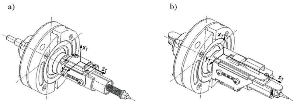
**Fig.9. Multiple-sensor 3D tyre deformation transducer of the second generation: a) option with a potentiometric displacement sensor; b) option with an optic displacement encoder**
