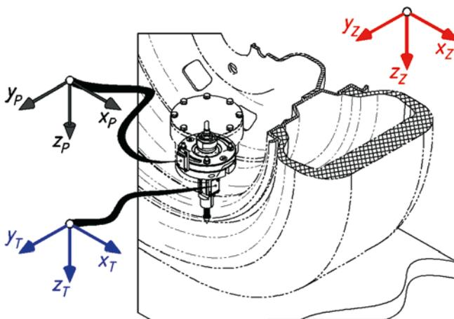
**Fig. 11. Multiple-sensor 3D tyre deformation transducer of the second generation: arrangement of the IMU modules used for determining the parameters of the unit quaternion that describes the mutual orientation between the base sleeve and the transducer base (i.e. the wheel rim)**
