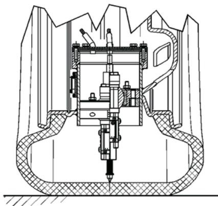
**Fig. 10. Multiple-sensor 3D tyre deformation transducer of the second generation: adjustable positioning of the transducer probe centre of rotation by changing the position of the datum-setting part of the transducer base**
