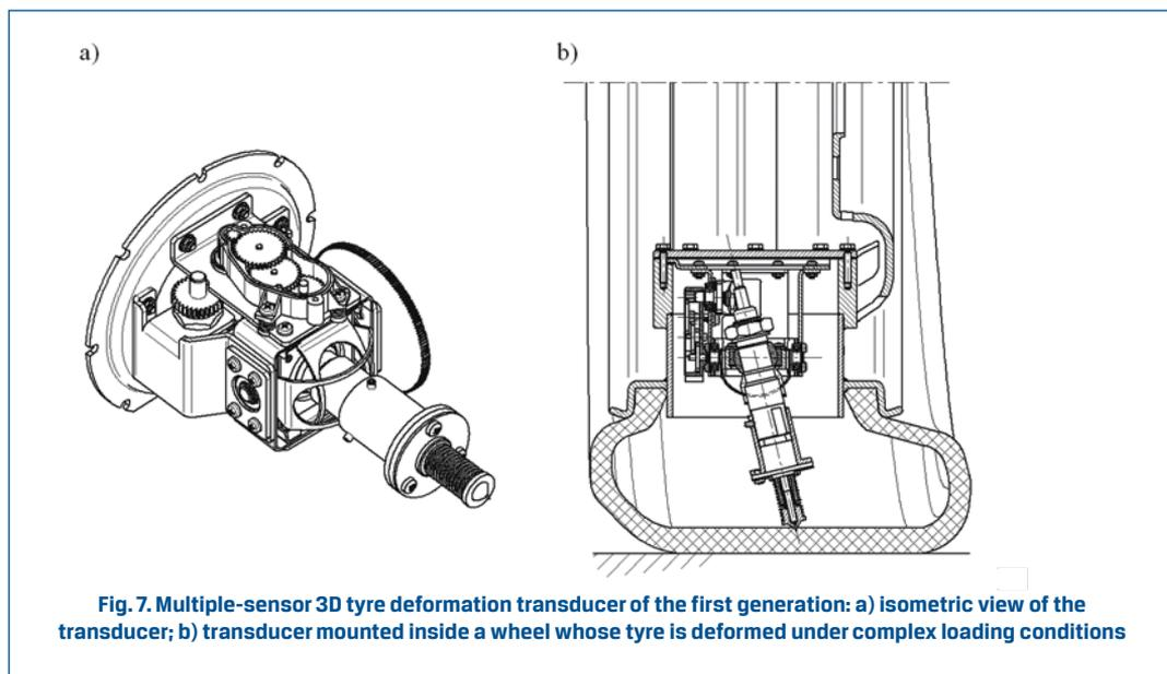
**Fig. 7. Multiple-sensor 3D tyre deformation transducer of the first generation: a) isometric view of the transducer; b) transducer mounted inside a wheel whose tyre is deformed under complex loading conditions**
