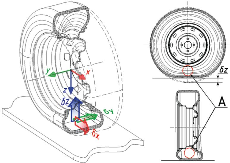
**Fig. 1. Illustration of the design basis against the background of a road wheel in the tyre deformation conditions:  $x, y, z$  - coordinate system attached to the rim as a reference frame for the tyre deformation measurement;  $\delta x, \delta y, \delta z$  - tangential, lateral and radial component of the tyre deformation, respectively; A - location of the multiple-sensor 3D tyre deformation transducer assembly**
