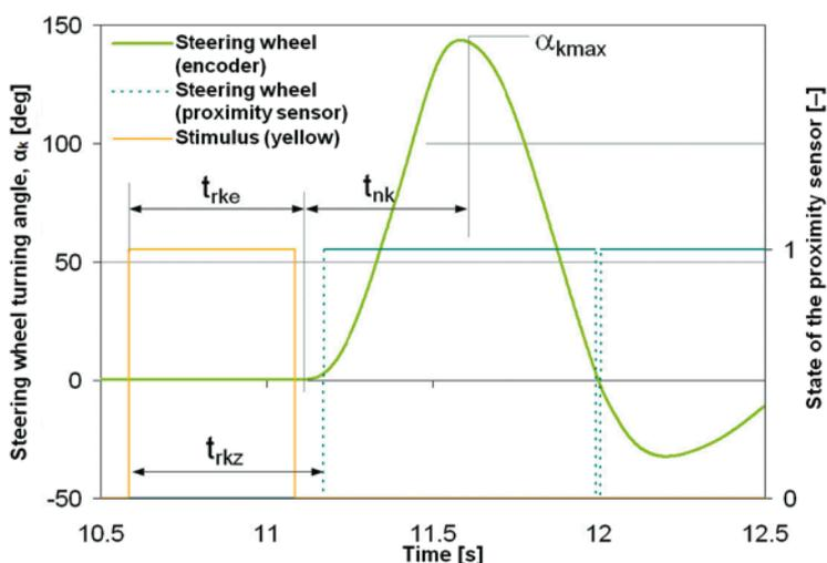
Fig. 6. Parameters of a driver's action on the steering wheel
