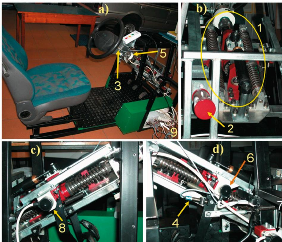
**Fig. 2. Views of the "autoPW T" test machine with its covering panels having been removed; a) - general view; b) - front view; c) - left-side view; d) - right-side view: 1 - steering wheel resistance mechanism; 2 - brake pedal resistance mechanism; 3, 4 - steering wheel and brake pedal proximity sensors; 5, 6, 7, 8 - rotational-impulse sensors (encoders) of steering wheel, brake pedal, accelerator pedal, and clutch pedal positions; 9 - box with a matching and adjustment system**
