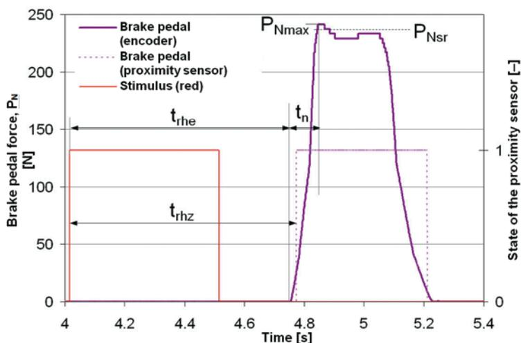
Fig. 5. Parameters of a driver's action on the brake pedal
