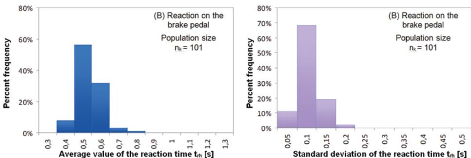
**Fig. 8. Test B. Time of driver reaction on the brake pedal: histograms of the average value (left) and standard deviation (right)**
