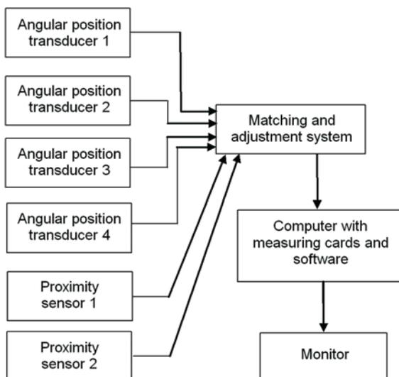
**Fig. 3. Schematic diagram of the measuring system of the "autoPW T" test machine**
