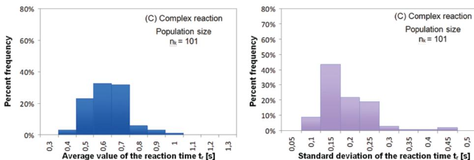
**Fig. 10. Test D. Time of driver reaction on the brake pedal (at "emergency braking"): histograms of the average value (left) and standard deviation (right)**
