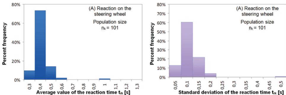
**Fig. 7. Test A. Time of driver reaction on the steering wheel: histograms of the average value (left) and standard deviation (right)**
