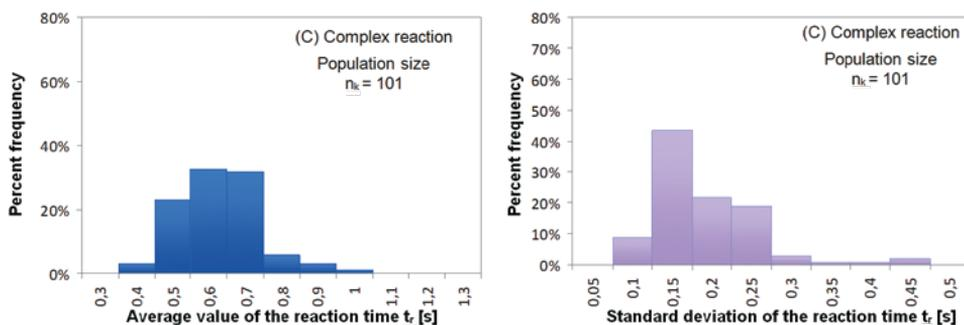
**Fig. 9. Test C. Time of complex driver reaction: histograms of the average value (left) and standard deviation (right)**
