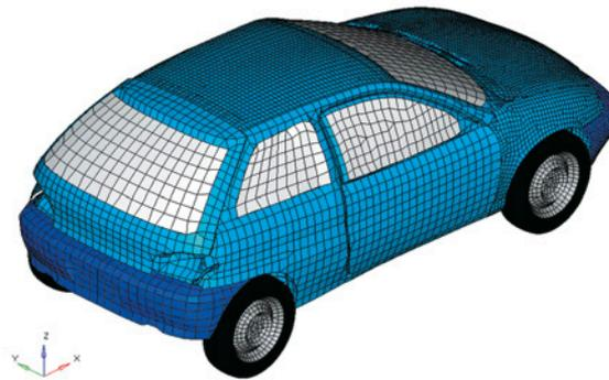
**Fig. 8. Geo Metro car model - isometric view from top [31]**
