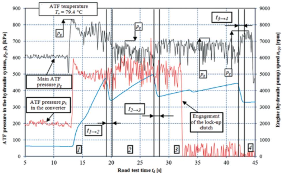
**Fig. 7. Values of ATF pressures  $p_g$  and  $p_k$  in the hydraulic system and of engine (hydraulic pump) speed  $n_{s(p)}$  vs. time  $t_d$  of the maximum vehicle acceleration test (with maximum displacement of the accelerator pedal), with the gearshift time  $t_{i \rightarrow i+1}$  being also shown in the graph**
