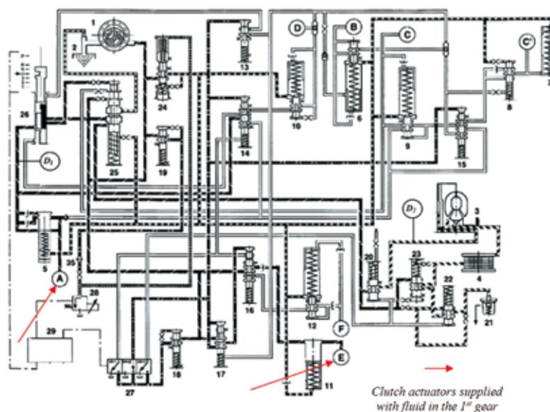
**Fig. 4.** Schematic diagram of the hydraulic control system of the ZF4HP-24 automatic transmission, with the electrohydraulic controller components and ATF flow routes shown for the selector lever set to "D" and the 1<sup>st</sup> gear being implemented: 1 - hydraulic pump; 2 - hydraulic filter; 3 - torque converter; 4 - ATF cooler.
