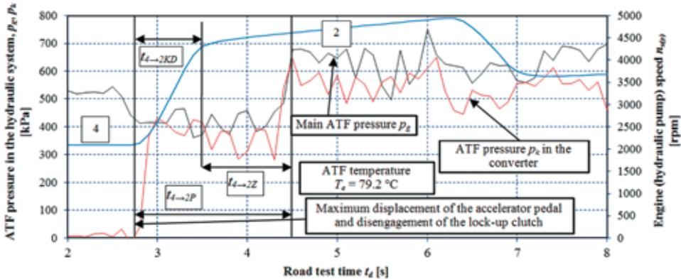
**Fig. 8.** Values of ATF pressures  $p_g$  and  $p_k$  in the hydraulic system and of engine (hydraulic pump) speed  $n_{sp}$  vs. time  $t_d$  of the test with the "kick-down" function being used (when the accelerator pedal is suddenly fully depressed), with the gear-down change time  $t_{4 \rightarrow 2KD}$ , total slippage time  $t_{4 \rightarrow 2P}$  and time lag  $t_{4 \rightarrow 2Z}$  being also shown in the graph
