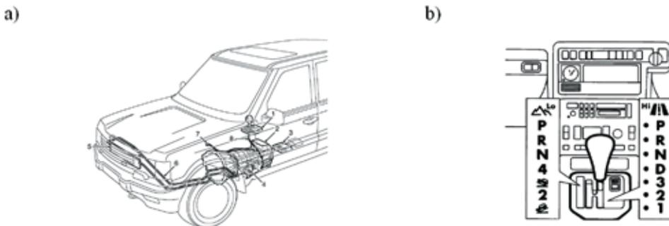
**Fig. 3. The ZF4HP-24 automatic transmission system: a) automatic transmission component layout; b) drive mode selector lever assembly with an "H gate" mechanism;**
