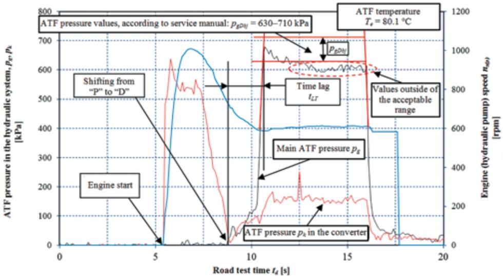
Fig. 9. Values of ATF pressures  $p_g$  and  $p_k$  in the hydraulic system and of engine (hydraulic pump) speed  $n_{s(p)}$  vs. time  $t_d$  of the test on the vehicle being stationary
