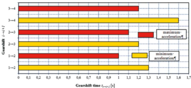
Fig. 6. Values of the gearshift time  $t_{i \rightarrow j}$  during the minimum and maximum vehicle acceleration tests
