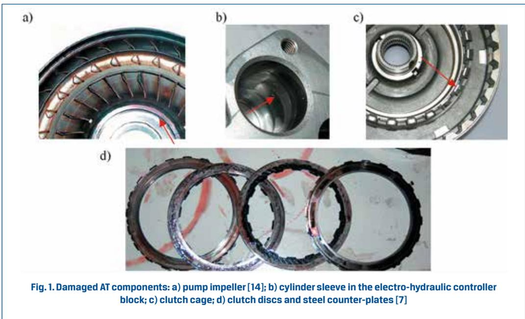
**Fig. 1. Damaged AT components: a) pump impeller [14]; b) cylinder sleeve in the electro-hydraulic controller block; c) clutch cage; d) clutch discs and steel counter-plates [7]**
