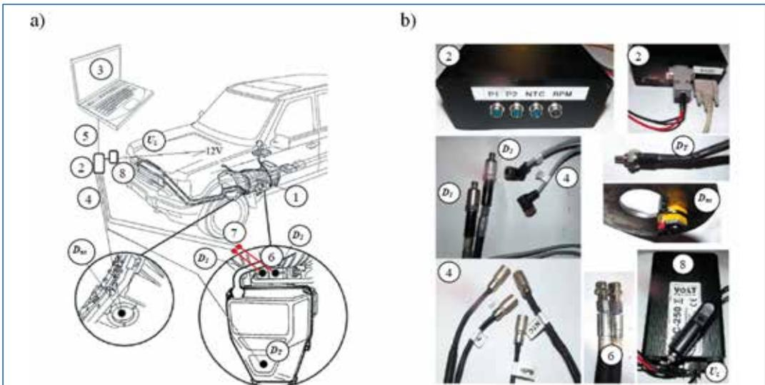
**Fig. 2. Diagnostic system: a) connection diagram; b) view of system components;**
