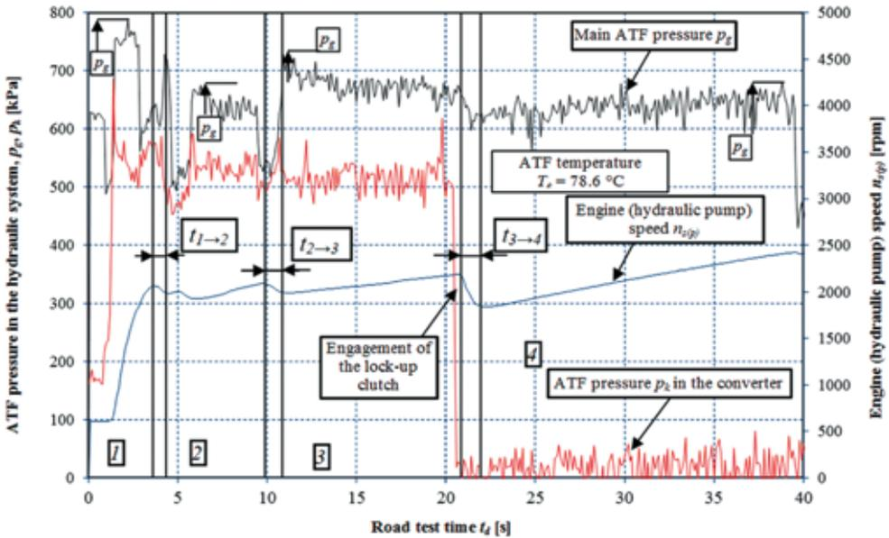
**Fig. 5.** Values of ATF pressures  $p_g$  and  $p_k$  in the hydraulic system and of engine (hydraulic pump) speed  $n_{s(p)}$  vs. time  $t_d$  of the minimum vehicle acceleration test (with minimum displacement of the accelerator pedal), with the gearshift time  $t_{i \rightarrow i+1}$  being also shown in the graph
