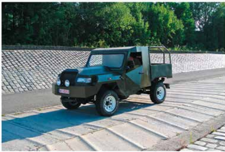
Fig. 2. Test vehicle SOF during coast-down measurements of rolling resistance on a road with sinusoidal profile [8]
