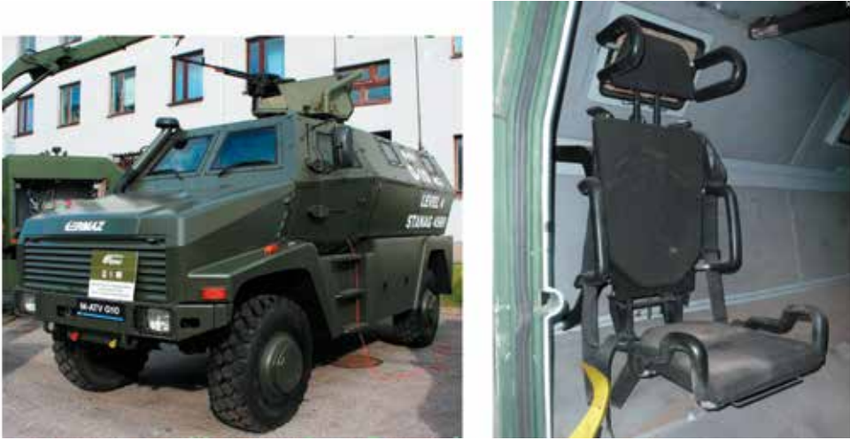
Fig. 12. The mine resistant armored vehicle Germaz G-10 (left) and the prototype of the blast attenuating seat (right)
