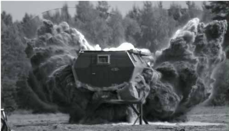
Fig. 13. Full scale blast test of the Germaz G10 mine resistant vehicle.
