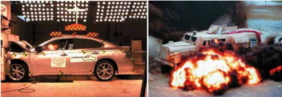
Fig. 1. Crash test of the passenger car (left), full scale blast test of vehicle (right),
