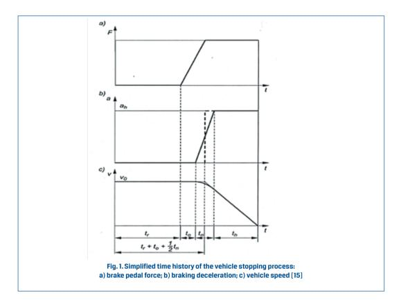
equal to the one with which the vehicle moved when the driver made a decision to apply brakes. The braking process as such actually begins after the end of this period.
