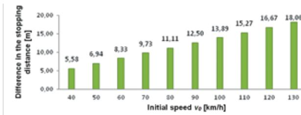
Fig. 5. Differences [m] between the lengths of the stopping distance determined for the driver's perception time values of  $t_{r1} = 0.82$  s and  $t_{r1} = 0.32$  s [9]
