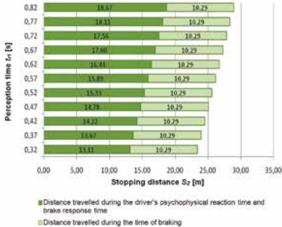
**Fig. 3. Relation between the length of vehicle stopping distance and changes in the driver's perception time, for a single combination of the initial vehicle speed and braking acceleration, i.e.  $v_0 = 40$  km/h and  $a_h = 6$  m/s<sup>2</sup>, respectively [9]**
