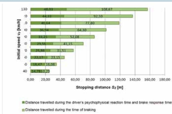
Fig. 4. Relation between the length of vehicle stopping distance and initial vehicle speed  $v_0$  at a constant average driver's perception time and a constant deceleration [9]
