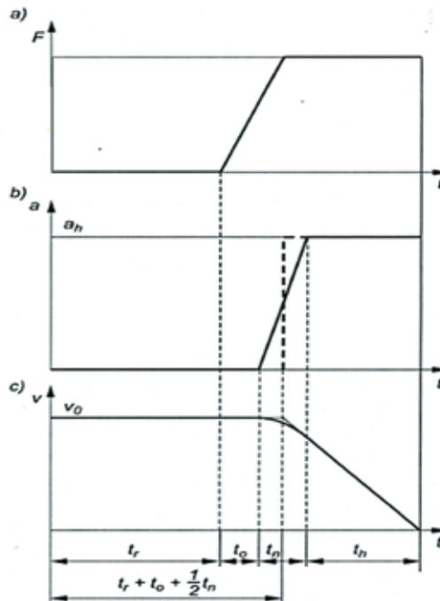
**Fig. 1. Simplified time history of the vehicle stopping process:**
