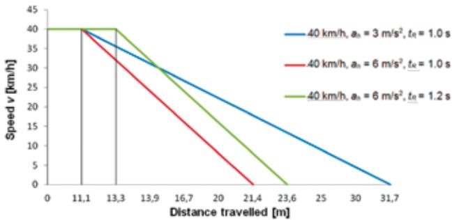
**Fig. 8. Stopping distance at an initial speed of 40 km/h, depending on the reaction time and braking deceleration [9]**
