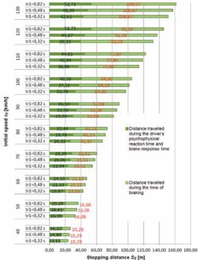
Fig. 2. Changes in the length of vehicle stopping distance depending on vehicle speed  $v_0$  for different values of the perception time (i.e. for  $t_{r1} = 0.32$  s,  $t_{r1} = 0.48$  s, and  $t_{r1} = 0.82$  s), at  $a_h = 6$  m/s<sup>2</sup> [9]
