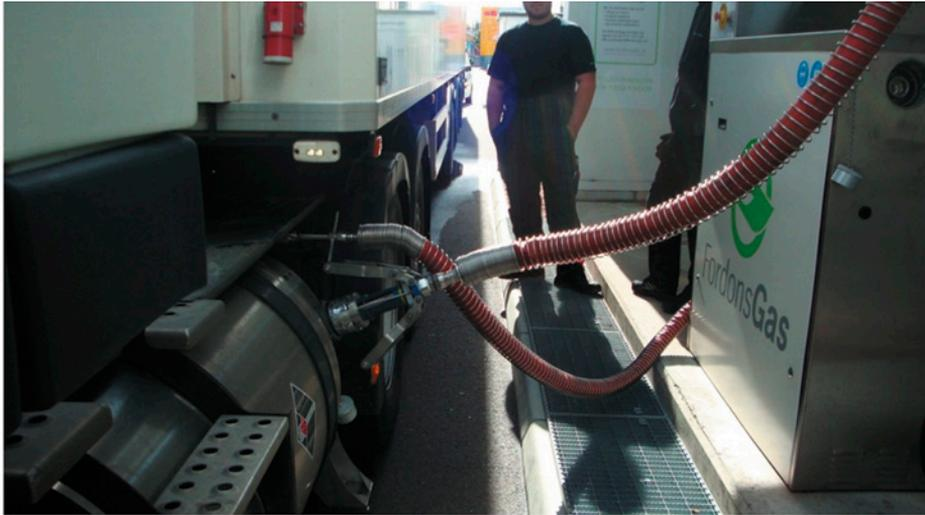
**Fig. 4. Volvo LNG/biomethane truck at filling station, Göteborg**
