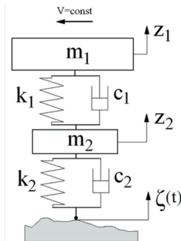
Fig. 2. Quarter-car model (for the notation used, see the text)
