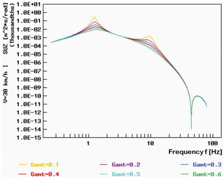
Fig. 12. Power spectral densities of suspension deflection (denoted by SUZ in the graph, see the element of integration in equation (16)) vs. excitation frequency  $f$ , for various values of the coefficient of relative damping (see (22), denoted by  $G_{ant}$  in the graph), for the road of class C (i.e. of average quality) according to the ISO standard [8], and for a vehicle speed of  $V = 30$  [km/h]
