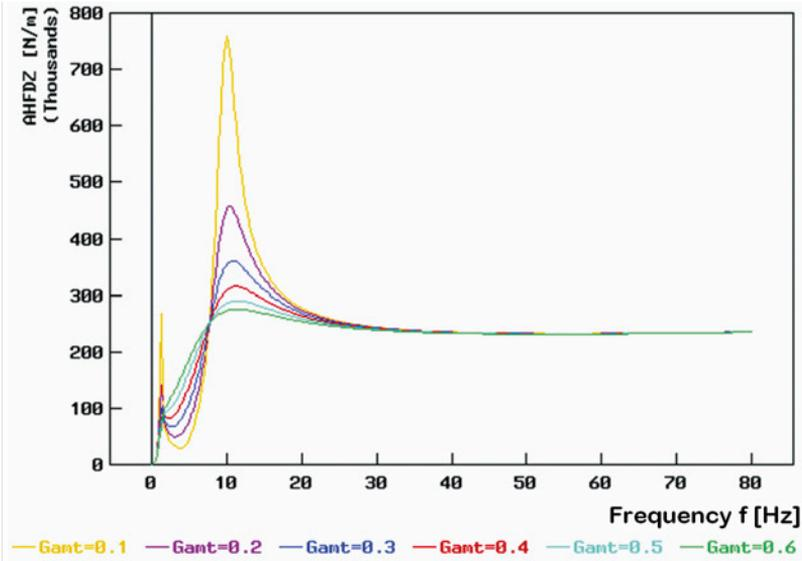
Fig. 6. Absolute value of the spectral transmittance for the dynamic component of the normal reaction at the tyre/road contact (see (17) and (20), denoted by AHFDZ in the graph) vs. excitation frequency  $f$ , for various values of the relative damping coefficient (see (22), denoted by  $G_{ant}$  in the graph)
