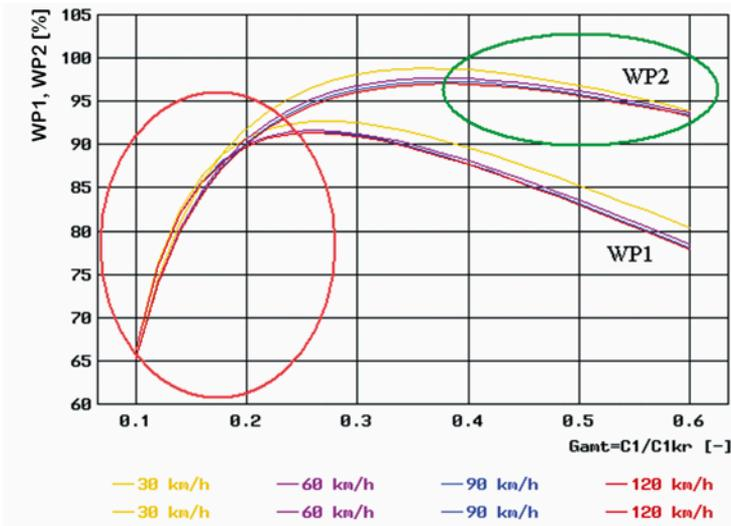
Fig. 20. Comfort indicator WP1 (see (30)) and safety indicator WP2 (see (31)) vs. the relative damping coefficient (see (22), denoted by  $G_{ant}$  in the graph), for the road of class C (i.e. of average quality) according to the ISO standard [8] and for 4 vehicle speed values ranging from 30 km/h to 120 km/h
