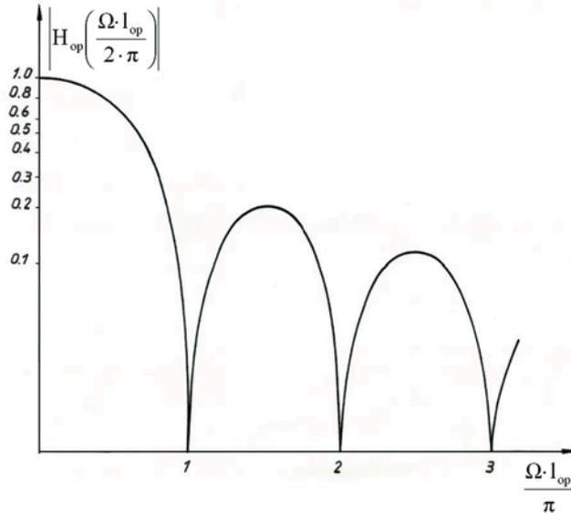
Fig. 4. Absolute value of the transmittance of a filter describing the smoothing properties of vehicle tyres, corresponding to the "constant patch model" [14] (for the notation used, see the text)
