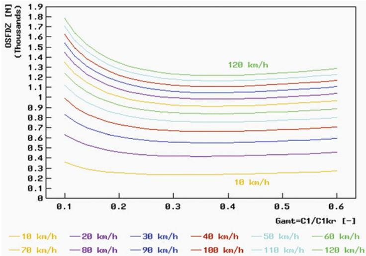
Fig. 14. Standard deviations of the dynamic component of the normal reaction at the tyre/road contact (see (15), denoted by OSFDZ in the graph) vs. the relative damping coefficient (see (22), denoted by  $G_{amt}$  in the graph), for the road of class C (i.e. of average quality) according to the ISO standard [8] and for 12 vehicle speed values ranging from 10 km/h to 120 km/h
