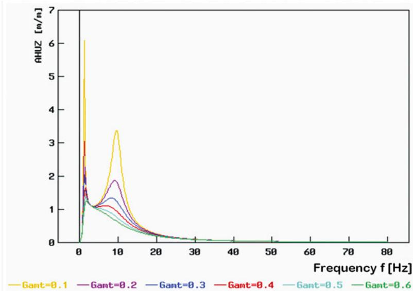
Fig. 7. Absolute value of the spectral transmittance for suspension deflection (see (18) and (21), denoted by AHUZ in the graph) vs. excitation frequency  $f$ , for various values of the relative damping coefficient (see (22), denoted by  $G_{ant}$  in the graph)
