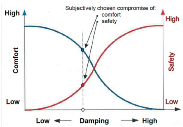
**Fig. 1. Pictorial illustration of seeking a compromise between the comfort and safety requirements at the selection of constant damping in the suspension system [30]**
