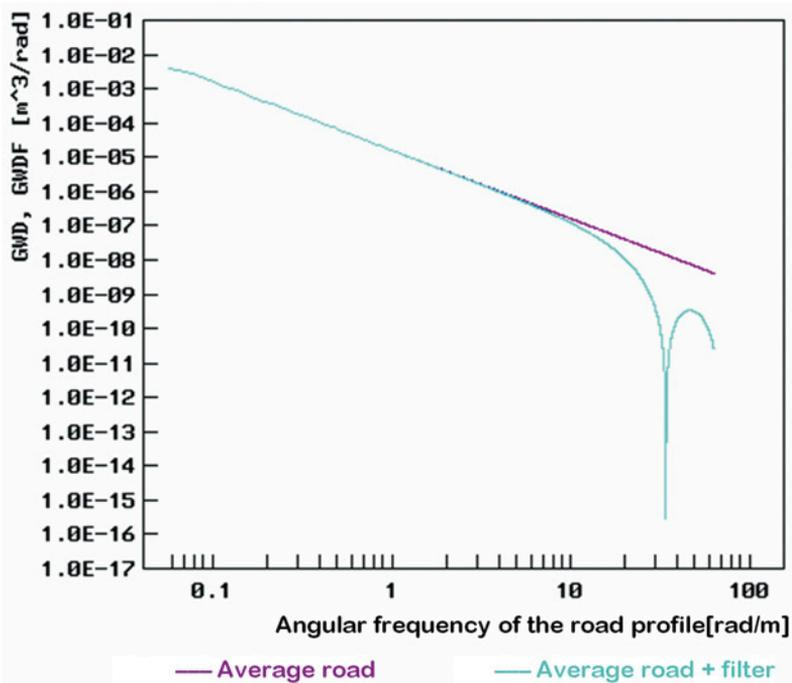
Fig. 8. Power spectral density of road surface irregularities (see (9), denoted by GWD in the graph, dark purple curve) and the effect of filtration (denoted by GWDF), obtained with the use of a "constant patch model" of the pneumatic tyre (aquamarine curve), vs. angular frequency of the road profile, for the road of class C (i.e. of average quality) according to the ISO standard [8]
