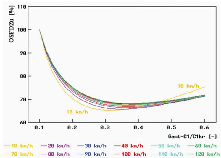
Fig. 17. Normalized standard deviations of the dynamic component of the normal reaction at the tyre/road contact (see (29), denoted by OSFDZu in the graph) vs. the relative damping coefficient (see (22), denoted by  $G_{amt}$  in the graph), for the road of class C (i.e. of average quality) according to the ISO standard [8] and for 12 vehicle speed values ranging from 10 km/h to 120 km/h
