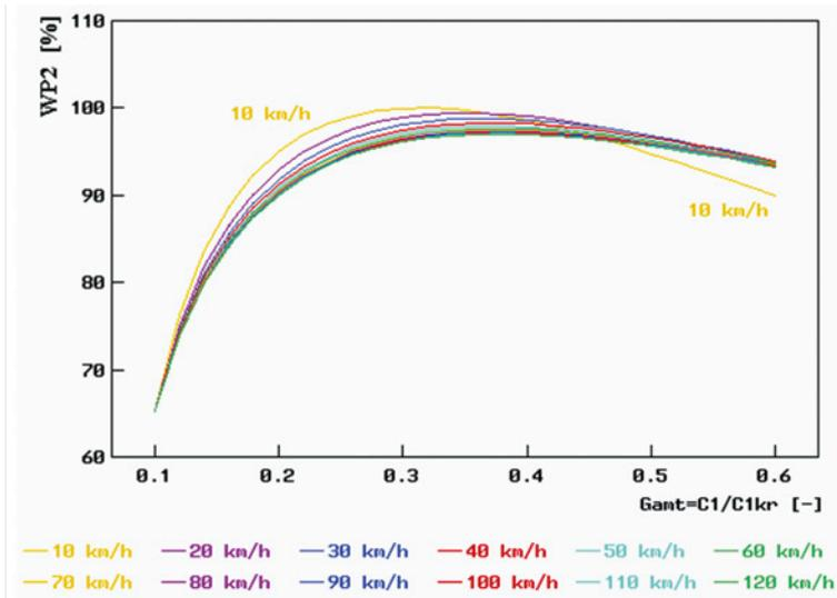
Fig. 19. Safety indicator WP2 (see (31)) vs. the relative damping coefficient (see (22), denoted by  $G_{ant}$  in the graph), for the road of class C (i.e. of average quality) according to the ISO standard [8] and for 12 vehicle speed values ranging from 10 km/h to 120 km/h
