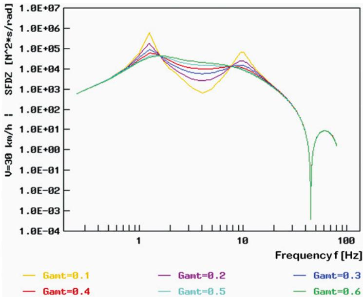
Fig. 11. Power spectral densities of the dynamic component of the normal reaction at the tyre/road contact (denoted by SFDZ in the graph, see the element of integration in equation (15)) vs. excitation frequency  $f$ , for various values of the relative damping coefficient (see (22), denoted by  $G_{ant}$  in the graph), for the road of class C (i.e. of average quality) according to the ISO standard [8], and for a vehicle speed of  $V = 30$  [km/h]
