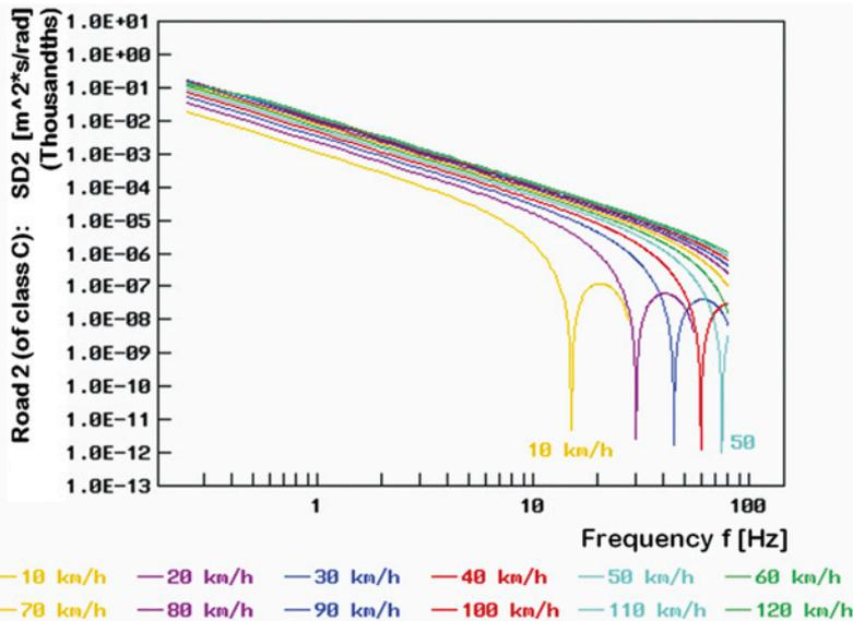
**Fig. 9. Power spectral densities of road surface irregularities  $S_{df}(\omega)$  (denoted by SD2 in the graph) vs. the radian frequency  $\omega$  [rad/s], presented as Hertz frequency  $f$  [Hz] of the excitation (for easier comparisons with other graphs), for the road of class C (i.e. of average quality) according to the ISO standard [8] and for various vehicle speeds  $V$  [km/h]**
