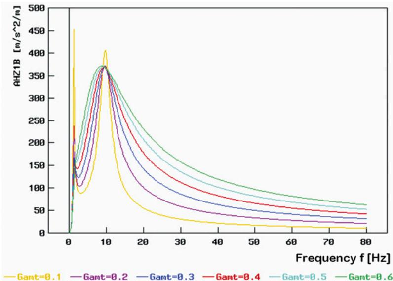
**Fig. 5. Absolute value of the spectral transmittance for sprung mass acceleration (see (8) and (19), denoted by AHZ1B in the graph) vs. excitation frequency  $f$ , for various values of the relative damping coefficient (see (22), denoted by  $G_{ant}$  in the graph)**
