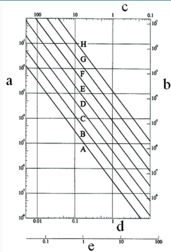
**Fig. 3. Power spectral density values of random road surface irregularities according to the ISO classification [8]; road classes from A to H; log-log scale. Meaning of the lowercase letters in the drawing: a – power spectral density  $S_d(1/L)$  [ $m^2$ ]; b – power spectral density  $S_d(\Omega)$  [ $m^2/rad$ ]; c – wavelength  $L$  [ $m$ ]; d – wave number  $1/L$  [ $1/m$ ]; e – angular frequency of the longitudinal road profile  $\Omega = 2\pi/L$  [ $rad/m$ ]**
