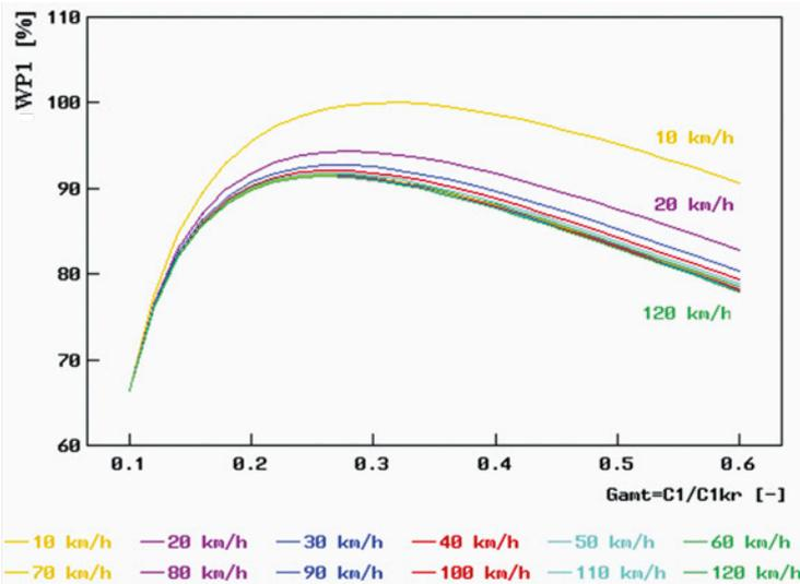
**Fig. 18. Comfort indicator WP1 (see (30)) vs. the relative damping coefficient (see (22), denoted by  $G_{amt}$  in the graph), for the road of class C (i.e. of average quality) according to the ISO standard [8] and for 12 vehicle speed values ranging from 10 km/h to 120 km/h**
