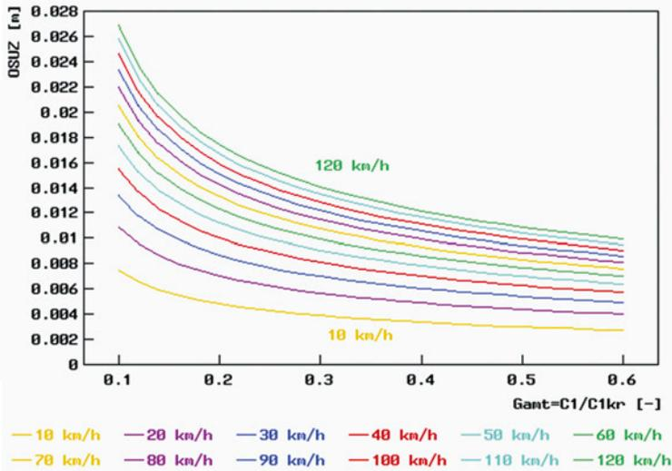
**Fig. 15. Standard deviations of suspension deflection (see (16), denoted by OSUZ in the graph) vs. the relative damping coefficient (see (22), denoted by Gamt in the graph), for the road of class C (i.e. of average quality) according to the ISO standard [8] and for 12 vehicle speed values ranging from 10 km/h to 120 km/h**
