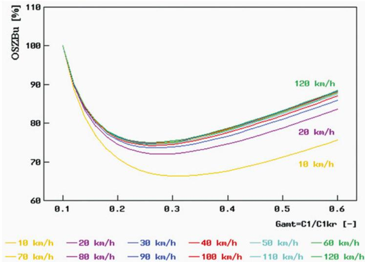
Fig. 16. Normalized standard deviations of sprung mass accelerations (see (28), denoted by OSZBu in the graph) vs. the relative damping coefficient (see (22), denoted by  $G_{amt}$  in the graph), for the road of class C (i.e. of average quality) according to the ISO standard [8] and for 12 vehicle speed values ranging from 10 km/h to 120 km/h
