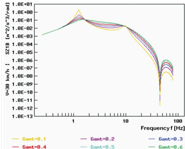
**Fig. 10.** Power spectral densities of sprung mass accelerations (denoted by SZ1B in the graph, see the element of integration in equation (14)) vs. excitation frequency  $f$ , for various values of the relative damping coefficient (see (22), denoted by  $G_{ant}$  in the graph), for the road of class C (i.e. of average quality) according to the ISO standard [8], and for a vehicle speed of  $V = 30$  [km/h]
