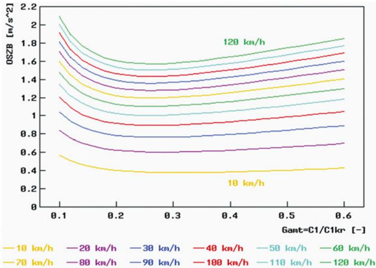
Fig. 13. Standard deviations of sprung mass accelerations (see (14), denoted by OSZB in the graph) vs. the relative damping coefficient (see (22), denoted by  $G_{amt}$  in the graph), for the road of class C (i.e. of average quality) according to the ISO standard [8] and for 12 vehicle speed values ranging from 10 km/h to 120 km/h
