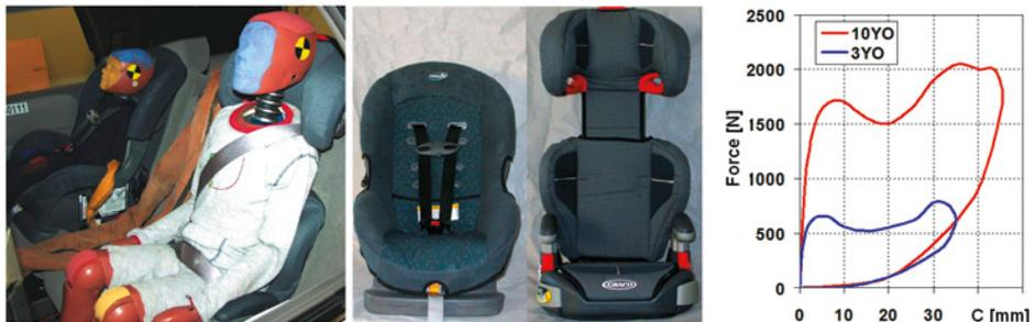
**Fig. 4. The child safety seat and cushion seat used for restraining the test dummies during the crash tests and the characteristic curves representing the dynamic thoracic deflection of the dummies [15, 16]**
