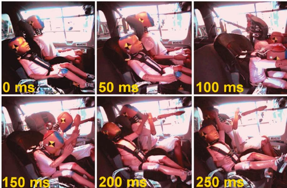
Fig. 6. Dummies' displacements during the collision in test V1 (based on [32])
