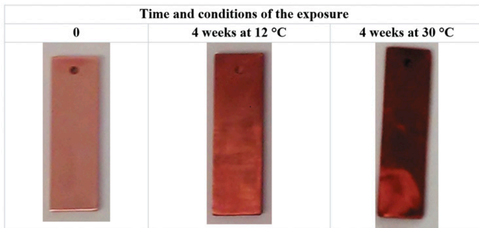
Fig. 3. The appearance of the copper plates before and after the exposure to contact with the diesel oil
