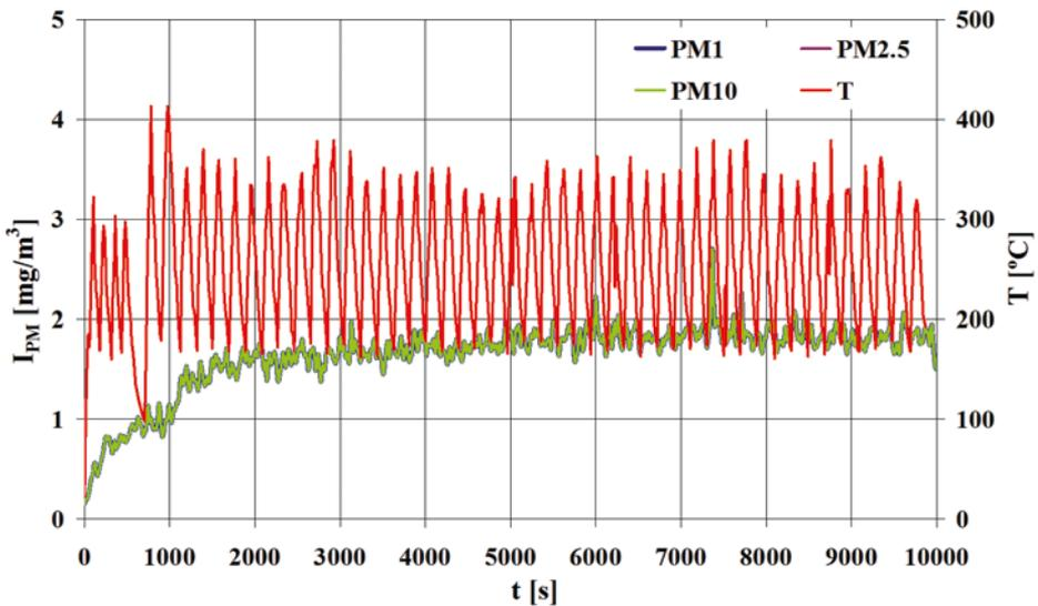
Fig. 4. Time histories of the immissions of specific particulate matter size fractions ( $I_{PM}$ ) in the measuring room and of the friction surface temperature (T) for the friction pair with ceramic brake pads (the second series of measurements)
