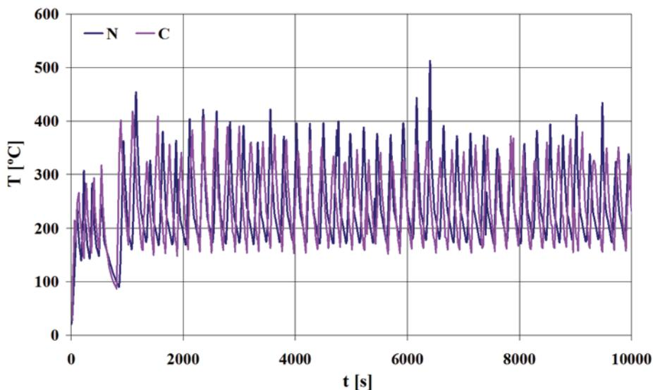
Fig. 8. Comparison between the temperature (T) vs. time (t) curves plotted for the brake disc's friction surface for the friction pairs with conventional and ceramic brake pads (the second series of measurements)
