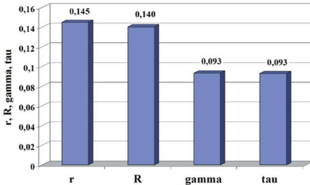
Fig. 10. Coefficients of Pearson, Spearman, Kruskal gamma, and Kendall tau correlation ( $r$ ,  $R$ ,  $\gamma$ , and  $\tau$ , respectively) between the TSP dust immission in the measuring room ( $I_{TSP}$ ) and the temperature ( $T$ ) of the brake disc's friction surface for the friction pair with conventional brake pads in the third series of measurements
