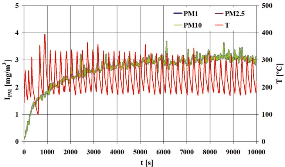
Fig. 2. Time histories of the immissions of specific particulate matter size fractions ( $I_{PM}$ ) in the measuring room and of the friction surface temperature ( $T$ ) for the friction pair with conventional brake pads (the second series of measurements)
