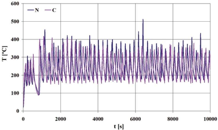
Fig. 7. Comparison between the temperature ( $T$ ) vs. time ( $t$ ) curves plotted for the brake disc's friction surface for the friction pairs with conventional and ceramic brake pads (the first series of measurements)
