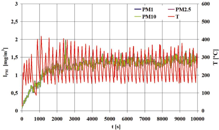
Fig. 3. Time histories of the immissions of specific particulate matter size fractions ( $I_{PM}$ ) in the measuring room and of the friction surface temperature (T) for the friction pair with ceramic brake pads (the first series of measurements)
