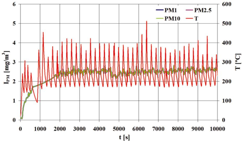
Fig. 1. Time histories of the immissions of specific particulate matter size fractions ( $I_{PM}$ ) in the measuring room and of the friction surface temperature ( $T$ ) for the friction pair with conventional brake pads (the first series of measurements)
