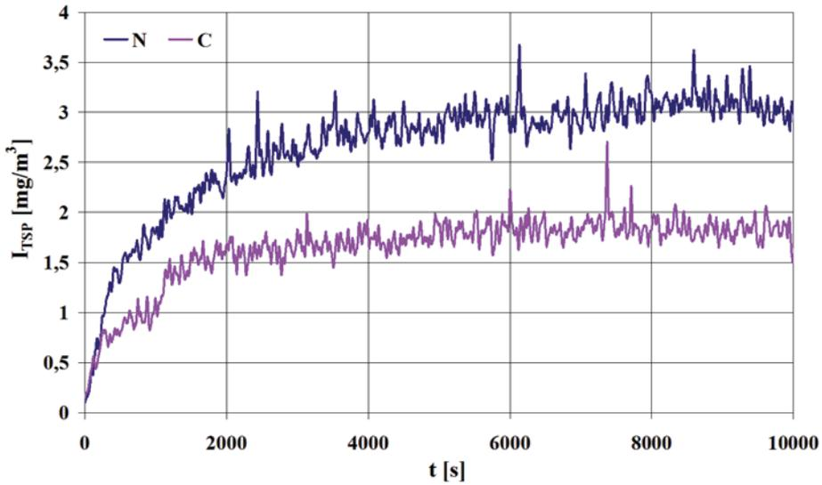
Fig. 6. Comparison between time histories of the TSP dust immission ( $I_{TSP}$ ) recorded for the friction pairs with conventional and ceramic brake pads (the second series of measurements)
