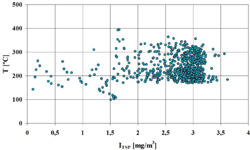
Fig. 9. Correlational interdependence between the TSP dust immission in the measuring room ( $I_{TSP}$ ) and the temperature ( $T$ ) of the brake disc's friction surface for the friction pair with conventional brake pads in the third series of measurements
