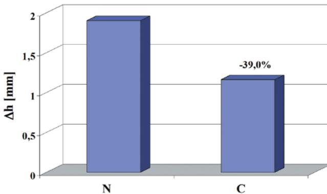
Fig. 12. A reduction in thickness of the friction pairs with conventional (N) and ceramic (C) brake pads
