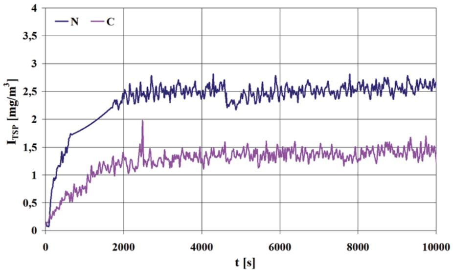
Fig. 5. Comparison between time histories of the TSP dust immission ( $I_{TSP}$ ) recorded for the friction pairs with conventional and ceramic brake pads (the first series of measurements)
