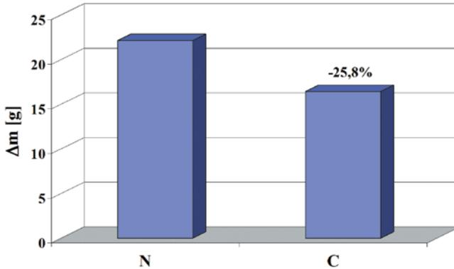
Fig. 11. A reduction in mass of the friction pairs with conventional (N) and ceramic (C) brake pads
