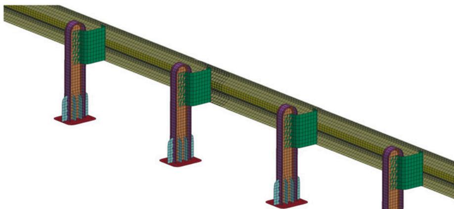
Fig. 4. Back view of the numeric model of the KTC 015 barrier
