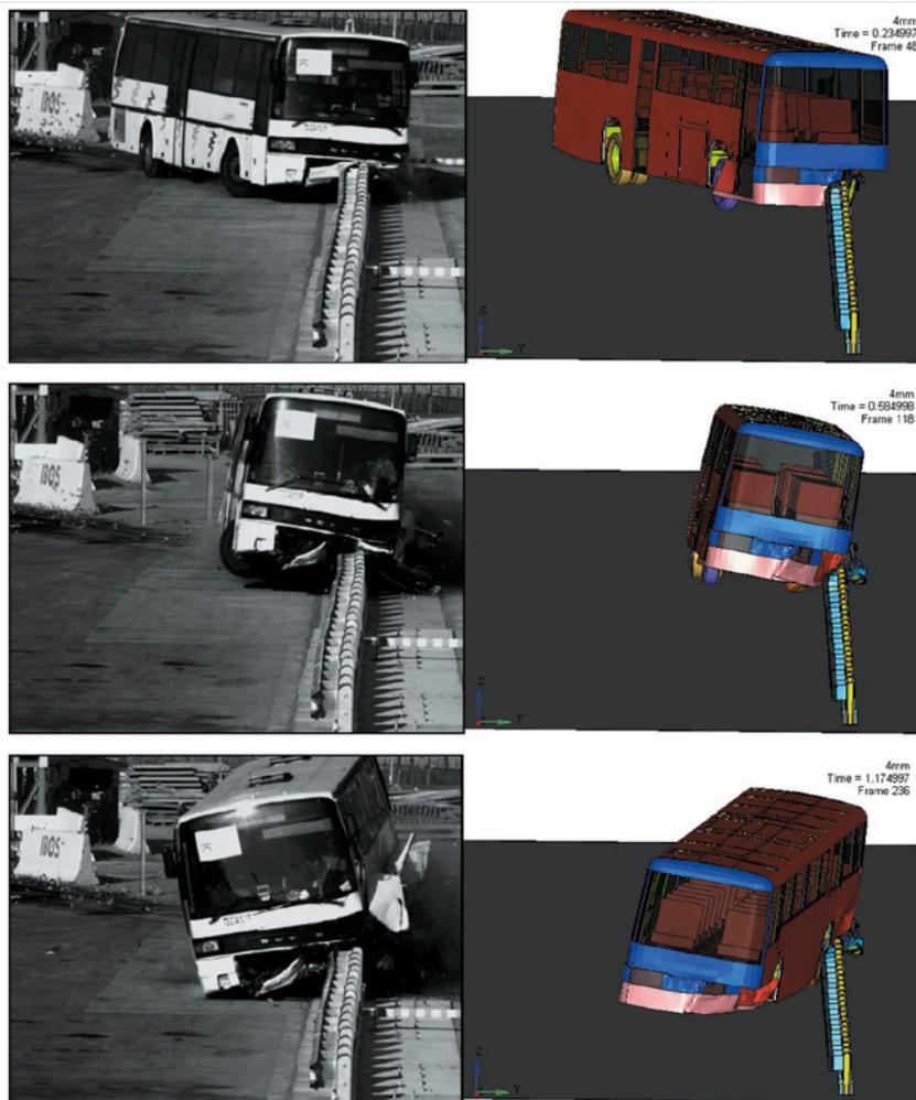
Fig. 7. Deformations of the vehicle-barrier system in selected time points
