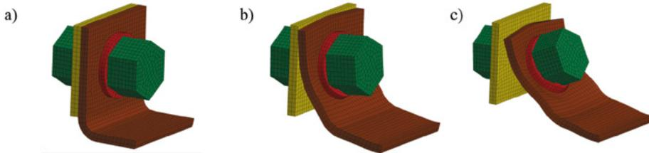
Fig. 5. Absorber-guide bar joint in subsequent load phases until breakage
