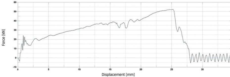
Fig. 6. Course of strength in the displacement function for the absorber-guide bar joint
