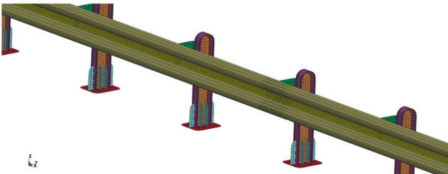
Fig. 3. Front view of the numeric model of the KTC 015 barrier
