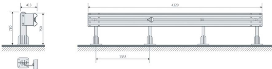
Fig. 2. Dimensions of the repeating fragment of the KTC 015 system [11]
