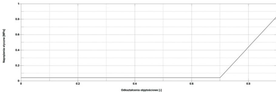
Fig.12. CURVE2. Shear stresses in a function of dilatational strains
