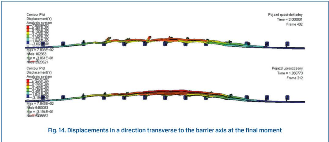
Fig. 14. Displacements in a direction transverse to the barrier axis at the final moment
