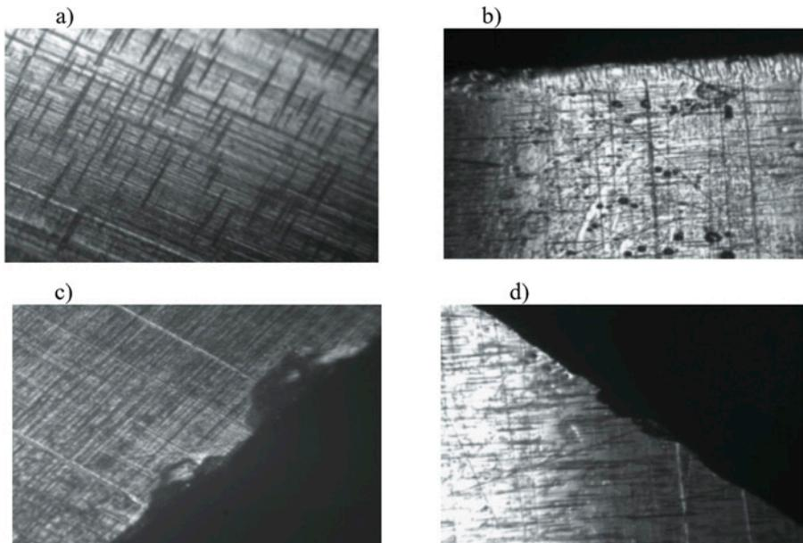
Fig. 27. Image of an injection section piston surface: a) a new piston surface fragment (the grinding traces clearly dominate), b, c, d) the piston surface area after operation (125x zoom) [16]
