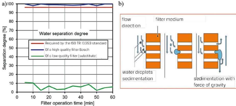
**Fig. 36. Water filtration in the fuel filters in terms of the ISO 13353 requirements:**
