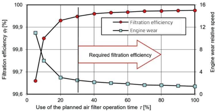
Fig. 17. Filtration efficiency and the engine wear speed in a function of time of air filter operation [14]
