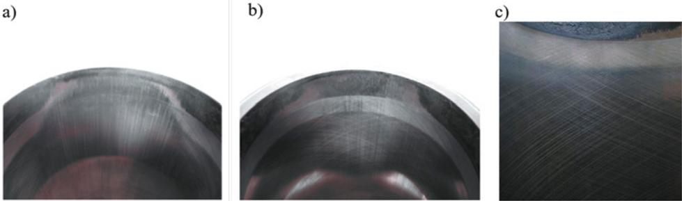
**Fig. 10. View of a truck's engine cylinder bearing surface operated with an operative and inoperative air filtration system:**
