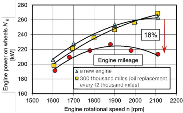
Fig. 23. The Cummins N14 engine power change – the new one and after different vehicle mileages with oil replacement every 12 and 25 thousand miles [11]
