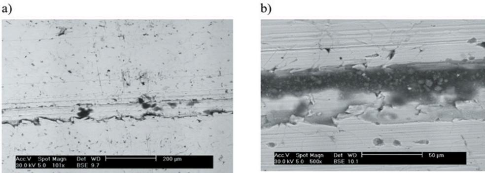
**Fig. 11. Cracks in the cylinder bearing surface caused by dust particles [9]**
