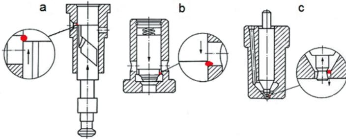
Fig. 26. The manners of the contaminants' entering between plunger and barrel assemblies sealing surfaces: a) in a pumping section, b) in a pressure valve, c) at a washer pivot
