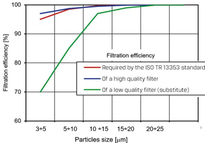
Fig. 33. Filtration efficiency of fuel filters compared to the ISO 13353's requirements [10]
