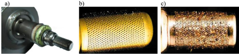
Fig. 32. DRV Bosch Common Rail pressure control valve with a mesh filter (a), new filter view (b), after operation (c) view from a digital microscope [16]
