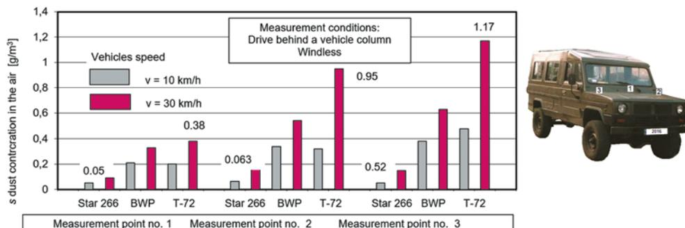
Fig. 4. Dust concentration in the air at the measuring points nos. 1, 2, 3 of an off-road passenger vehicle driving behind the column of: tanks T-72, BWP, Star 266 cars at different speeds [7]
