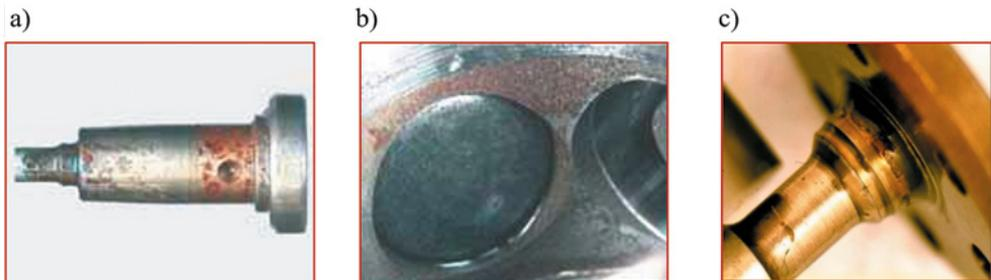
**Fig. 35. Corrosive wear of the injection system components at inadequate water filtration: a) injector element corrosion, b) high pressure pump housing [10], c) valve in the Delphi injector [15]**
