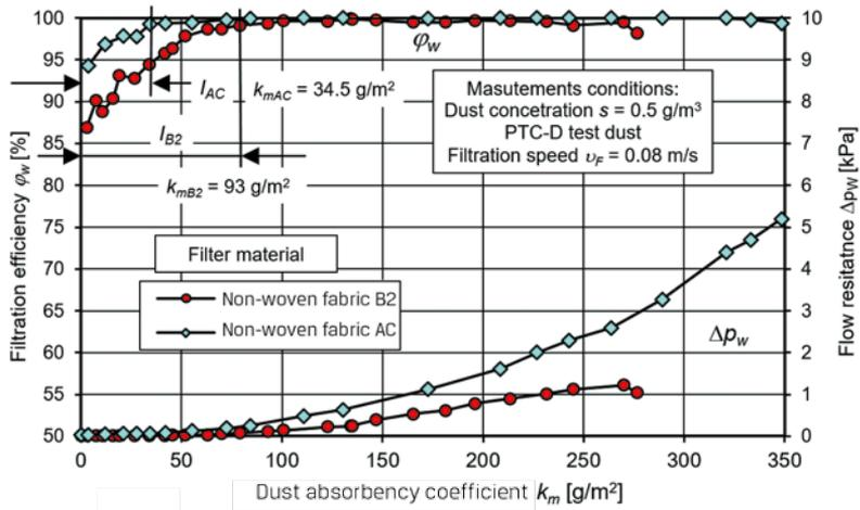
Fig. 21. Filtration efficiency  $\phi_w = f(k_m)$  and flow resistance  $\Delta p_w = f(k_m)$  characteristics in a function of the dust  $k_m$  absorbency coefficient of the B2 and AC filter non-woven fabrics specified under single-stage filtration conditions [6]
