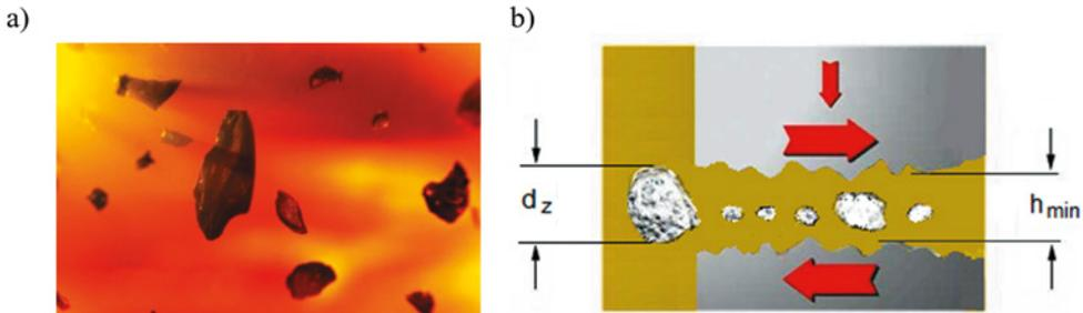
Fig. 7. Effect of solid particulates on a tribological connection: a) contaminations suspended in the oil [1], b) condition of the maximum connection consumption [11]
