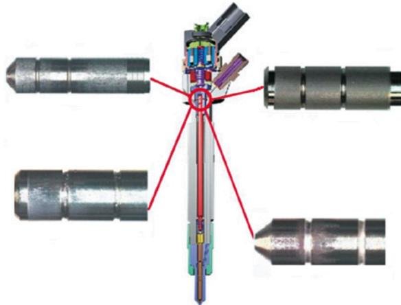
**Fig. 31. Example abrasive wear of injection components visible as control piston peripheral abrasions [23]**
