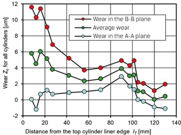
Fig. 13. Wear of a cylinder liner of a 4-cylinder, turbocharged engine with spontaneous ignition and power  $N_{emax} = 66$  kW in a plane perpendicular (B-B) and parallel (A-A) to the engine axis [21]
