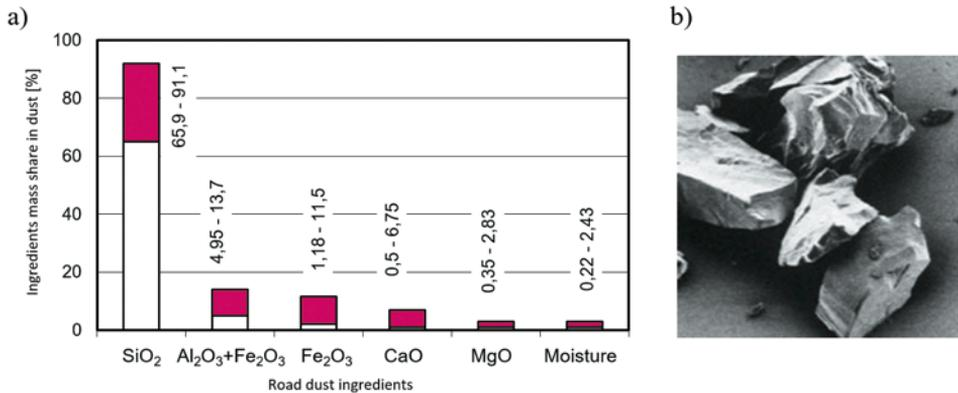
Fig. 1. Average chemical composition of road dust in Poland (a) [2], image of silica grains (b) [12]
