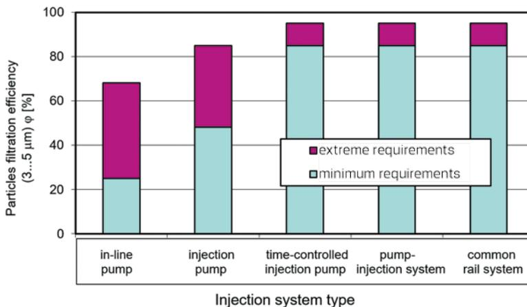
Fig. 6. Recommendations for minimum filtration efficiency of diesel oil filters [5]
