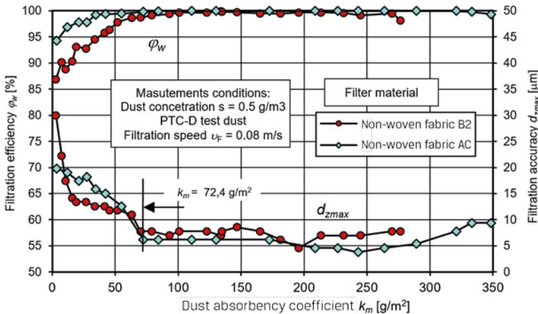
Fig. 22. Filtration efficiency  $\phi_w = f(k_m)$  and accuracy  $d_{zmax} = f(k_m)$  characteristics in a function of the dust  $k_m$  absorbency coefficient of the B2 and AC filter non-woven fabrics specified under single-stage filtration conditions [6]
