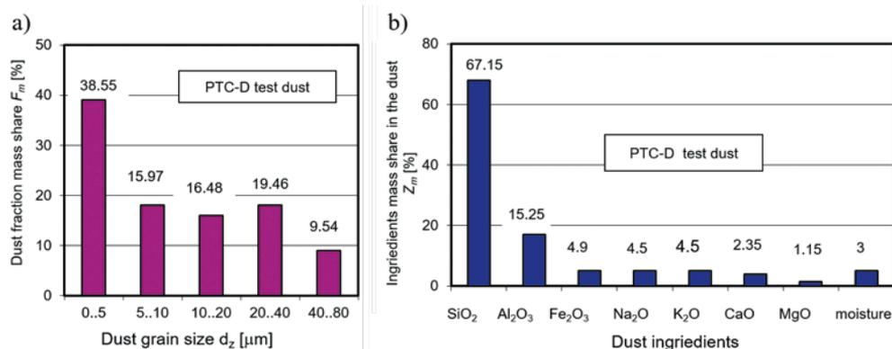
Fig. 18. Granulometric (a) and chemical composition (b) of the PTC-D test dust [27]
