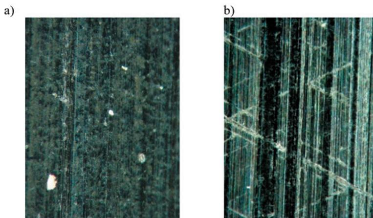
**Fig. 12. Topography of the truck engine's cylinder bearing surface operated with an inoperative air filtration system:**
