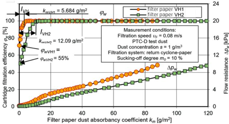
Fig. 19. Filtration performance  $\varphi_{in} = f(k_m)$  and flow resistance  $\Delta p_w = f(k_m)$  characteristics of the VH1 and VH2 filter paper in a function of the dust absorbancy coefficient  $k_m$  [7]
