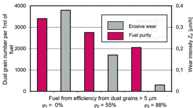
Fig. 29. Contaminants in the fuel effect on the injector erosive wear intensity [30]
