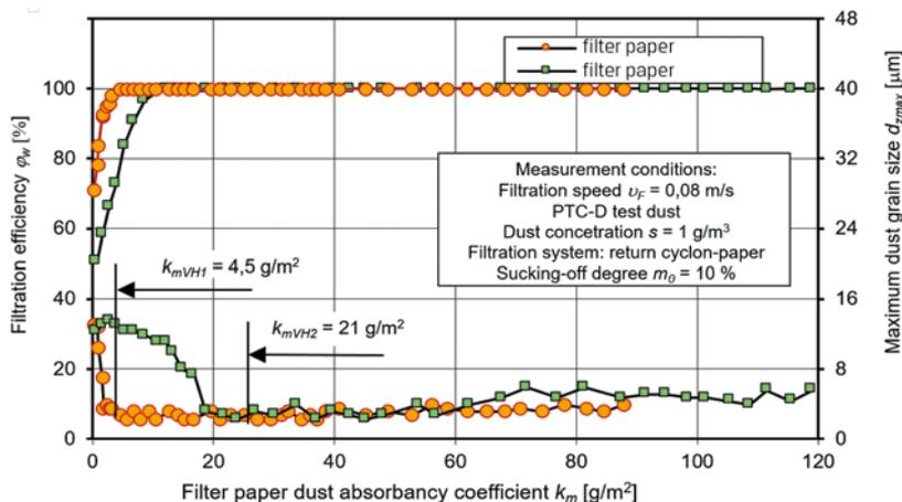
Fig. 20. Maximum dust grains size  $d_{zmax}$  in a function of the dust coefficient absorptivity  $k_m$  of the VH1 and VH2 filter paper operating behind the cyclone as the second filtration stage [7]
