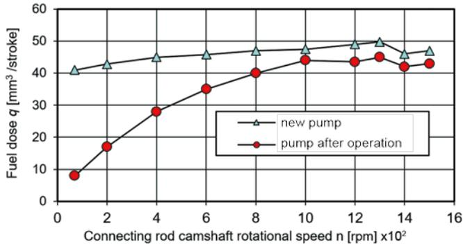
Fig. 28. Classic injection pump characteristics – the new one and after operation [7]
