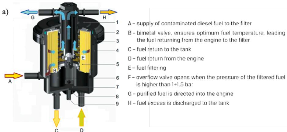
**Fig. 37. Fuel filter in the Common Rail system: 1 - plastic filter cover, 2 - o-ring, 3 - metal ring, 4 - plastic filter housing, 5 - filter medium (with folds in a star pattern), 6 - bimetal valve (thermostatic switch), 7 - water settlement tank, 8 - water drain plug, 9 - drainage tube [33]**
