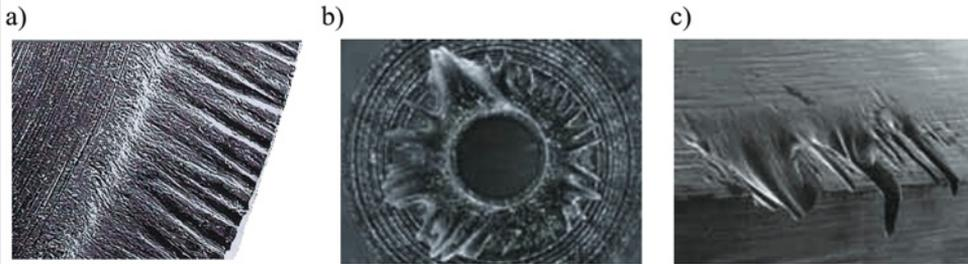
**Fig. 30. Wear of injection system components at insufficient fuel filtration:**
