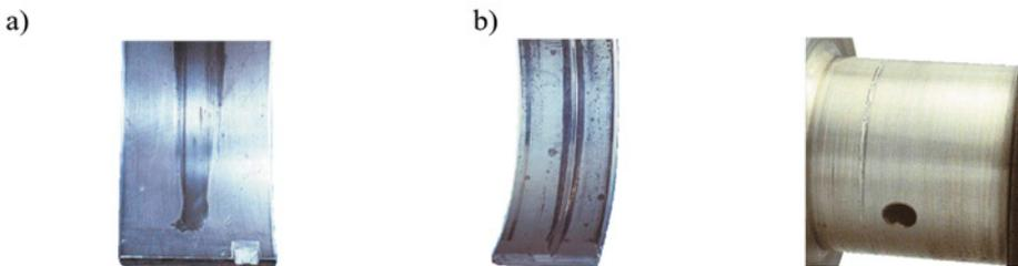
Fig. 24. View of engine shells (a) and crankshaft pivot (b) of the car operated with an inoperative air filtration system [26]
