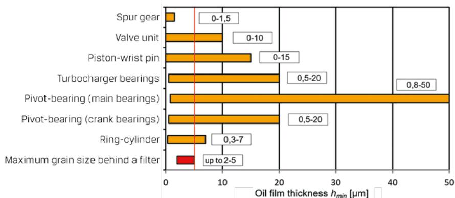
Fig. 9. Oil film thicknesses in typical combustion engine connections [4]
